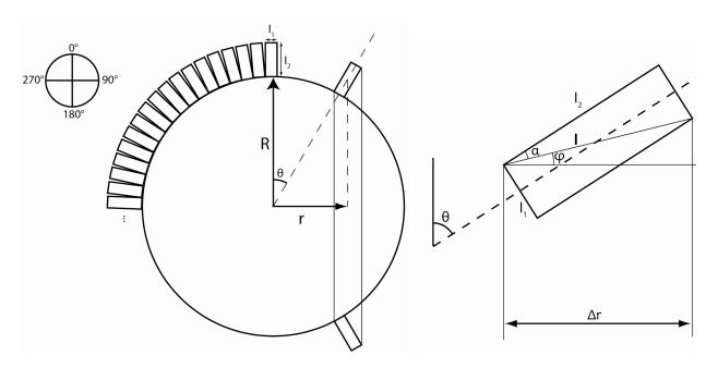
a) The width of the line of response (LOR)  $\Delta r$  is the projection of the diagonal of the crystal:
