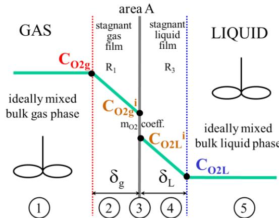
$$\text{rate} = A \underbrace{k_g}_{\text{red}} \left( C_{O_2g} - C_{O_2g}^i \right) = A \underbrace{k_l}_{\text{blue}} \left( C_{O_2L}^i - C_{O_2L} \right) = K_L A \left( C_{O_2L}^* - C_{O_2L} \right) \text{ with } C_{O_2L}^* = m \cdot C_{O_2g}$$
