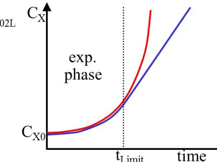
O<sub>2</sub> transfer limitation in **Chemostat** reactor.
