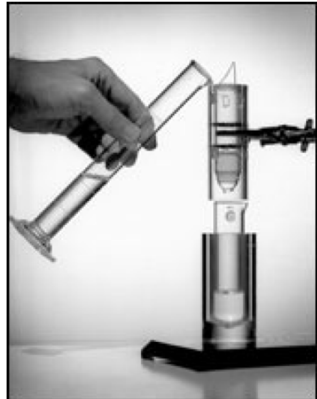
Demonstration of eluting the ^{99\text{m}}\text{Tc} of ^{99}\text{Mo} (shielding is removed, Brookhaven NL, 1957)
