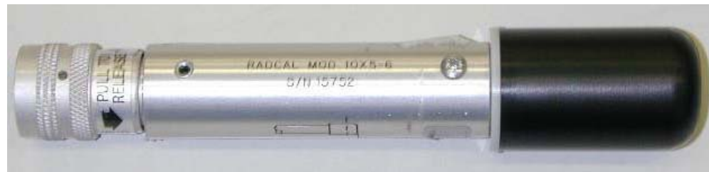
Figure 2.5: Example of an ionization chamber used in radiodiagnosics (Radcal chamber with a volume equal to 6 cm 3 ).
