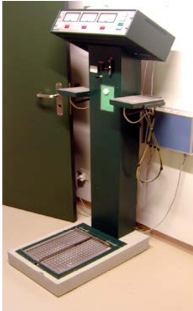
Example proportional counter used to monitor foot and hand contamination (Berthold LB 1041 counter).
