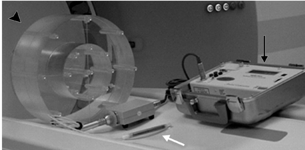
Equipment typically used to measure  $CTDI_{100}$  includes an integrating electrometer (black arrow), a 100-mm-long CTDI ionization chamber (white arrow), and a CTDI phantom made of polymethylmethacrylate (arrowhead).
