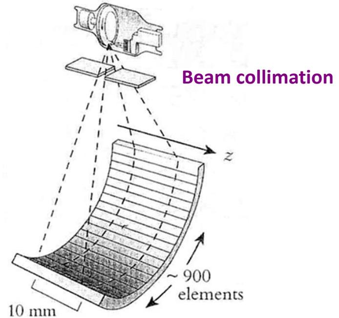
$$\text{Pitch} = \frac{\text{Table advance per tube rotation}}{\text{X-ray beam nominal collimation}}$$
