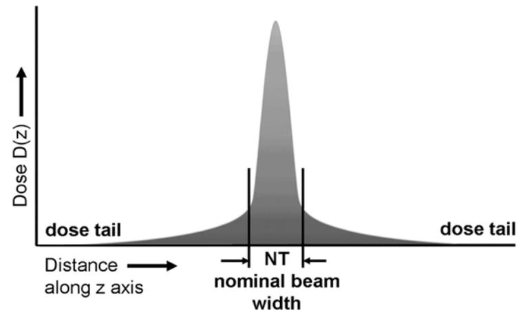
The radiation dose profile along a line perpendicular to the plane of a single axial CT scan shows a peak where the primary beam slices through the CTDI phantom. The tails of the dose profile are caused by scattered radiation. The integral of the area under the curve is normalized to the nominal beam width  $NT$  to determine the CTDI. A  $\text{CTDI}_{100}$  value is obtained if integration limits of  $\pm 50$  mm are used
