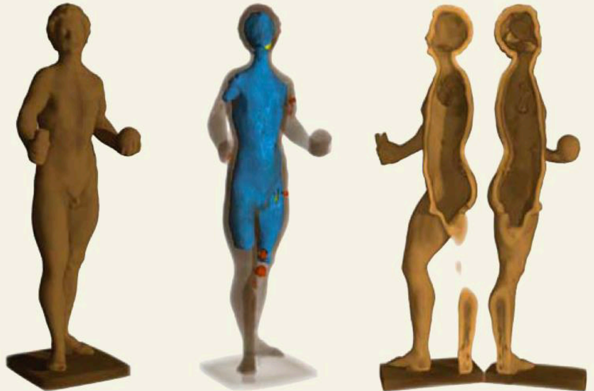
Figure 24: Tomographic views of a bronze sculpture: virtual slices can be created without damaging this unique object.
