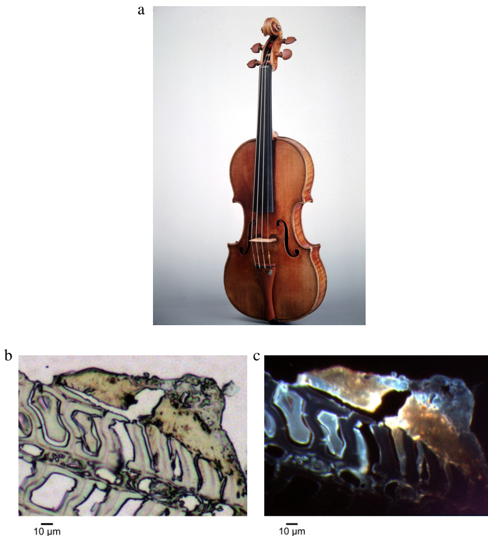
Fig. 28. SR-UV/VIS study of the finishing of the Provigny violin from A. Stradivari at the DISCO beamline, SOLEIL synchrotron (France). (a) Photograph of the Provigny violin (Antonio Stradivari, 1716, Cremona, coll. Musée de la musique, Paris, inv. num. E.1730). Credits: Cité de la musique/J.-C. Billing. (b) Transmitted light microscopy image of a cross-section of a varnish from the Provigny violin by A. Stradivari, exhibiting several strata of organic binding media materials on top of spruce wood. (c) Reconstructed RGB full-field luminescence microscopy image of the cross-section; 340 nm excitation. Images collected band-pass emission filters centred at 500, 600, and 700 nm (all with 40 nm FWHM) (respectively 150, 45, and 120 s integration times) have been corrected from dark field and respectively attributed to the blue, green, and red channels [148]. (For interpretation of the references to colour in this figure legend, the reader is referred to the web version of this article.)
