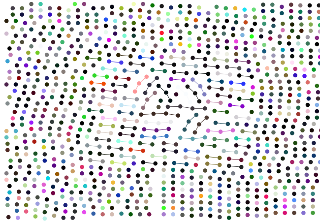
Figure 3.4: An instance of G(1000, 0.2/1000) . The graph consists only of small trees.
