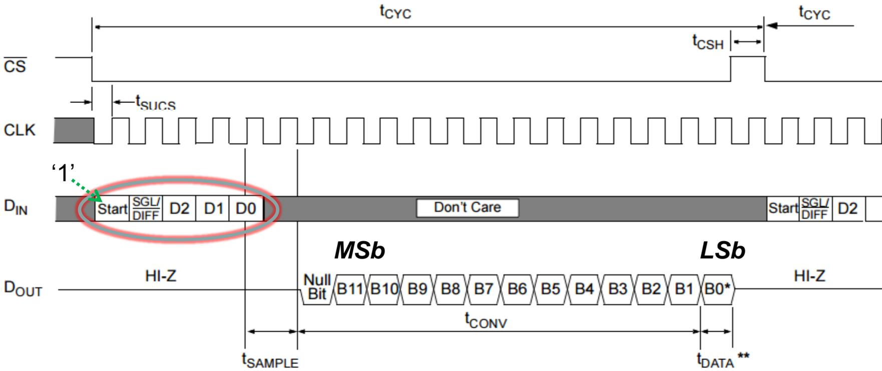
\* After completing the data transfer, if further clocks are applied with  $\overline{CS}$  low, the A/D converter will output LSB first data, followed by zeros indefinitely (see Figure 5-2 below).
