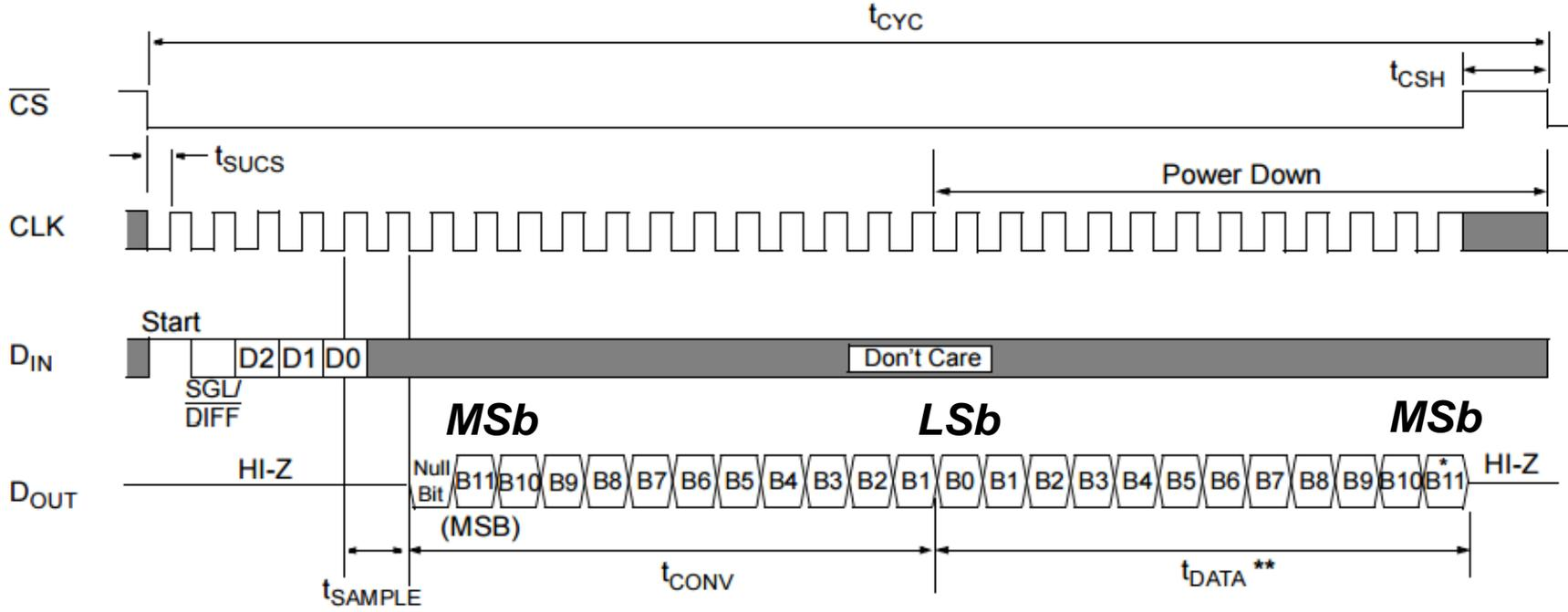
\* After completing the data transfer, if further clocks are applied with  $\overline{CS}$  low, the A/D converter will output zeros indefinitely.
