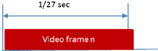
Clock Too Slow - Failure to Read an Entire Frame Within the Frame Period
