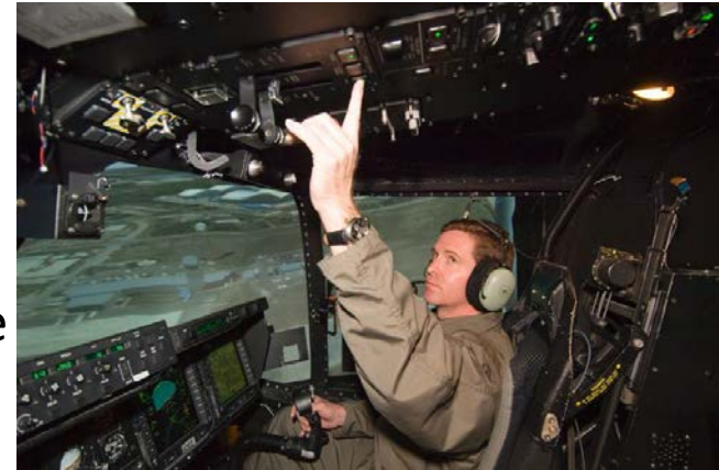
[modern flight simulator with a tangible cockpit serving as a rest frame]
