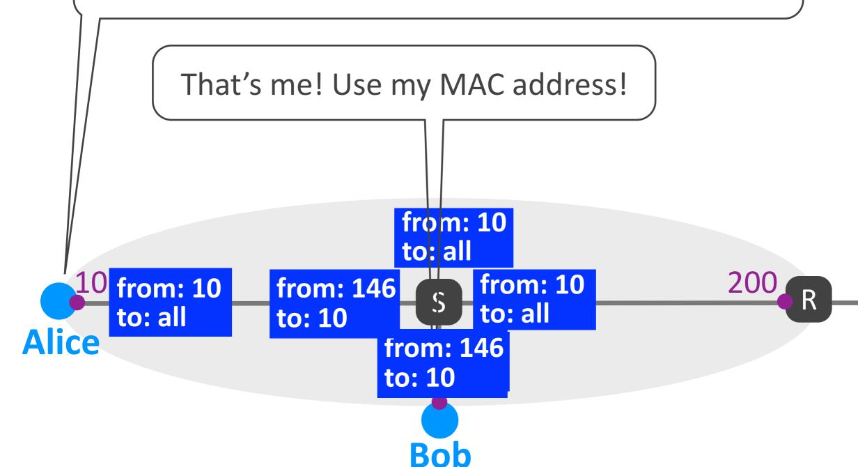
I want to send a packet to IP address 129.12.80.43 Which destination MAC address should I use? Use my MAC address! from: 10 to: all from: 10 from: 200 200 from: 10 to: 10 to: all to: all **Alice**
