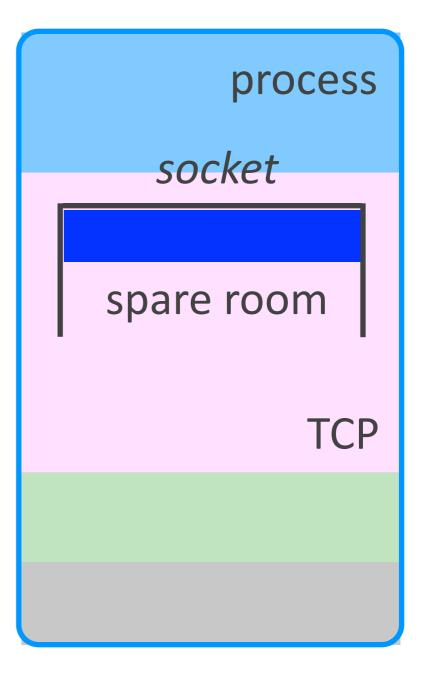
receiver window=100 bytes SEQ=1, data=bytes #1 to #100 ACK=101, receiver window=80 bytes
