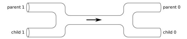
To ensure the pipe works properly, the ends of the pipe that are not used should be closed. For instance, if the child receives data from the parent, the parent should close pipefds[0] and the child should close pipefds[1].
