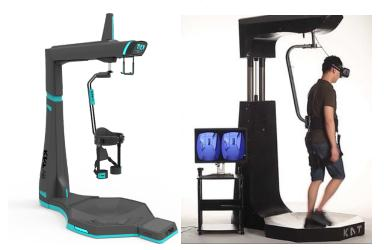
**Goal**: Experiment treadmill in VR with head mounted display and a consumer tracking system. Locomotion is a real challenge in VR. Indeed, you might have to travel a whole world in your living room. If the user uses the Joystick to move it might have cyber sickness. You can teleport yourself but you will be less immersed.
