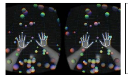
**Goal**: Experiment VR hand tracking and head mounted display with budget equipment. Controlling all the degrees of freedom of a virtual hand is far from trivial, leap motion accomplishes that that with stereo geometry (infrared projection + infrared cameras).
