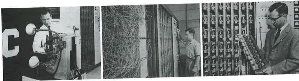
Figure 4.8 Illustration of the Mark 1 perceptron hardware. The photograph on the left shows how the inputs were obtained using a simple camera system in which an input scene, in this case a printed character, was illuminated by powerful lights, and an image focussed onto a 20 \times 20 array of cadmium sulphide photocells, giving a primitive 400 pixel image. The perceptron also had a patch board, shown in the middle photograph, which allowed different configurations of input features to be tried. Often these were wired up at random to demonstrate the ability of the perceptron to learn without the need for precise wiring, in contrast to a modern digital computer. The photograph on the right shows one of the racks of adaptive weights. Each weight was implemented using a rotary variable resistor, also called a potentiometer, driven by an electric motor thereby allowing the value of the weight to be adjusted automatically by the learning algorithm.
