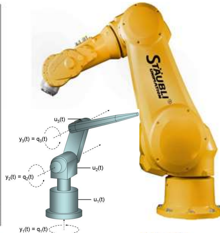
Figure 1, Serial robots. (Left) representation of the principle. (Right) Robot Staubli TX200
