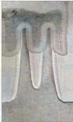
14 nm 2 nd Generation Tri-gate Transistor
