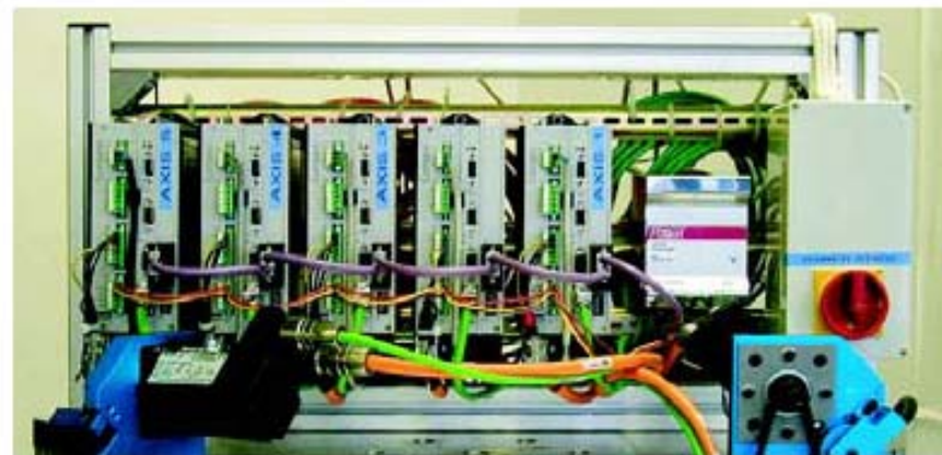
Figure 5: The Control Hardware. The figure shows the 5 drives of our prototype. They contain the PROFIBUS-interface, the control-"intelligence" and the amplifiers.
