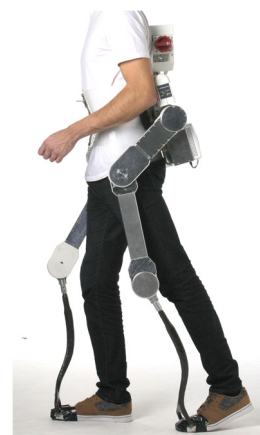
Figure 1. AUTONOMYO exoskeleton worn by a healthy subject, the current prototype is missing leg attachments (see Fig.2)
