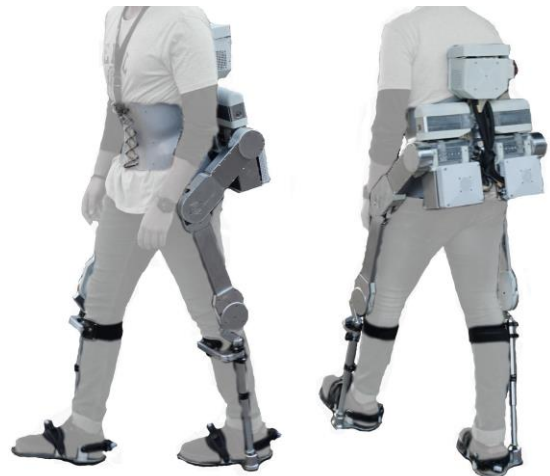
Figure 1. The AUTONOMYO lower limb exoskeleton with its six actuated degrees of freedom at the hip and knee flexion/extension and at the hip adduction/abduction. On left, a front-side view at 45°. On right, a back-side view at 45°.
