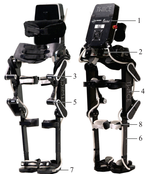
Fig. 1: TWICE, front and rear view. From top to bottom: electronics enclosure (1), back structure (2), hip actuation (3), thigh segment (4), knee actuation (5), shank segment (6) and foot plate (7). Cuffs with hook-and-loop straps (8) are used to create the mechanical interface with the user, in-between the legs.
