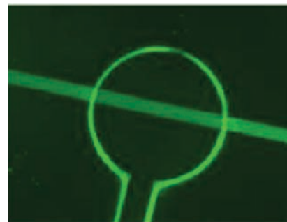
Quake Valve Off
