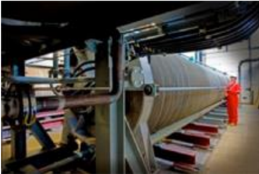
NEL-Hydrogen: 50-485 Nm 3 H 2 /h 25% KOH aqueous solution, 80°C
