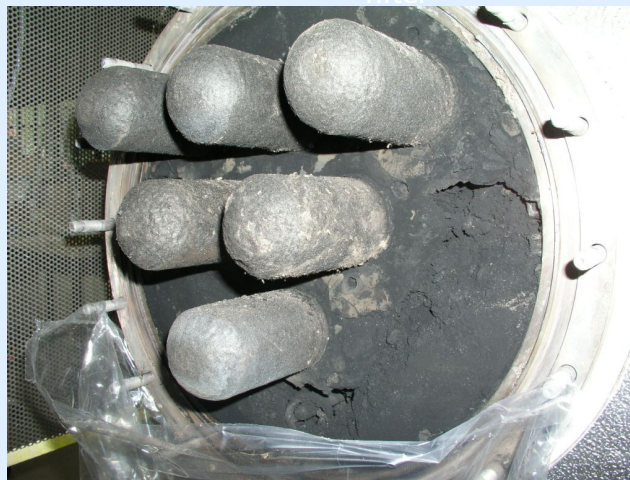
Raw gas chamber completely filled with ash (2 kg)
