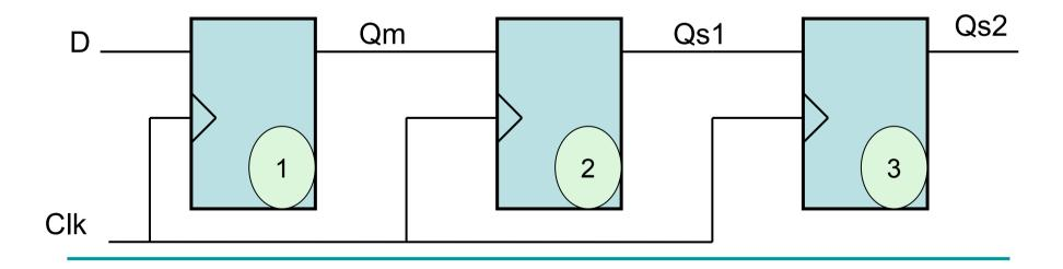
→ The Qsn signal can be used by all the logic that need it: the level will be the same for all the logic elements
