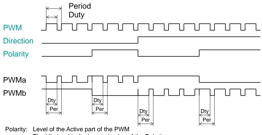
The Idle level is the inverted value of the Polarity
