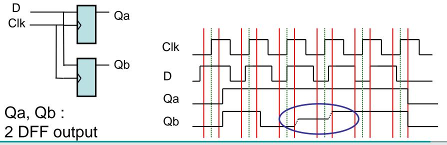
$\rightarrow$  At the same clk sampling time (i.e. rising\_edge), all the logics using the signal and clocking it need to see it at the same level !!
