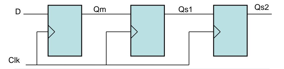
→ The Qsn signal can be used by all the logic that need it: the level will be the same for all the logic
