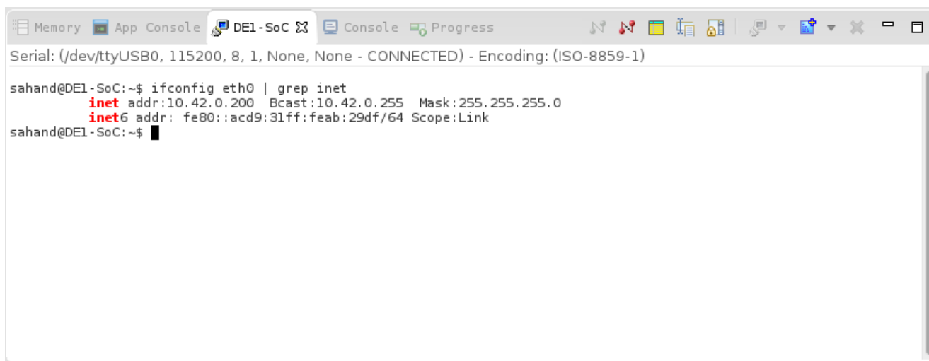
Figure 13-16. Obtaining the DE1-SoC's IP Address through ARM DS-5's Serial Terminal
