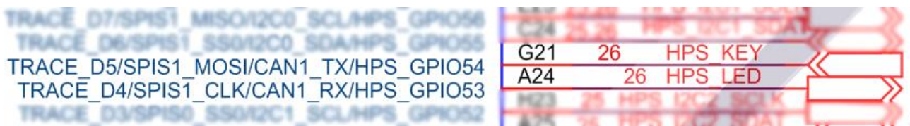
Figure 9-5. HPS_KEY_N & HPS_LED on DE1-SoC Schematic. Note that the schematic uses “HPS_KEY” instead of “HPS_KEY_N” as the name of the signal. This is a mistake, as the button is active-low, so the “_N” in the name is warranted for clarity.
