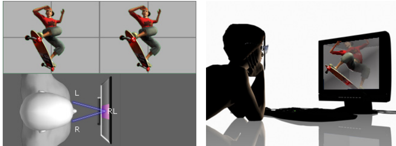
The L and R image lead your convergence point to fall on the display.
