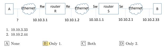
**Question 6** At point 3, a packet sniffer observes one IP packet sent by B to A . What is the IP destination address contained in the IP packet header ?
