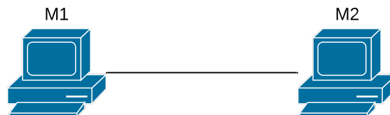
Figure 5: Point-to-point wired connection of two physical machines
