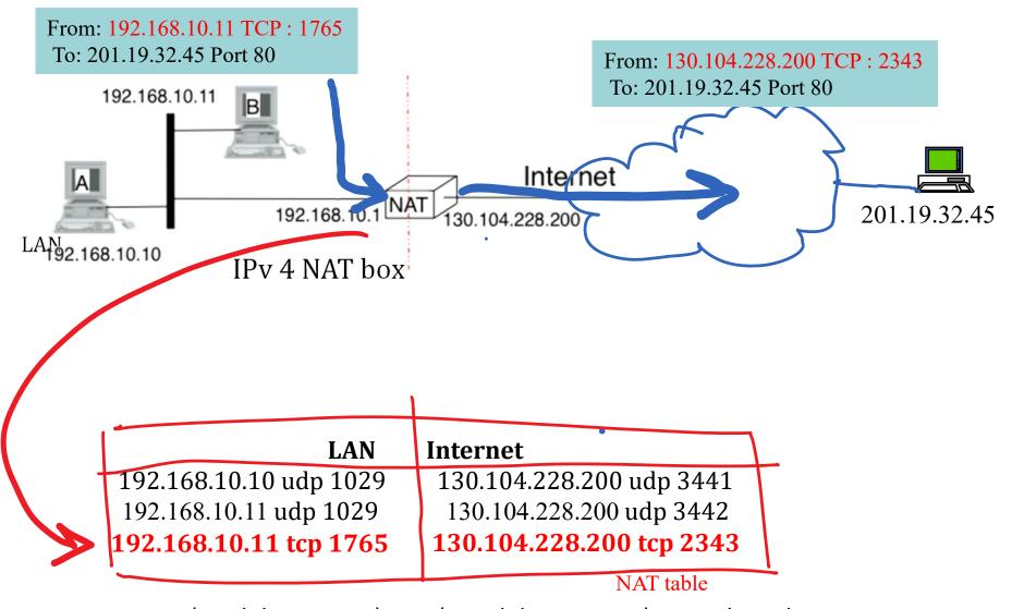
Mapping (iAddr, iPort) to (eAddr, ePort) can be done automatically, as shown; but also statically (e.g. to support a web server in LAN)
