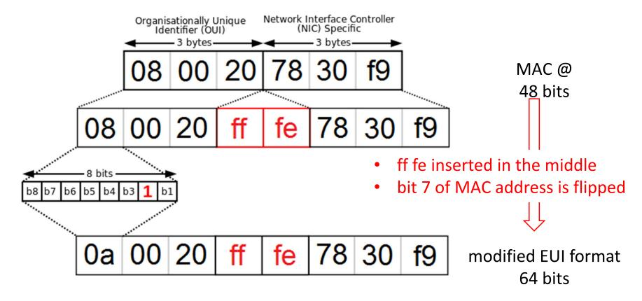
Q: Why is bit 7 flipped ? A: Bit 7 is the "g" bit -- an EUI is defined by IEEE; a locally assigned EUI (i.e not derived from MAC address) has g bit equal to 1; this is inconvenient for IPv6 addresses. IPv6 uses the reverse convention: bit 7 of modified EUI is 1 for EUI derived from globally assigned MAC addresses, and 0 for manually assigned addresses (e.g. 2001:620:618:100::1).
