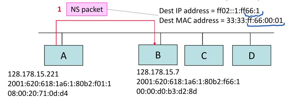
A has a packet to send to B = 2001:620:618:1a6:1:80b2:f66:1
