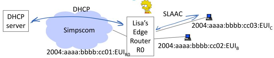
Why? A home (or enterprise) IPv6 router R0 is configured by ISP using DHCP. Local devices are autoconfigured from home router using e.g. SLAAC. Home router needs an IPv6 prefix for the entire home network.
