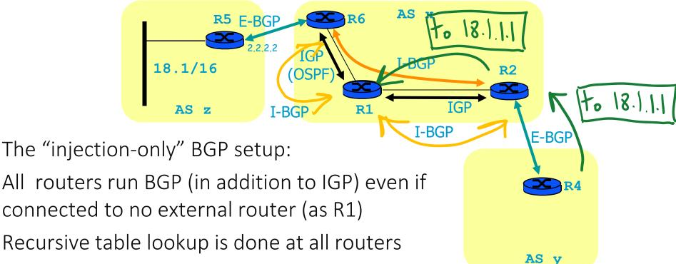
All routers run BGP (in addition to IGP) even if connected to no external router (as R1)
