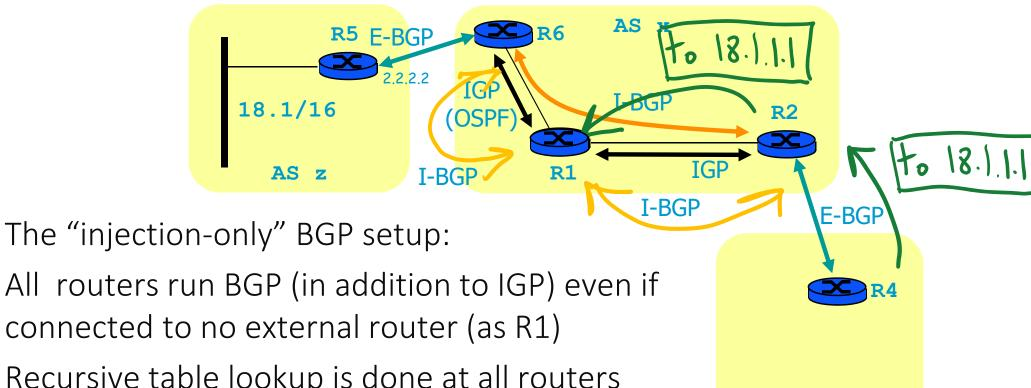
All routers run BGP (in addition to IGP) even if connected to no external router (as R1)
