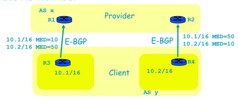
Client uses BGP with MED to control flows of traffic (e.g provider should use R1-R3 for all traffic to 10.1/16
