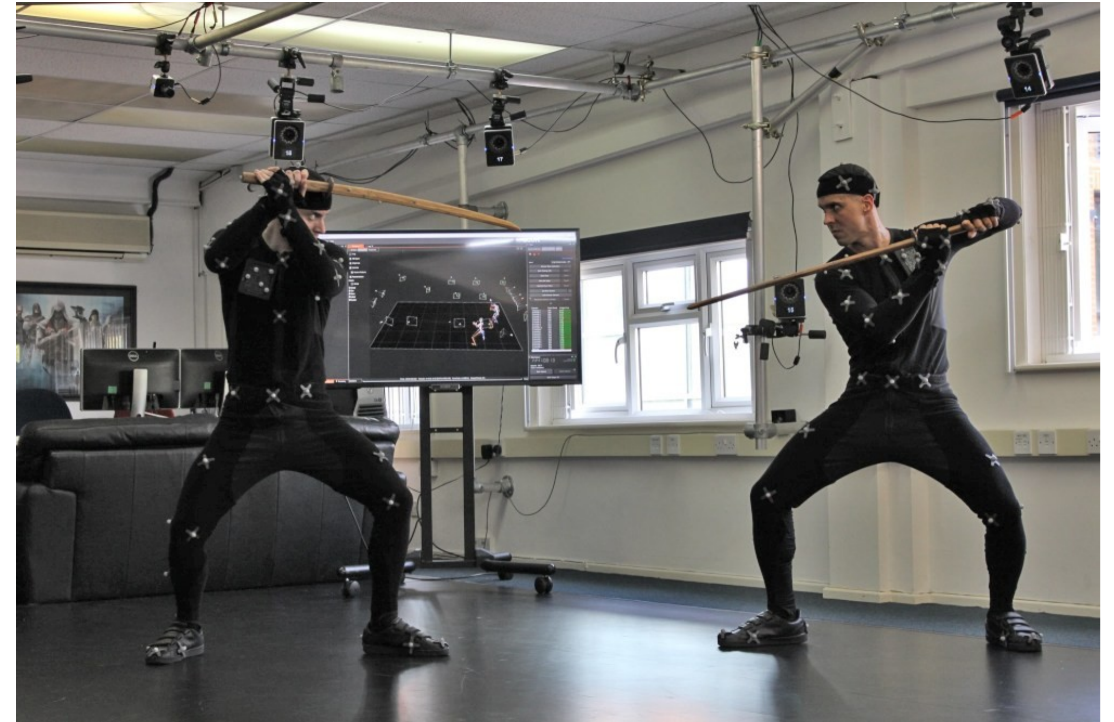
Performer equipped with passive suits for motion capture using Vicon Shogun
