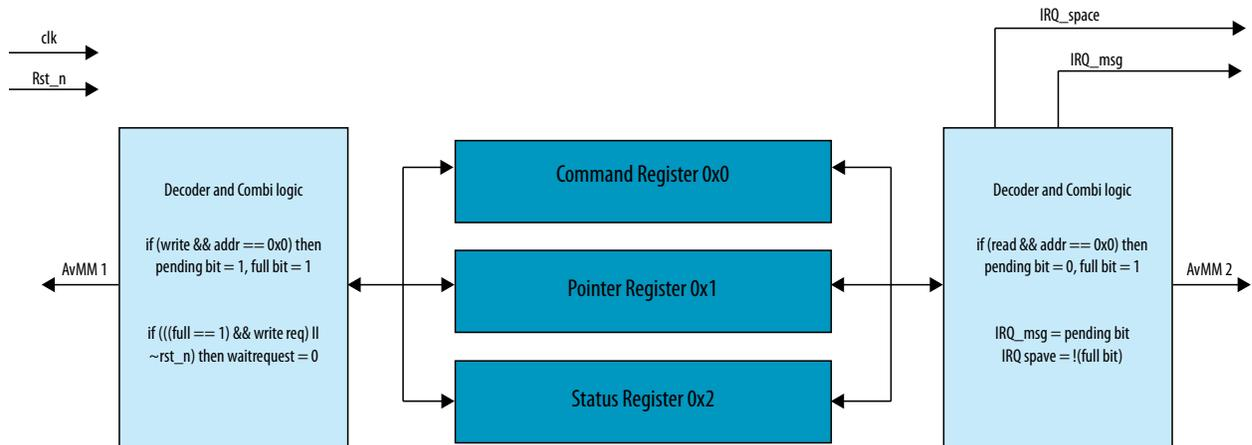
The Mailbox is clocked with single source. Both of the Avalon-MM Slave interfaces have its individual function to set and clear the Full bit and Message Pending bit. The Avalon-MM Slave of the sender processor will only set the status bits, while the Avalon-MM Slave of the receiver processor only clears the status bit.
