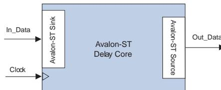
The Avalon-ST Delay core adds a delay between the input and output interfaces. The core accepts all transactions presented on the input interface and reproduces them on the output interface N cycles later without changing the transaction.
