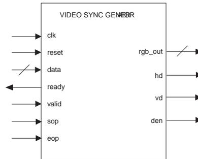
You can configure various aspects of the core and its Avalon-ST interface to suit your requirements. You can specify the data width, number of beats required to transfer each pixel and synchronization signals. See the **Parameters** section for more information on the available options.
