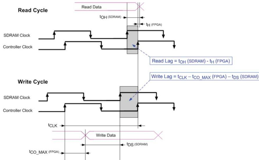
Figure 2-6: Calculating the Maximum SDRAM Clock Lead
