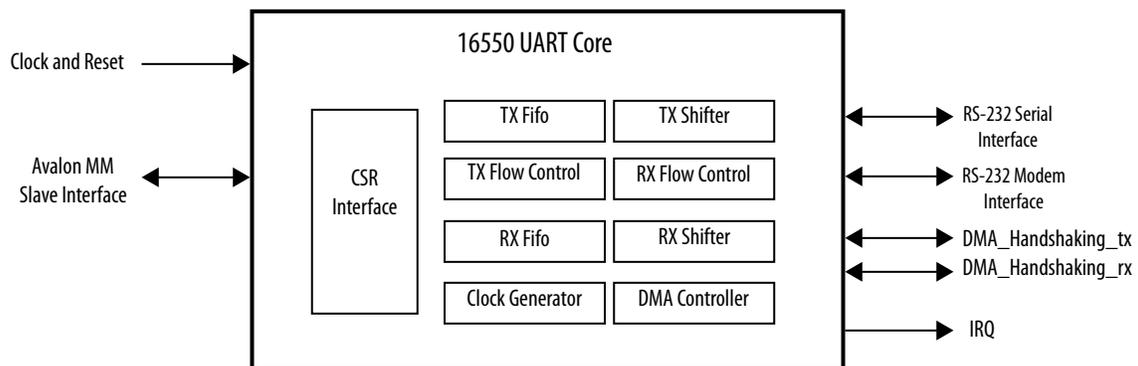
The figure above shows the high level architecture of the UART IP. Both Transmit and Receive logic have their own dedicated control & data path. An interrupt block and clock generator block is also present to service both transmit and receive logic.
