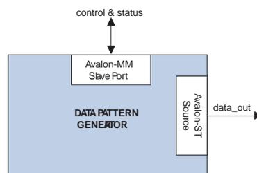
You can configure the width of the output data signal to either 32-bit or 40-bit when instantiating the core.
