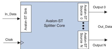
The Avalon-ST Splitter core copies all input signals from the input interface to the corresponding output signals of each output interface without altering the size or functionality. This includes all signals except for the `ready` signal.
