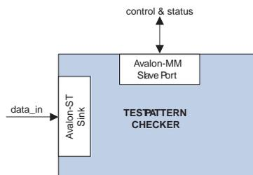
The test pattern checker core detects exceptions and reports them to the control interface via a 32-element deep internal FIFO. Possible exceptions are data error, missing start-of-packet (SOP), missing end-of-packet (EOP) and signalled error.
