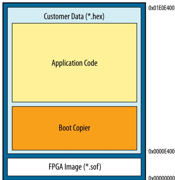
At the start of the memory map is the FPGA image, followed by the boot copier, the application and then customer data. The size of the FPGA image is unknown and the exact size can only be known after the Quartus compile. However, the Nios II Reset Vector must be set in Qsys and must point to right after the FPGA image (i.e. the start of the boot copier).
