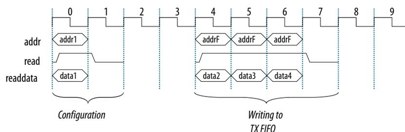
Writes to the UART are expected as singles during setup phase of any transaction and as back-to-back writes to the same address when the Tx FIFO needs to be filled.
