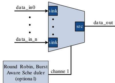
The internal scheduler considers one input interface at a time, selecting it for transfer. Once an input interface has been selected, data from that input interface is sent until one of the following scenarios occurs:
