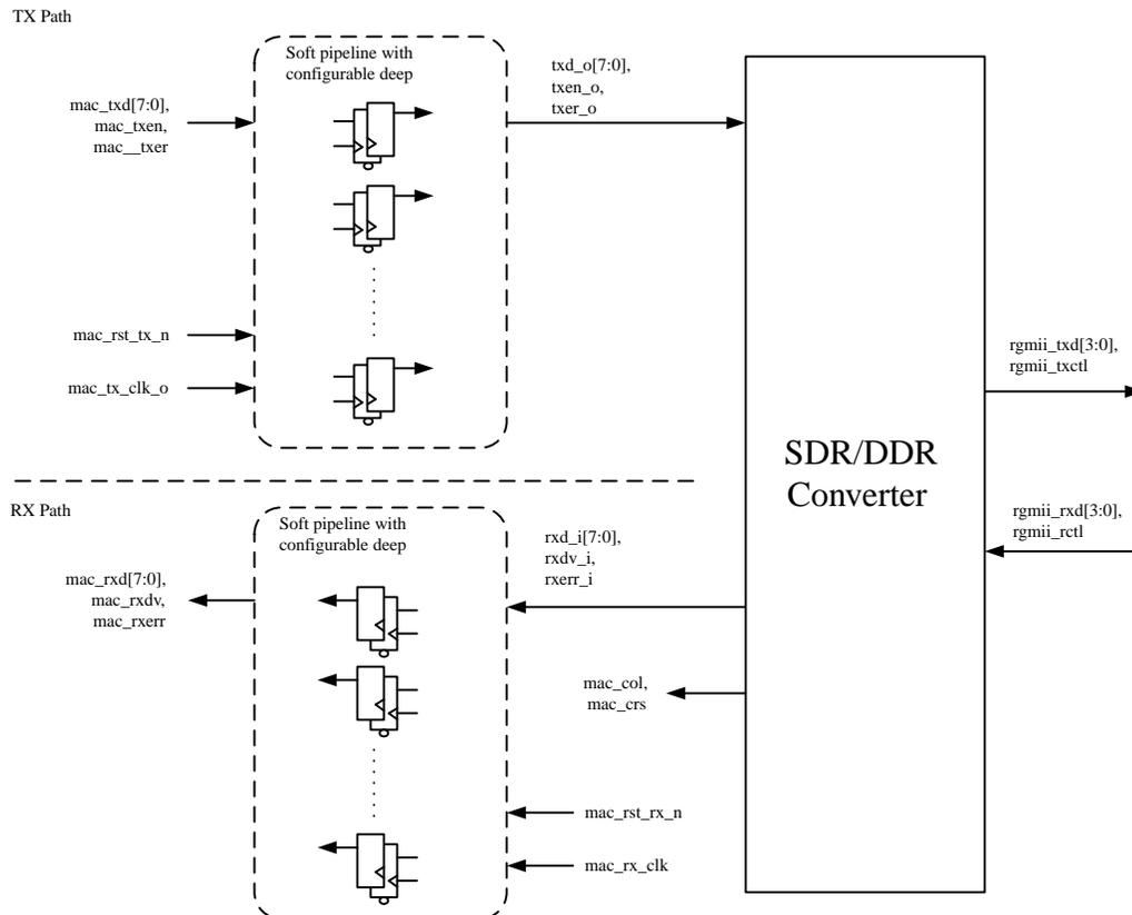
For transmit path, the GMII/MII data goes through the transmit pipeline register stage before going into the SDR/DDR converter block. The pipeline logic can be optionally enabled or disabled by the user during generation time.
