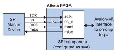
In the **SPI Core Block Diagram**, the SPI core provides a master interface driving multiple off-chip slave devices. Each slave device in the **SPI Core Configured as a Slave** figure must tristate its `miso` output whenever its select signal is not asserted.
