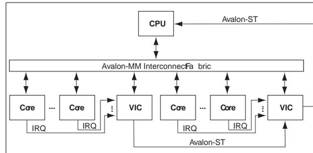
To use the VIC, the processor in your system needs to have a matching Avalon-ST interface to accept the interrupt information, such as the Nios<sup>®</sup> II processor's external interrupt controller interface.
