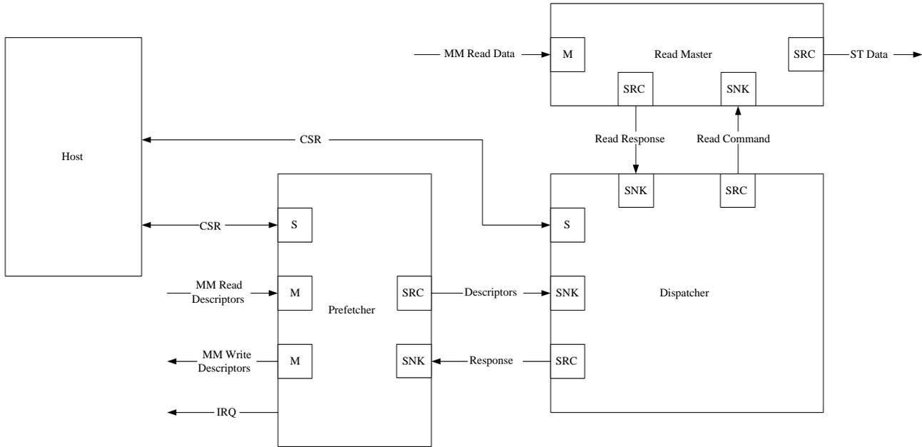
Figure 25-7: Streaming to Memory-Mapped Configuration with Prefetcher Enabled
