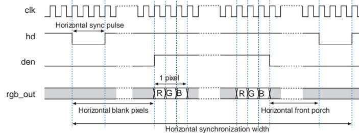
The table below shows the horizontal synchronization timing when the parameters **Data Stream Bit Width** and **Beats Per Pixel** are set to 24 and 1, respectively.
