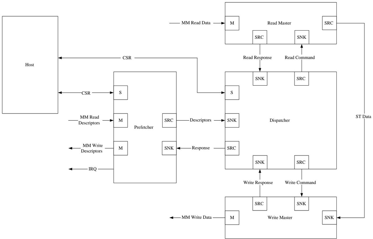
Figure 25-6: Memory-Mapped to Streaming Configuration with Prefetcher Enabled
