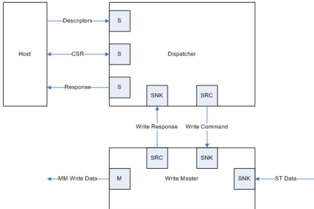
The Altera mSGDMA support 32-bit addressing by default. However, it can support 64-bit addressing when you select **enhanced feature** in the dispatcher module GUI. It also supports extended features such as dynamic burst count programming, stride addressing, extended descriptor format (64-bit addressing), and unique sequence number identification for executed descriptor.
