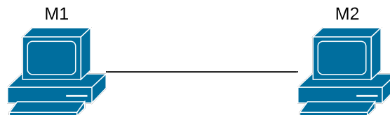
Figure 5: Point-to-point wired connection of two physical machines
