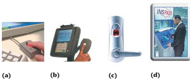
Figure 4. Biometrics application examples. (a) Digital Persona's fingerprint verification system provides personal recognition for computer and network login. (b) Indivios manufactures a fingerprint-based point-of-sale (POS) terminal that verifies customers before charging their credit cards. (c) BioThentica's fingerprint-based door lock restricts access to premises. (d) The Inspass immigration system, developed by Recognition Systems and installed at major airports in the US, uses hand geometry verification technology.
