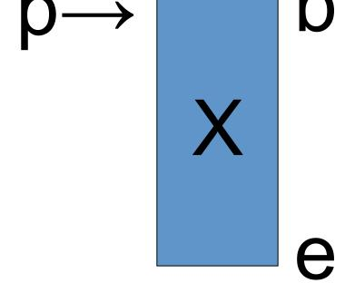
An execution is memory-safe <=> object X is only accessed through pointers that are based on X
