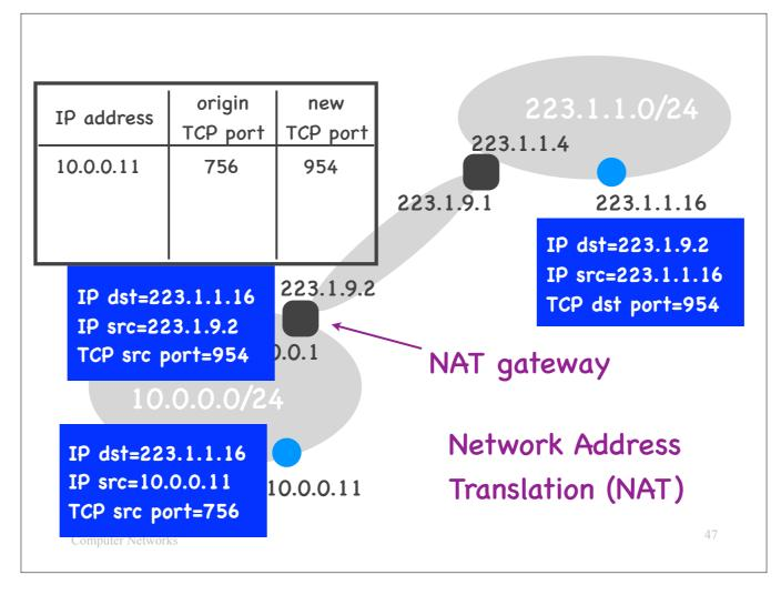
When the border router receives a packet coming from the private subnet, it first creates a piece of state, mapping IP address 10.0.0.11 and port number 756 to a new port number 954. Then it rewrites, not only the source IP address to 223.1.9.2; but also the source port number to 954.
