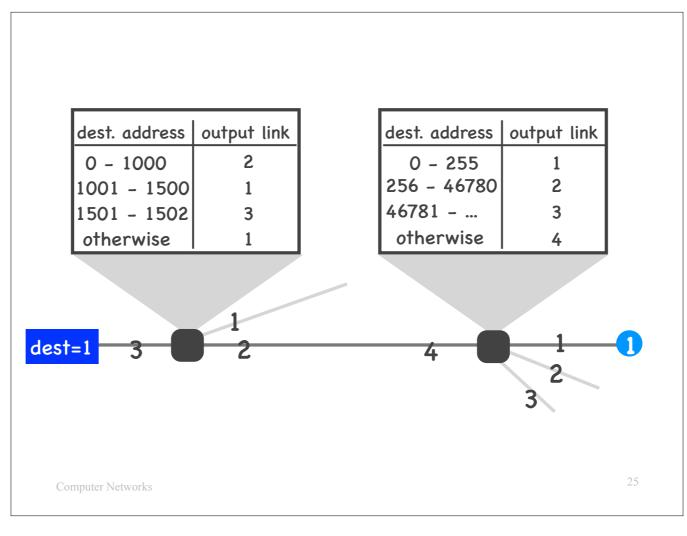
Each router actually maintains, in its forwarding table, a mapping from \*\*ranges\*\* of destination IP addresses (not individual IP addresses) to output links.
