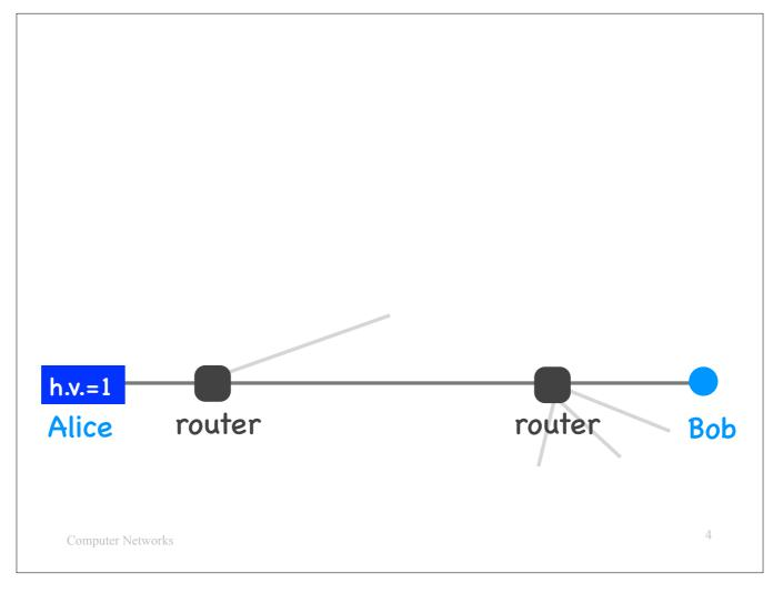
Forwarding is a process that takes place inside a router (also called network-layer switch) and determines what to do with a piece of data received by that device, e.g., where to send it next.
