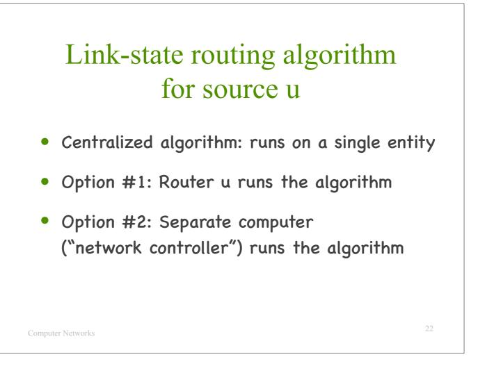
A link-state routing algorithm is a centralized algorithm, in the sense that, given the input (network graph and link costs), the algorithm is run on a single entity.
