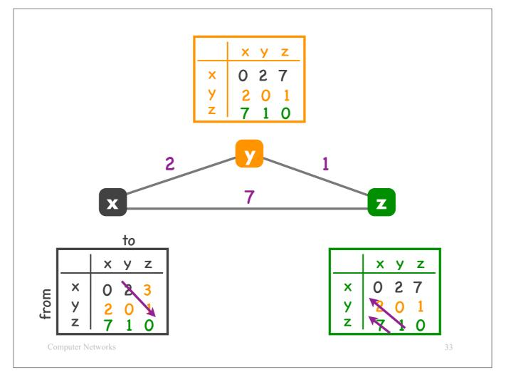
Hence, router x updates its structure with the fact that it can reach router z with cost 3. I have made the number 3 orange to indicate that router x can reach router z with this cost through router y (the orange router).
