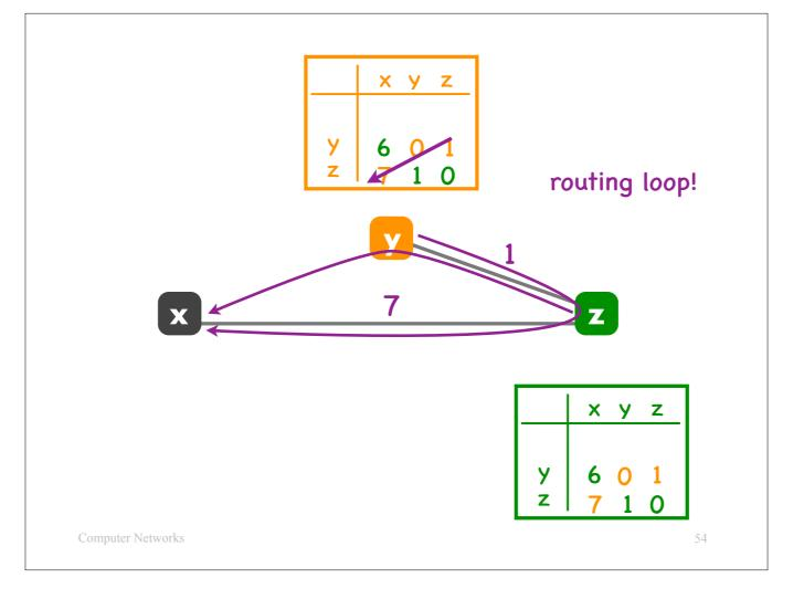
Router y says: – my path to router x is through router z; – router z's cost to router x has increased to 7;
