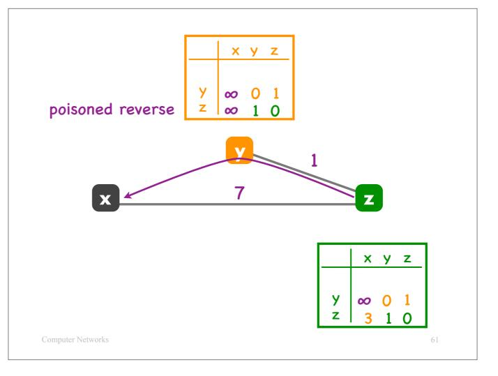
Then the neighbors exchange tables, router z learns that router y has been disconnected from router x...
