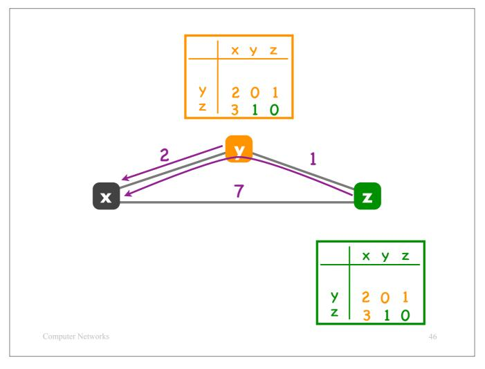
One of the main challenges in designing routing protocols is avoiding routing loops.
