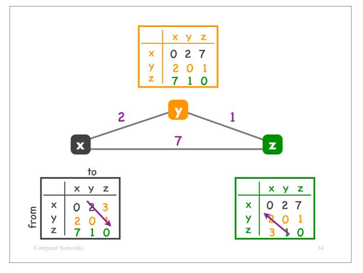
Hence, router z updates its structure with the fact that it can reach router x with cost 3.
