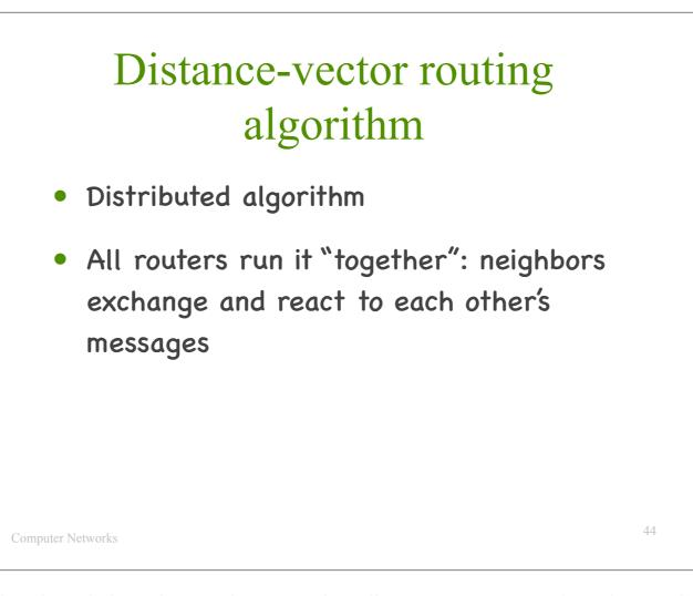
A distance-vector routing algorithm is a distributed algorithm, in the sense that all routers run it together: they exchange messages and they keep reacting to each other's messages.
