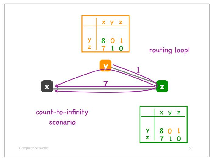
At this point, router z changes its path to router x: it routes to x through the direct link of cost 7 (note that the number 7 in z's table has now become green, it indicate that it corresponds to a direct link).
