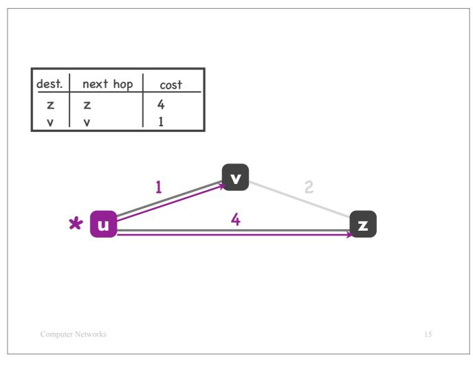
In the first step, the algorithm considers only the links that are directly connected to router u. It forgets about the rest of the network (it's as if the other links do not exist).
