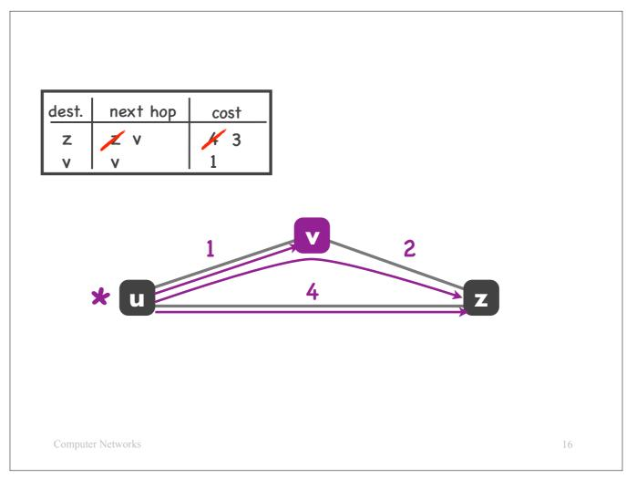
In the second step, the algorithm chooses a neighbor of router u — in our example, router v, and considers the links that are directly connected to that neighbor as well.
