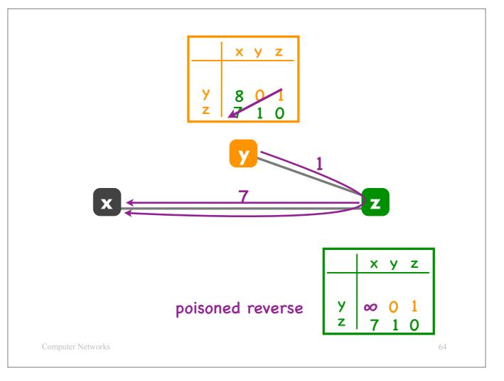
hence realizes that it (router y) can route to router x through router z with cost 1+7=8 and updates its table accordingly.
