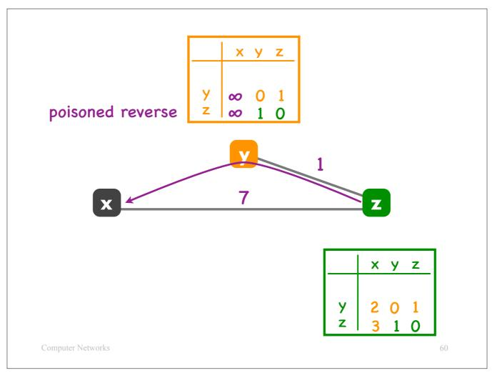
Hence, router y sets the cost of the path from itself to router x to infinity. Note that this infinity is NOT a poisoned reverse. It just indicates that the link from y to x is down, and y cannot route to x.
