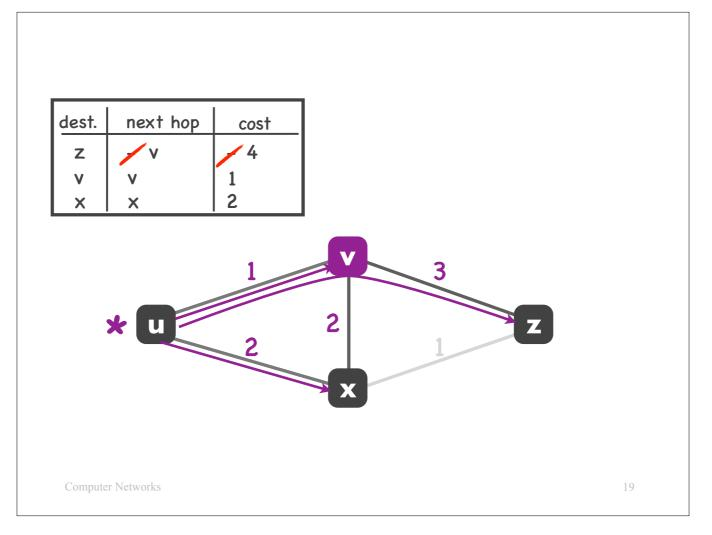
In the second step, the algorithm considers router v, and the links that are directly connected to router v.
