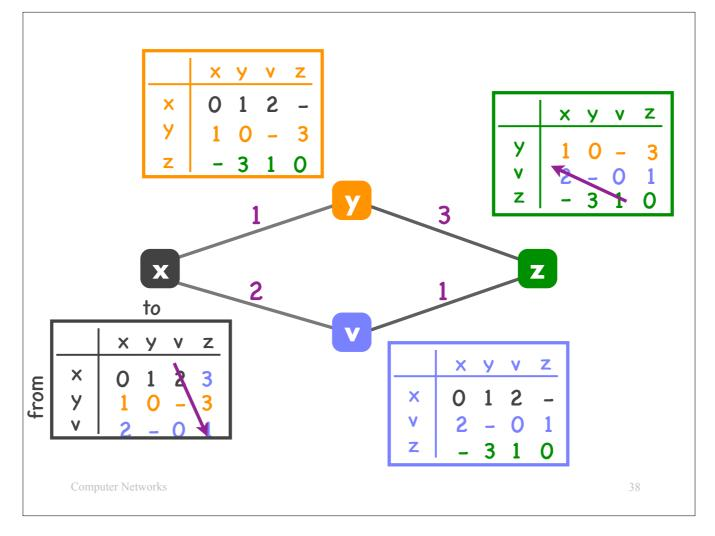
and updates its table accordingly (note that the new number 3 that appears in x's table is purple, because it was computed based on information propagated through router v).
