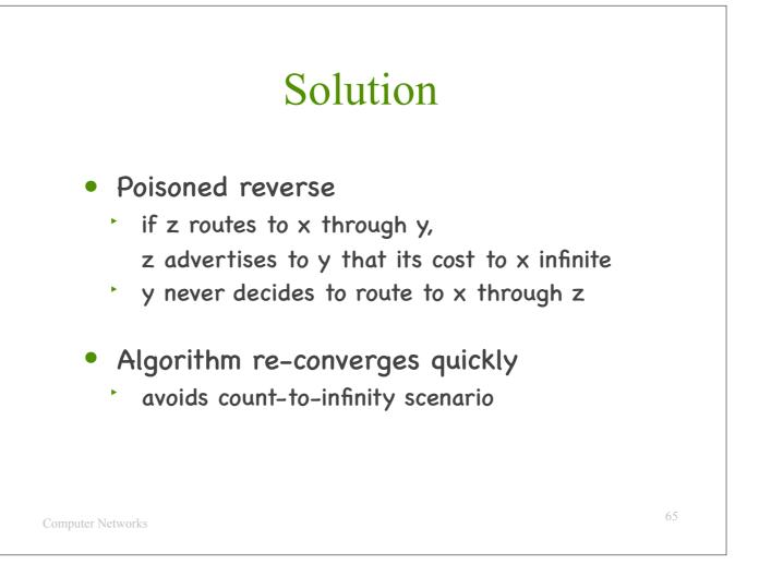
So: One way to avoid the count-to-infinity scenario is poisoned reverse, which enables the Bellman-Ford algorithm to re-converge quickly after a link failure.
