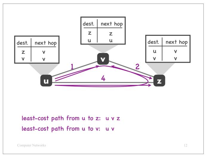
From router u to router z, there are two paths: a direct one, of cost 4, and an indirect one, through router v, of cost 1+2=3. The least-cost path is the indirect one.
