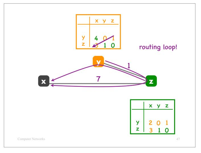
Router y immediately detects the problem, because it is directly connected to router x; so, it realizes that it does not have a link to router x any more.
