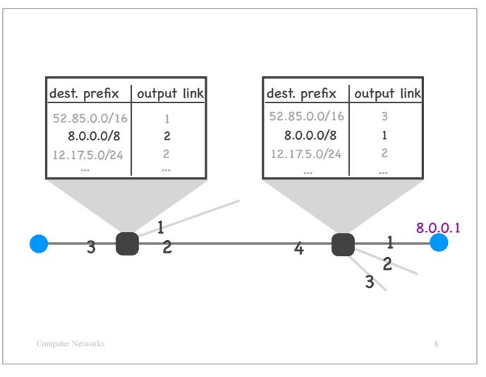
Consider a source and a destination end-system, the latter with IP address 8.0.0.1.
