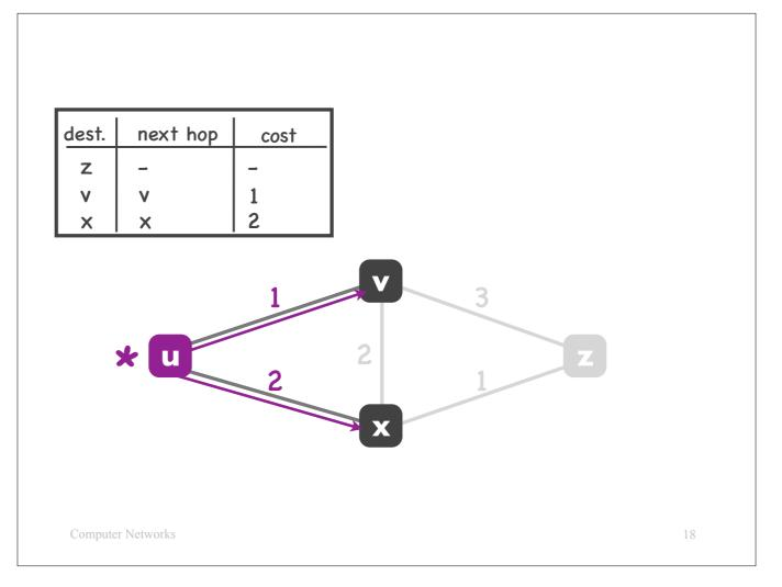
In the first step, the algorithm considers only the the links that are directly connected to router u.
