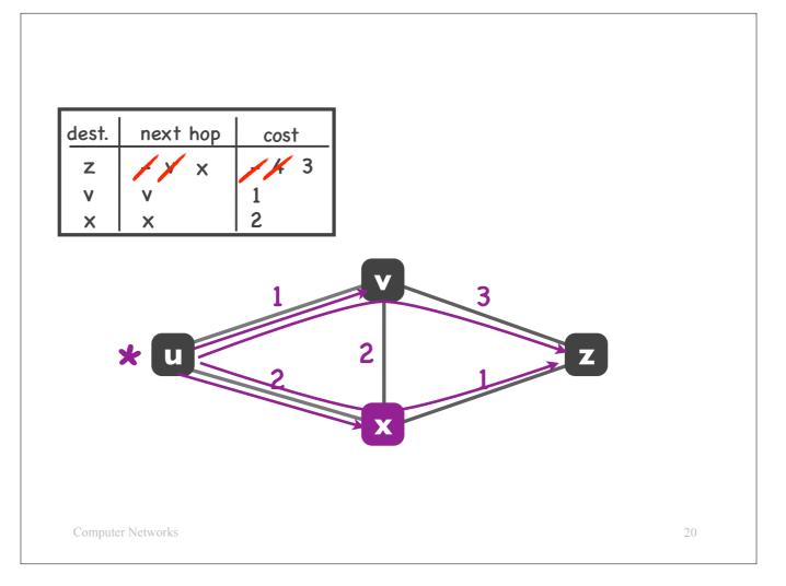
In the third step, the algorithm considers the other neighbor, router x, and the links that are directly connected to router x.
