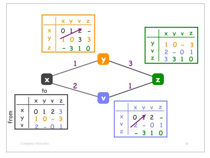
and updates its table accordingly (note that the new number 3 that appears in y's table is black, because it was computed based on information propagated by router x).
