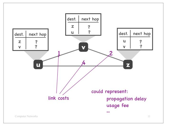
Suppose routers u and z are part of a 3-router topology.
