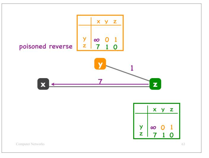
Then the neighbors exchange tables again, Router y learns that router z has a path to router x of cost 7...
