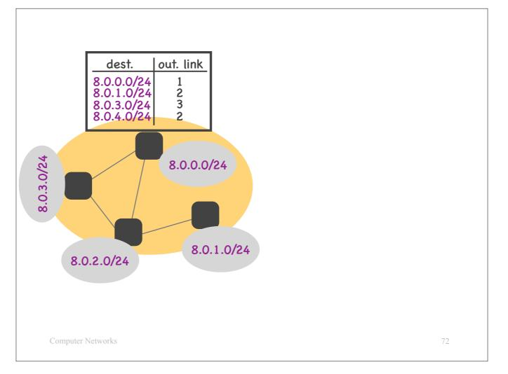
Consider this example AS, which has 4 routers, each providing connectivity to 1 IP subnet.
