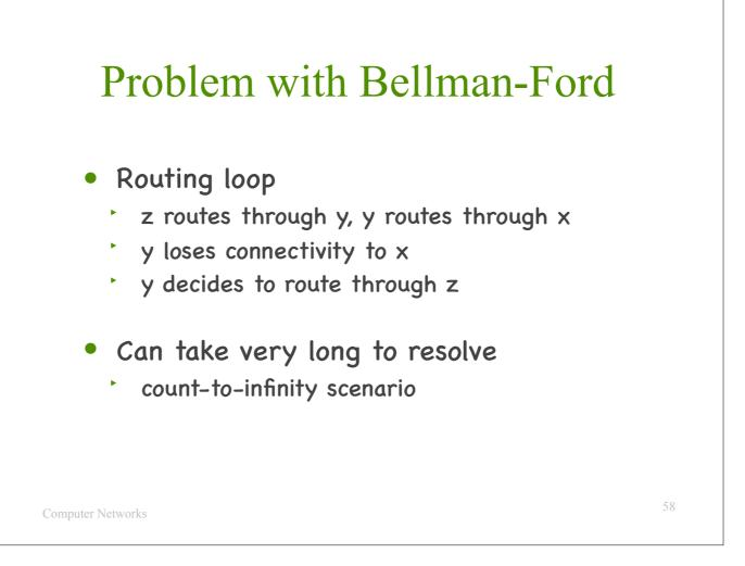
So: If we are not careful with the Bellman-Ford implementation (or any routing protocol implementation, for that matter), we may end up with routing loops,\_which may take a long time to resolve.
