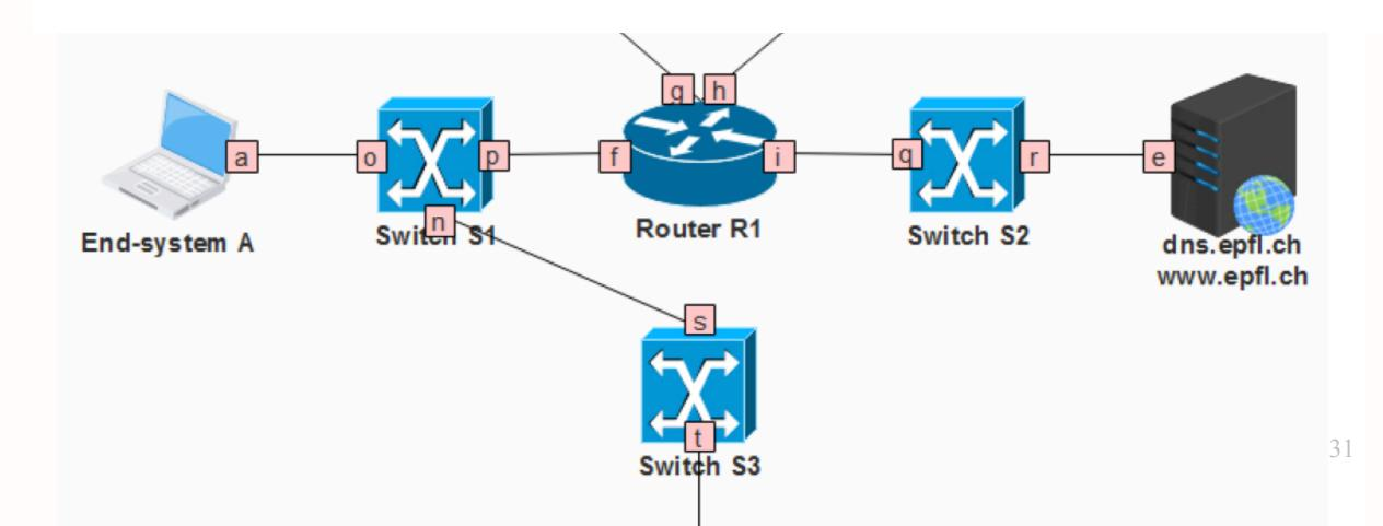
DNS request from A to server ARP request, MAC: A—broadcast ARP response, MAC: R1—A DNS request, MAC: A—R1, IP: A—DNS ARP request, MAC: R1—broadcast ARP response, MAC: DNS—R1 DNS request, MAC: R1—DNS, IP: A—DNS
