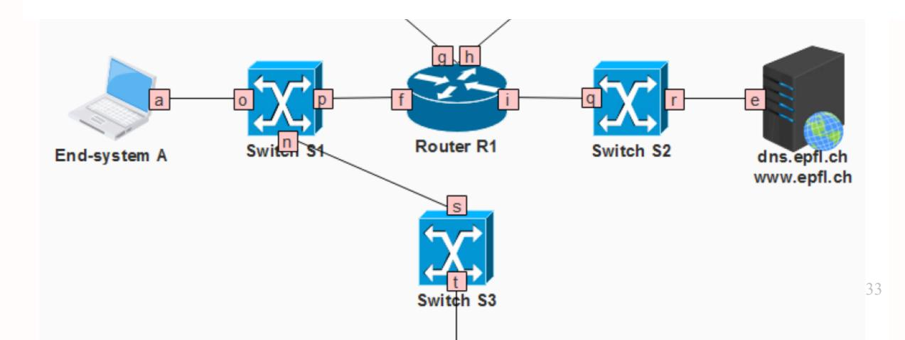
HTTP GET request from A to server TCP SYN, MAC: A-R1, IP: A-DNS TCP SYN, MAC: R1-DNS, IP: A-DNS TCP SYN ACK, MAC: DNS-R1, IP: DNS-A TCP SYN ACK, MAC: R1-A, IP: DNS-A HTTP GET request, MAC: A-R1, IP: A-DNS HTTP GET request, MAC: R1-DNS, IP: A-DNS
