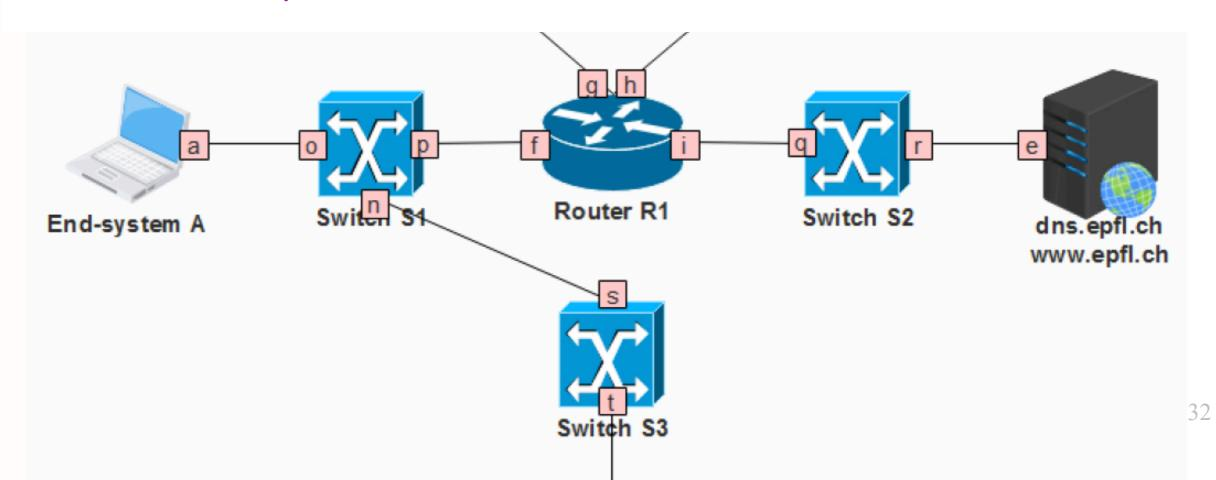
DNS response from server to A DNS response, MAC: DNS-R1, IP: DNS-A DNS response, MAC: R1-A, IP: DNS-A
