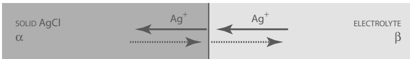
Figure 3.6 - Exchange equilibrium of \text{Ag}^+ ions between a crystal of \text{AgCl} and an aqueous solution
