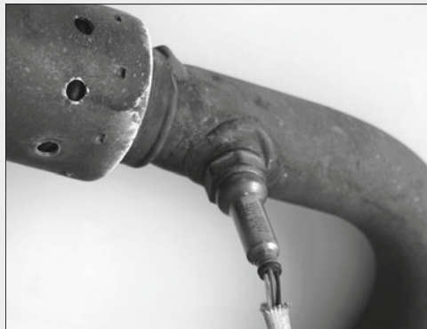
Photograph of a lambda sensor extracted from a car after use
