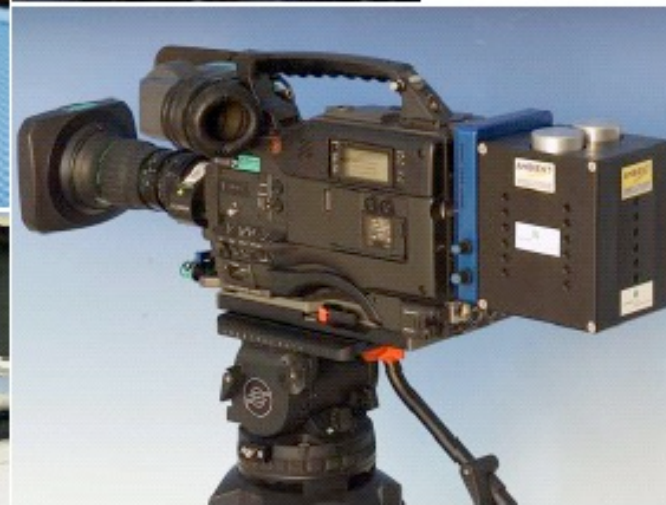
Professional camera with fuel cell
