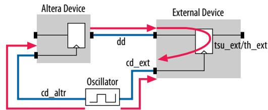
The calculation the TimeQuest analyzer performs to determine the typical out delay.
