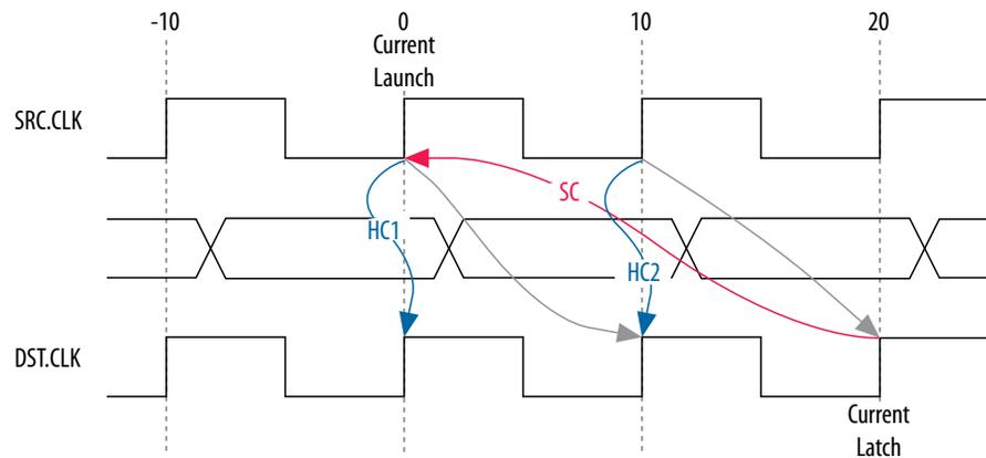
The calculation that the TimeQuest analyzer performs to determine the hold check. Both hold checks are equivalent.
