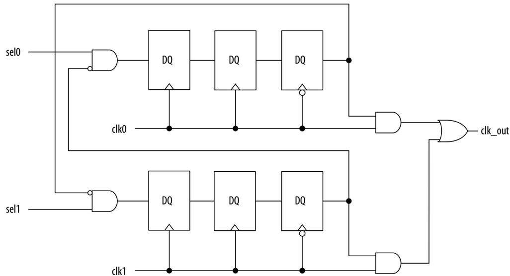
You can generalize this structure for any number of clock channels. The design ensures that no clock activates until all others are inactive for at least a few cycles, and that activation occurs while the clock is low. The design applies a `synthesis_keep` directive to the AND gates on the right side, which ensures there are no simultaneous toggles on the input of the `clk_out` OR gate.
