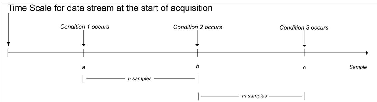
In this example, the SignalTap II Logic Analyzer does not write into the acquisition buffer until sample *a*, when Condition 1 occurs. Once sample *b* is reached, the `trigger value` command is evaluated. The logic analyzer continues to write into the buffer to finish the acquisition. The trigger flow specifies a `stop_store` command at sample *c*, *m* samples after the trigger point occurs.
