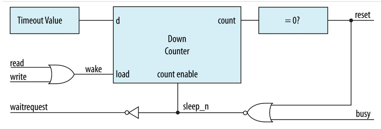
This example provides a schematic for the hardware-controlled sleep mode. If restoring the component to an active state takes a long time, use a long timeout value so that the component is not continuously entering and exiting sleep mode. The slave interface must remain functional while the rest of the component is in sleep mode. When the component exits sleep mode, the component must assert the `waitrequest` signal until it is ready for read or write accesses.
