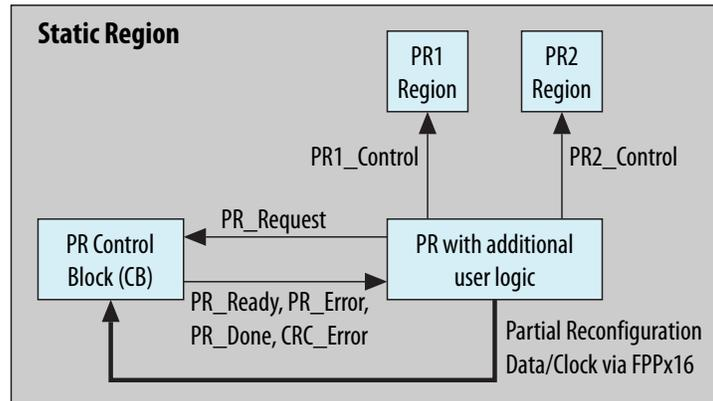
After the FPGA device has been configured with a full chip configuration at least once, the `INIT_DONE` signal is released, and the signal is asserted high due to the external resistor on this pin. The `INIT_DONE` signal must be assigned to a pin to monitor it externally. When a full chip configuration is complete, and the device is in user mode, the following steps describe the PR sequence:
