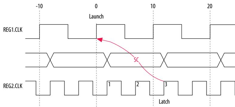
The timing diagram for default hold check analysis the TimeQuest analyzer performs with an end multicycle setup value of three.
