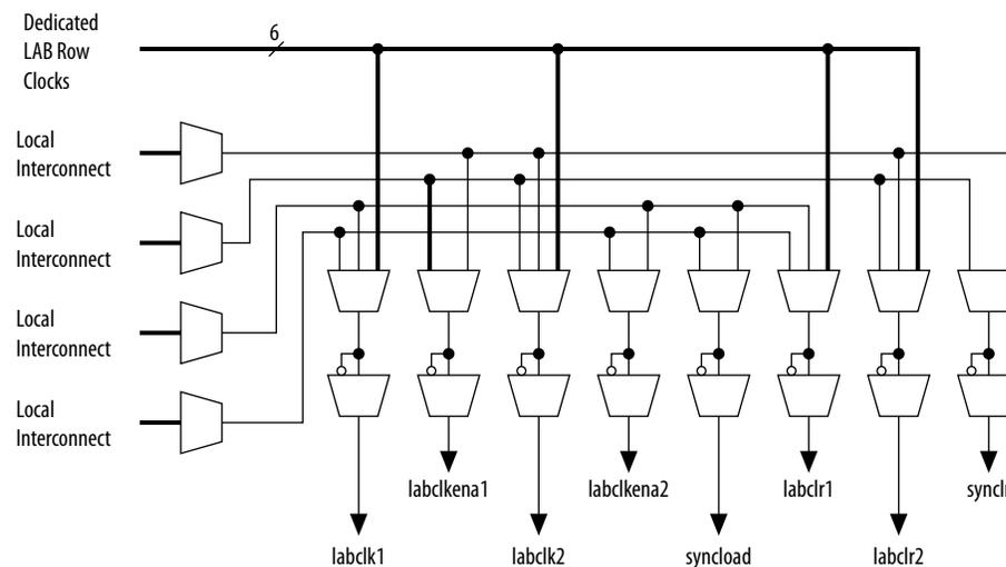
To reduce LAB-wide clock power consumption without disabling the entire clock tree, use the LAB-wide clock enable to gate the LAB-wide clock. The Quartus Prime software automatically promotes register-level clock enable signals to the LAB-level. All registers within an LAB that share a common clock and clock enable are controlled by a shared gated clock. To take advantage of these clock enables, use a clock enable construct in the relevant HDL code for the registered logic.
