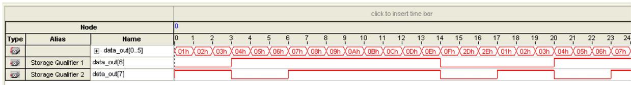
(1) Storage Qualifier condition is set up to evaluate data\_out[6] AND data\_out[7].
