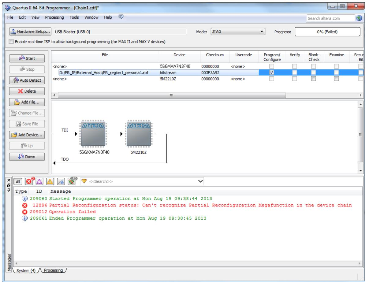
4. Configure the valid **.rbf** in JTAG debug mode with the Quartus Prime Programmer.
