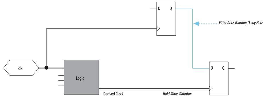
However, if your design still has internal hold time violations between registers, correct the violations by manually adding some delays by instantiating LCELL primitives, or by making changes to your design, such as using a clock enable signal instead of a derived or gated clock.
