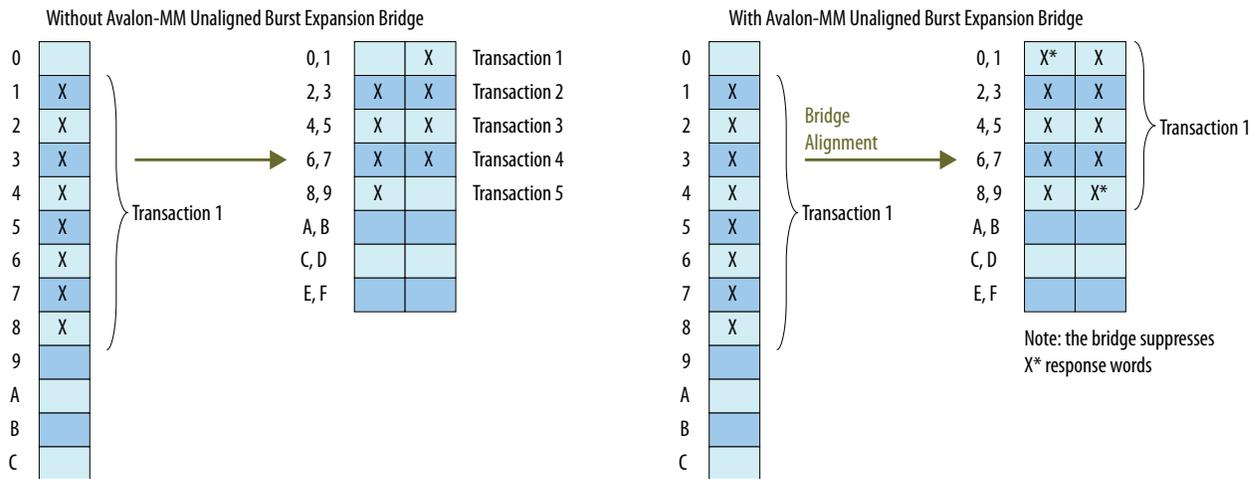
Because the target slave has a 64-bit data width, address 1 is unaligned in the slave's address space. As a result, several smaller burst transactions are needed to request the data associated with the master's read burst command.
