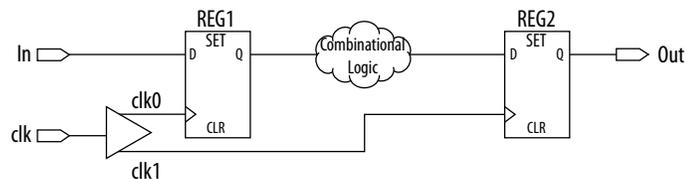
The timing diagram for default setup check analysis that the TimeQuest analyzer performs.
