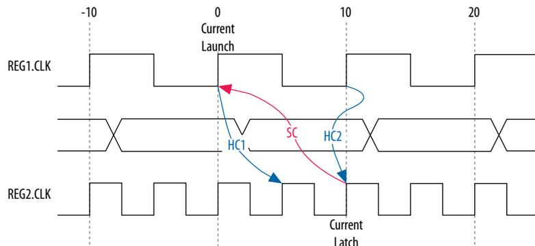
The calculation that the TimeQuest analyzer performs to determine the hold check.
