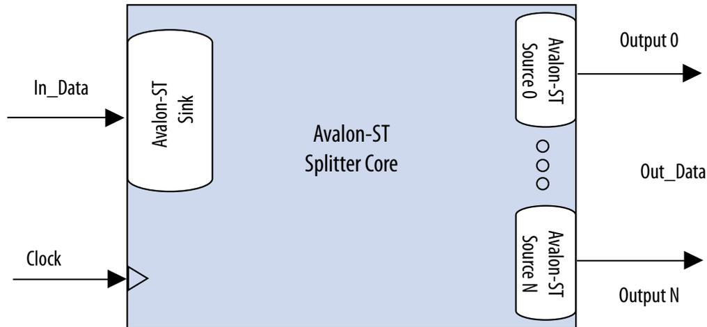
The Avalon-ST Splitter core copies input signals from the input interface to the corresponding output signals of each output interface without altering the size or functionality. This includes all signals except for the `ready` signal. The core includes a clock signal to determine the Avalon-ST interface and clock domain where the core resides. Because the splitter core does not use the `clock` signal internally, latency is not introduced when using this core.
