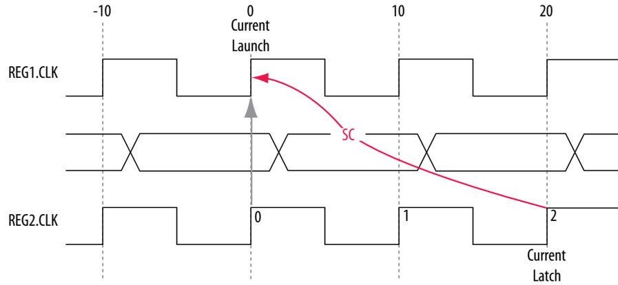
The calculation that the TimeQuest analyzer performs to determine the setup check.
