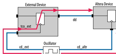
The calculation the TimeQuest analyzer performs to determine the typical input delay.
