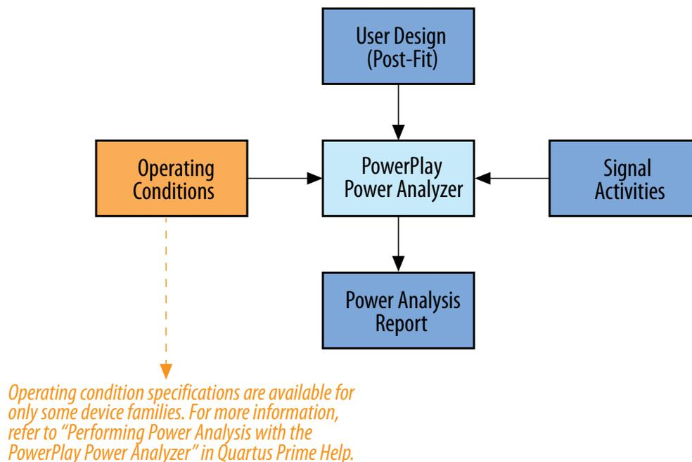
To obtain accurate I/O power estimates, the PowerPlay Power Analyzer requires you to synthesize your design and then fit your design to the target device. You must specify the electrical standard on each I/O cell and the board trace model on each I/O standard in your design.
