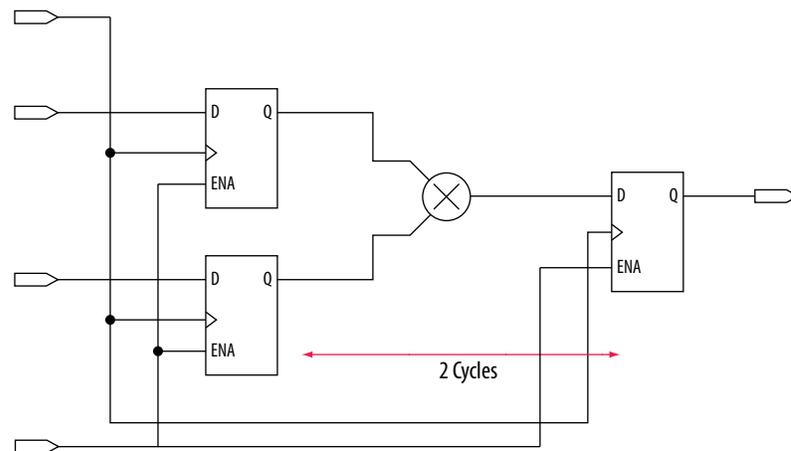
A register-to-register path used for the default setup and hold relationship, the respective timing diagrams for the source and destination clocks, and the default setup and hold relationships, when the source clock, `src_clk`, has a period of 10 ns and the destination clock, `dst_clk`, has a period of 5 ns. The default setup relationship is 5 ns; the default hold relationship is 0 ns.
