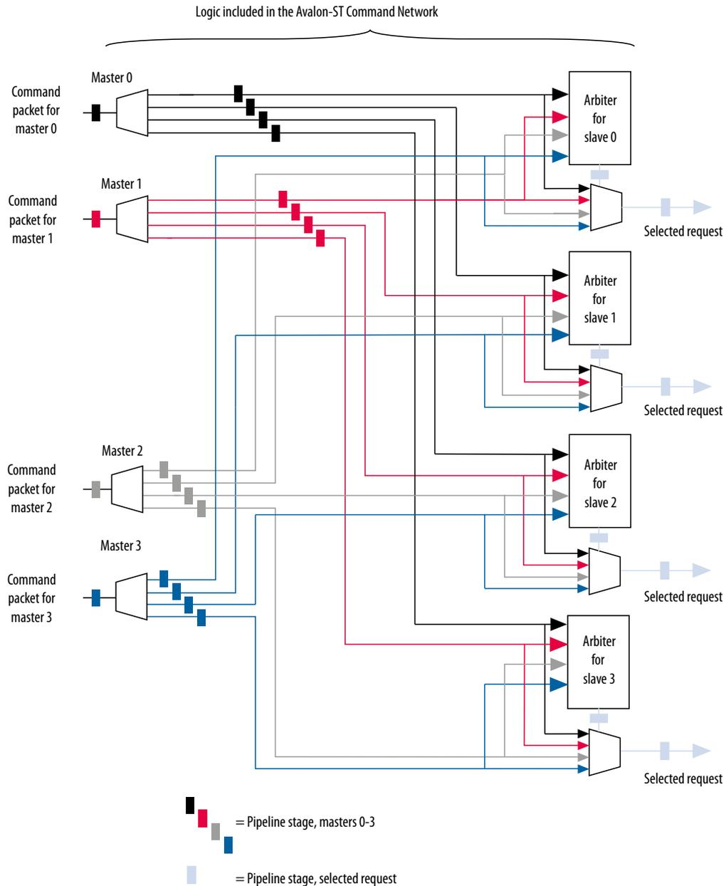
**Note:** If you specify a **Limit interconnect pipeline stages** to parameter greater than zero, the output of the Arbiter is registered. Registering this output reduces the amount of combinational logic between the master and the interconnect, increasing the  $f_{MAX}$  of the system.
