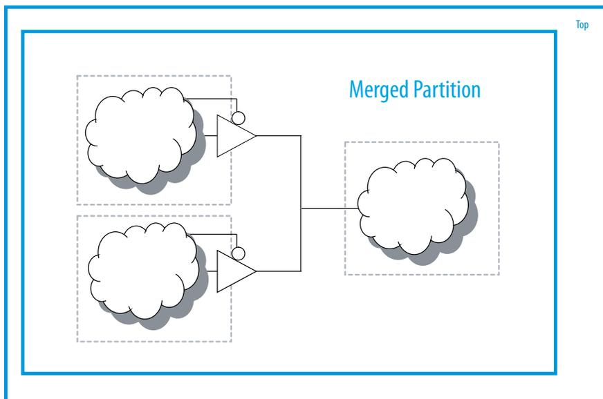
Merged partition allows synthesis to convert tri-state logic into combinational logic.
