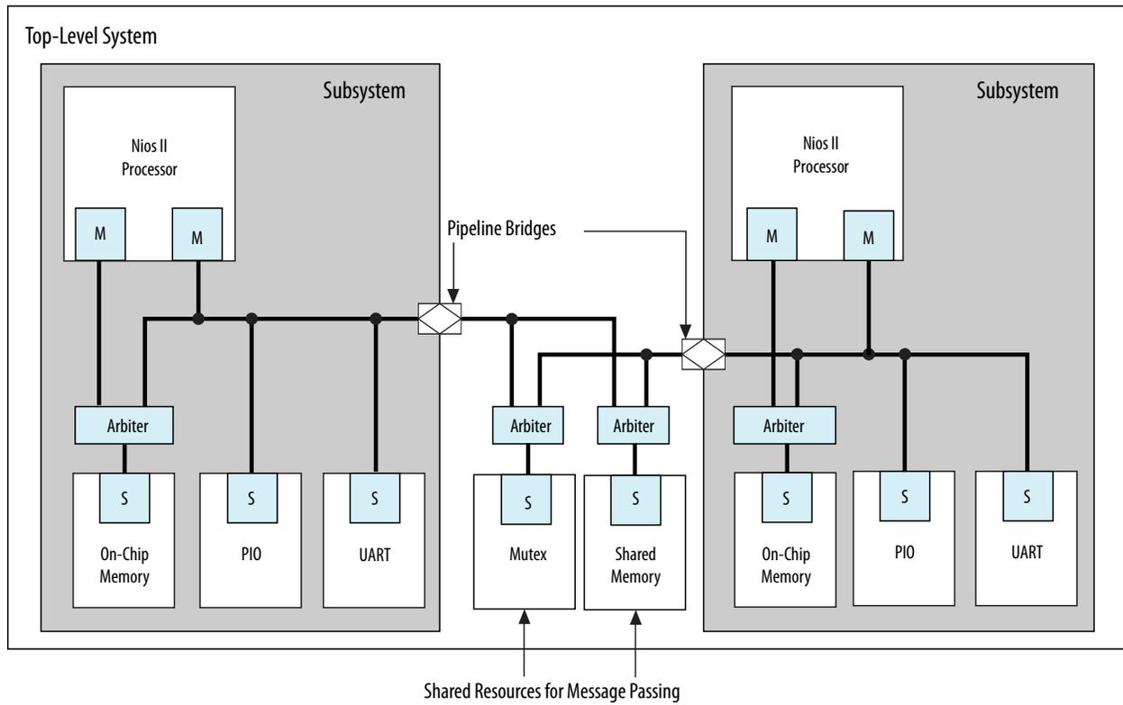
In this example, two Nios II processor subsystems share resources for message passing. Bridges in each subsystem export the Nios II data master to the top-level system that includes the mutex (mutual exclusion component) and shared memory component (which could be another on-chip RAM, or a controller for an off-chip RAM device).
