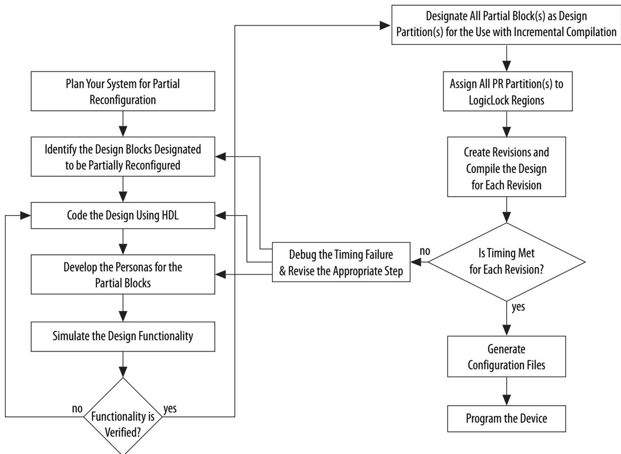
The PR design flow requires more initial planning than a standard design flow. Planning requires setting up the design logic for partitioning, and determining placement assignments to create a floorplan. Well-
