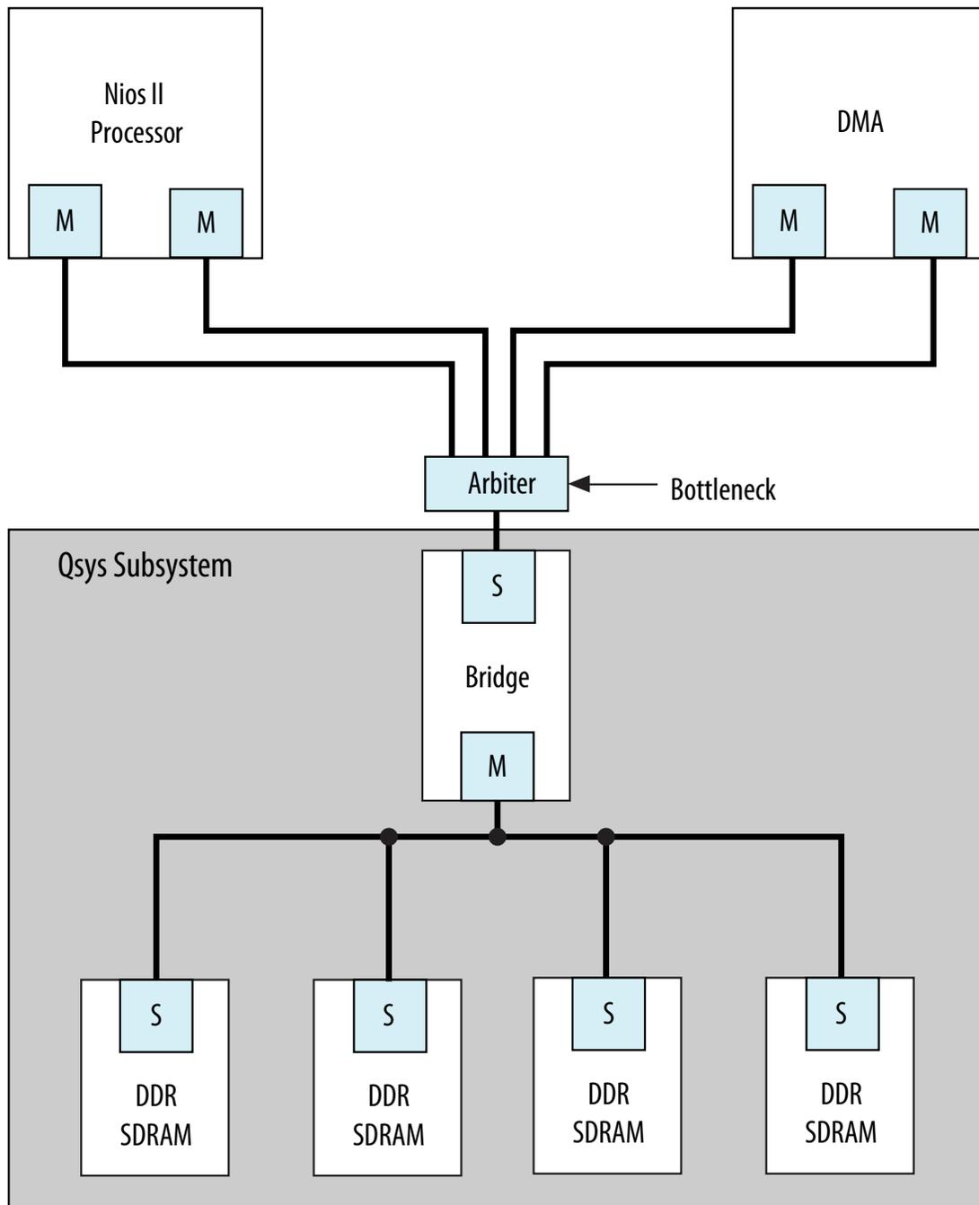
A memory subsystem with one bridge that acts as a single slave interface for the Avalon-MM Nios II and DMA masters, which results in a bottleneck architecture. The bridge acts as a bottleneck between the two masters and the memories.
