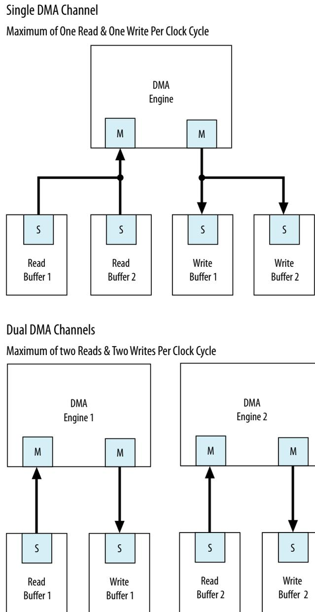
In this example, the system can sustain more concurrent read and write operations by including more DMA engines. Accesses to the read and write buffers in the top system are split between two DMA engines, as shown in the Dual DMA Channels at the bottom of the figure.
