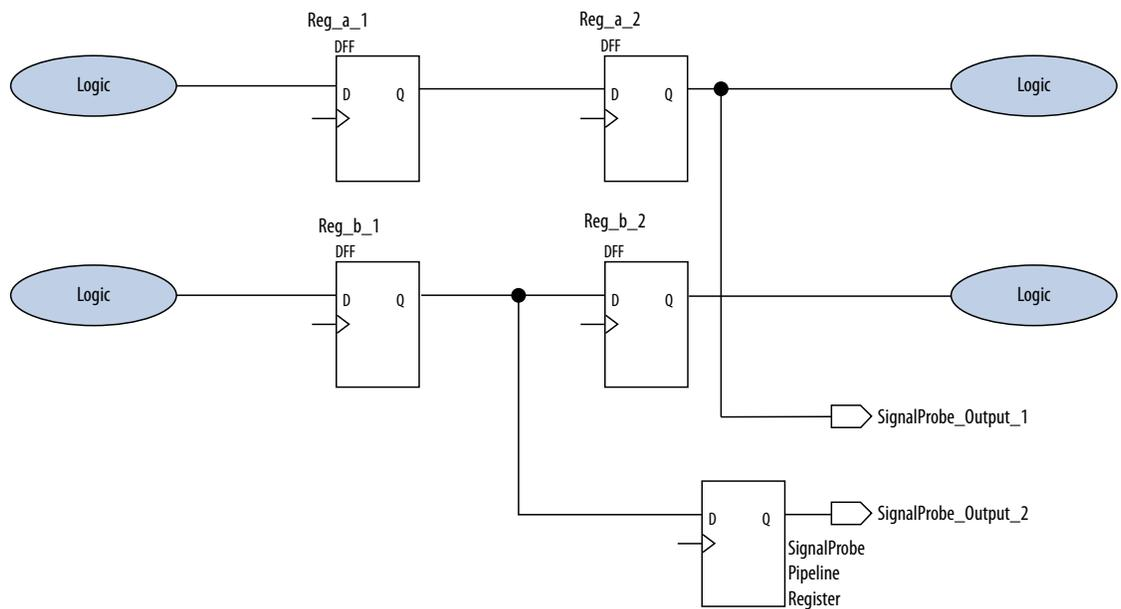
In addition to clock input for pipeline registers, you can also specify a reset signal pin for pipeline registers. To specify a reset pin for pipeline registers, use the Tcl command `make_sp`.
