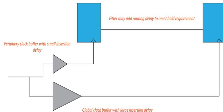
To identify cases where a path has different clock network types, review the path in the TimeQuest timing analyzer, and check nodes along the source and destination clock paths. Also, check the source and destination clock frequencies to see whether they are the same, or multiples, and whether there are multicycle exceptions on the paths. In some cases, cross-domain paths may also be false by intent, so make sure there are false path exceptions on those.
