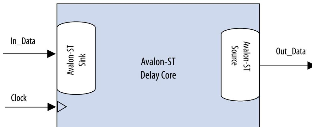
The Delay core adds a delay between the input and output interfaces. The core accepts transactions presented on the input interface and reproduces them on the output interface  $N$  cycles later without changing the transaction.
