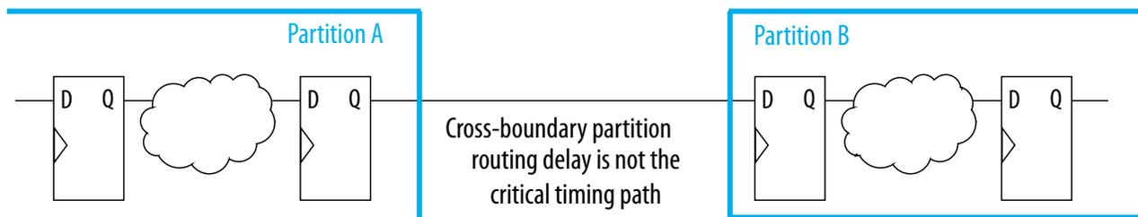
If a design cannot include both input and output registers for each partition due to latency or resource utilization concerns, choose to register one end of each connection. If you register every partition output, for example, the combinational logic that occurs in each cross-partition path is included in one partition so that it can be optimized together.
