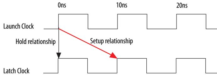
In timing analysis, and with the TimeQuest analyzer specifically, you create clock constraints and assign those constraints to nodes in your design. These clock constraints provide the structure required for repeatable data relationships. The primary relationships between clocks, in the same or different domains, are the setup relationship and the hold relationship.
