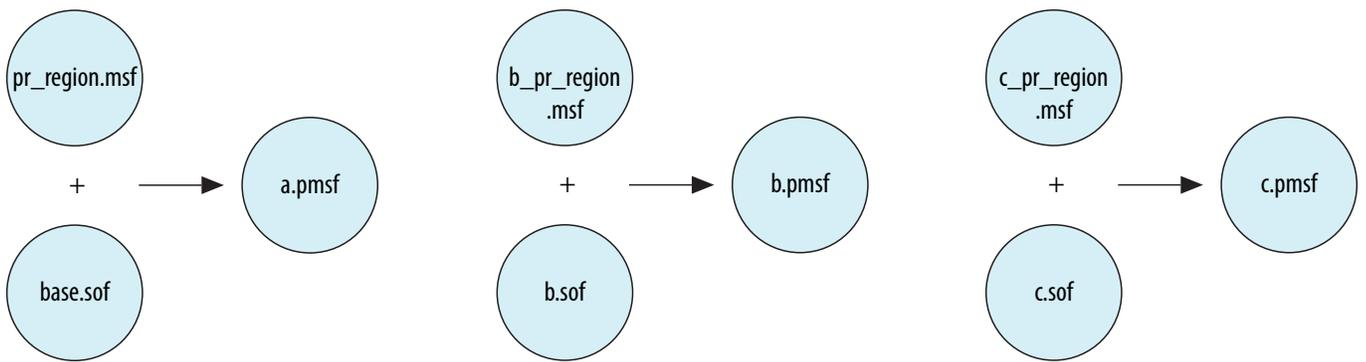
The **.msf** file helps determine the PR region from each of the **.sof** files during the PR bitstream computation.
