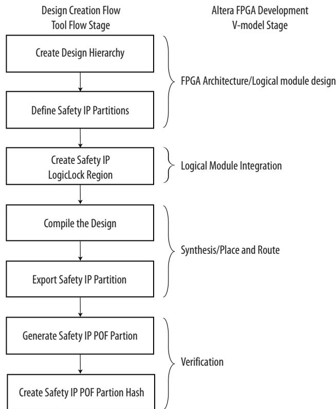
The design creation flow becomes active when you have a valid safety IP partition in your Quartus Prime project and that safety IP partition does not have place and route data from a previous compile. In the design creation flow, the Assembler generates a Partial Settings Mask (**.psm**) file for each safety IP partition. Each **.psm** file contains a list of programming bits for its respective safety IP partition.
