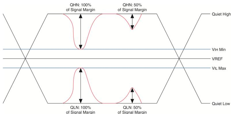
The figure shows four noise events, two on QH signals and two on QL signals. The two noise events on the right-side of the figure consume 50 percent of the signal margin and do not cause voltage functional errors. However, the two noise events on the left side of the figure consume 100 percent of the signal margin, which can cause a voltage functional error.
