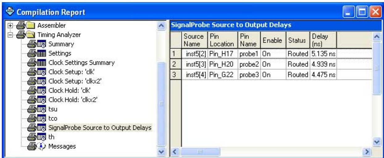
**Note:** After a SignalProbe compilation, the processing screen of the Messages window also provides the results for each SignalProbe pin and displays slack information for each successfully routed SignalProbe pin.
