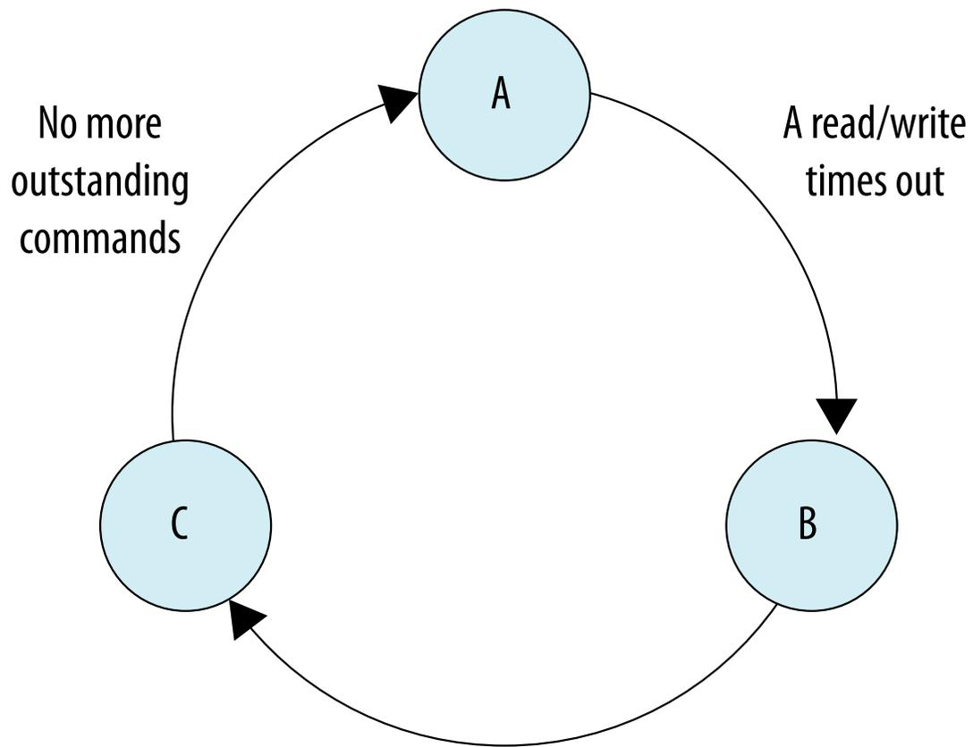
The AXI Timeout Bridge is notified that the slave is reset.
