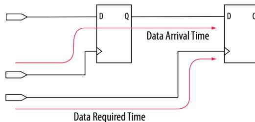
The basic calculations for data arrival and data required times including the launch and latch edges.
