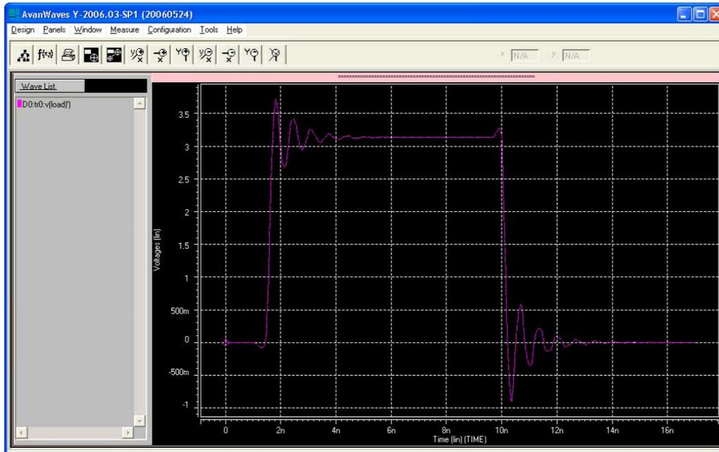
If there is a discontinuity or any other anomalies at the destination, adjust the board description in the Quartus Prime Board Trace Model, or in the generated HSPICE model files to change the termination scheme or adjust termination component values. After making these changes, regenerate the HSPICE files if necessary, and rerun the simulation to verify whether your adjustments solved the problem.
