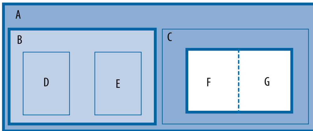
You can create partition assignments to any design instance. The instance can be defined in HDL or schematic design, or come from a third-party synthesis tool as a VQM or EDIF netlist instance.
