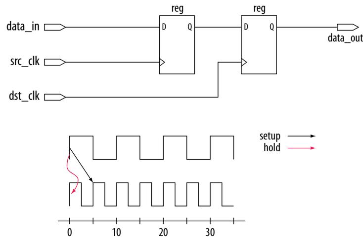
To accommodate the system requirements you can modify the default setup and hold relationships with a multicycle timing exception.
