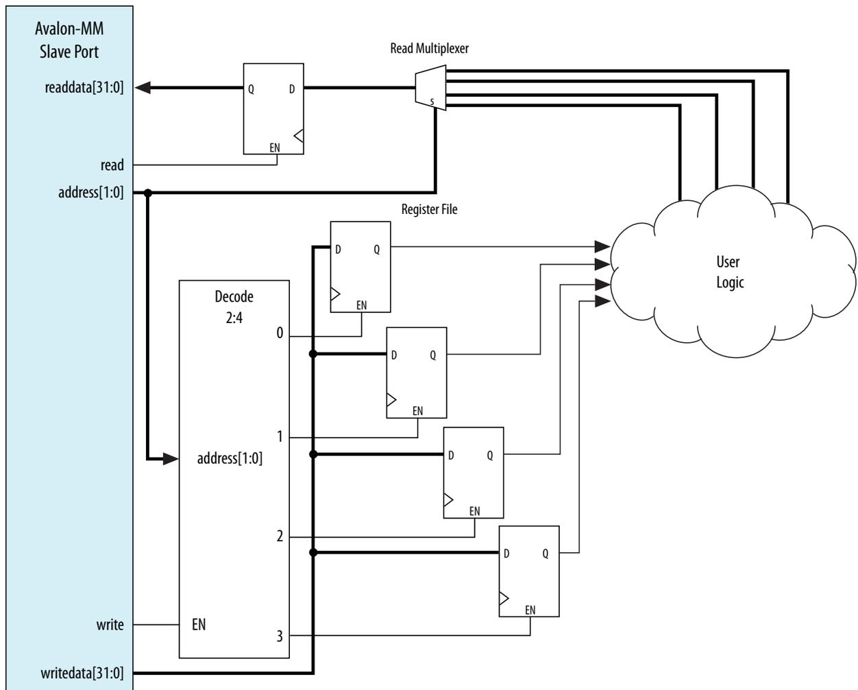
This slave component has write wait states and one read wait state. Alternatively, if you want high throughput, you may set both the read and write wait states to zero, and then specify a read latency of one, because the component also supports pipelined reads.
