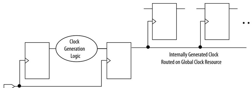
Registering the output of combinational logic ensures that glitches generated by the combinational logic are blocked at the data input of the register.
