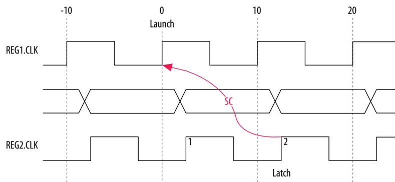
The timing diagram for default hold check analysis that the TimeQuest analyzer performs with an end multicycle setup value of two.
