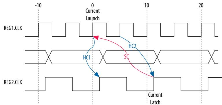
The calculation that the TimeQuest analyzer performs to determine the hold check.
