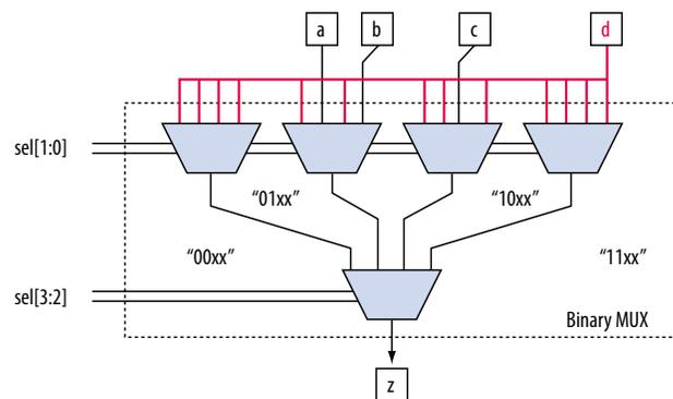
Depending on the number of multiplexers in the chain, the timing delay through this chain can become large, especially for device families with 4-input LUTs.
