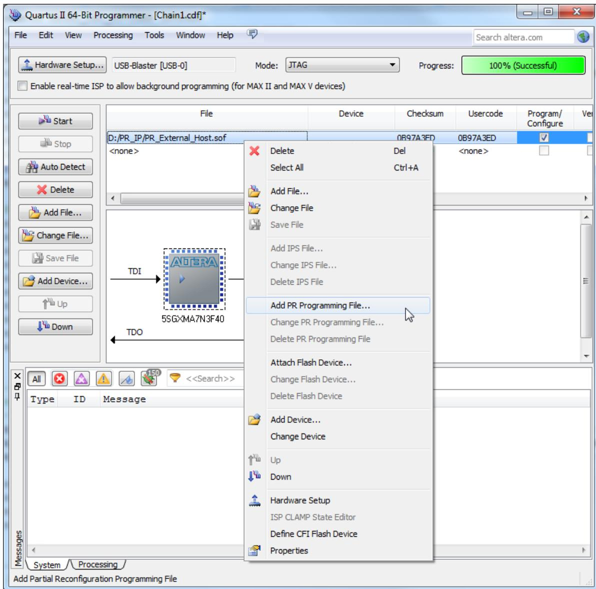
2. After adding the PR bitstream, you can change or delete the Partial Reconfiguration programming file by clicking **Change PR Programming File** or **Delete PR Programming File**.
