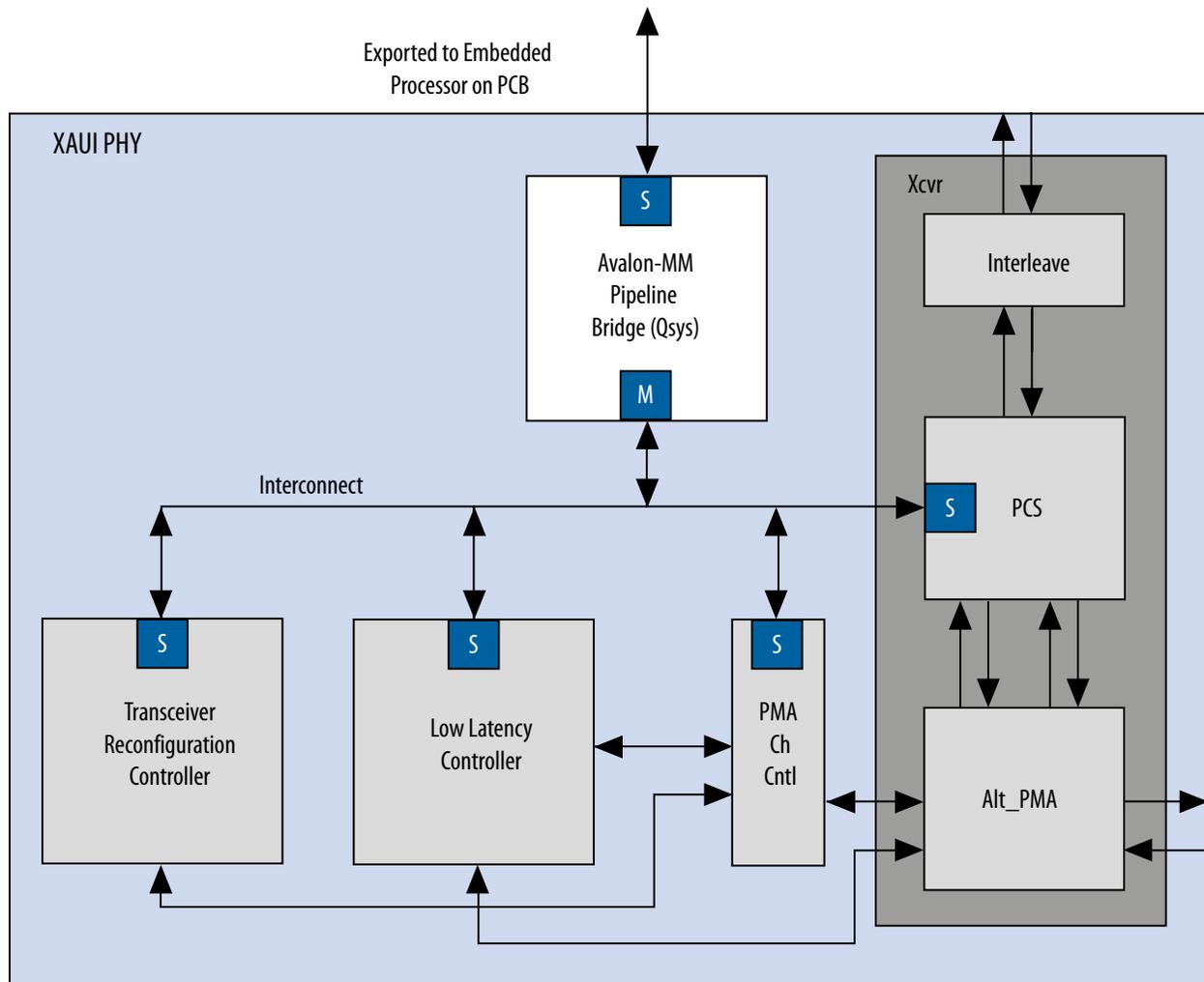
Because the slave interface is exported to the pins of the device, having a single slave port, rather than separate ports for each slave device, reduces the pin count of the FPGA.
