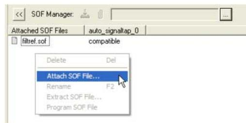
As you switch between configurations in the Data Log, you can extract the SOF that is compatible with that particular configuration. You can use the programmer in the SignalTap II Logic Analyzer to download the new SOF to the FPGA, ensuring that the configuration of your **.stp** always matches the design programmed into the target device.
