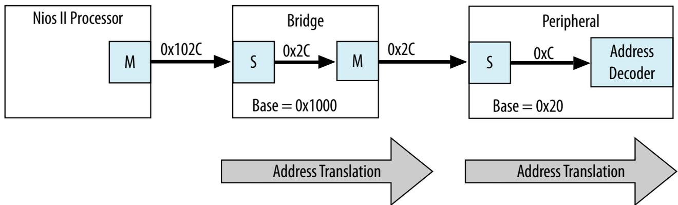
In this example, the Nios II processor connects to a bridge located at base address 0x1000, a slave connects to the bridge master interface at an offset of 0x20, and the processor performs a write transfer to the fourth 32-bit or 64-bit word within the slave. Nios II drives the address 0x102C to interconnect, which is within the address range of the bridge. The bridge master interface drives 0x2C, which is within the address range of the slave, and the transfer completes.
