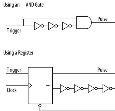
A trigger signal feeds both inputs of a 2-input AND gate, but the design adds inverters to create a delay chain to one of the inputs. The width of the pulse depends on the time differences between path that feeds the gate directly, and the path that goes through the delay chain. This is the same mechanism responsible for the generation of glitches in combinational logic following a change of input values. This technique artificially increases the width of the glitch.
