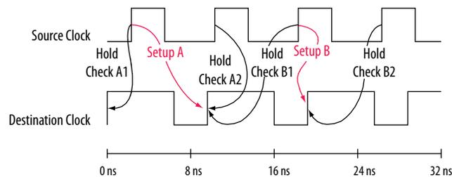
**Figure 6-12: Clock Hold Slack for Internal Register-to-Register Paths**
