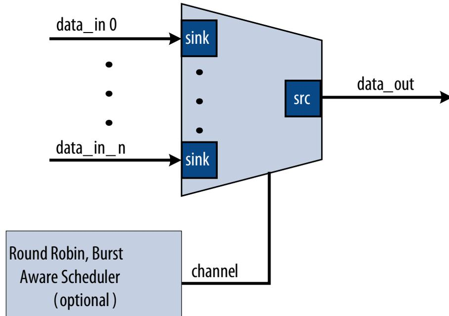
The multiplexer includes an optional channel signal that enables each input interface to carry channelized data. The output interface channel width is equal to:
