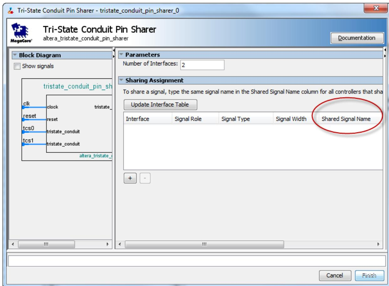
**Note:** All tri-state conduit components are connected to a pin sharer must be in the same clock domain.
