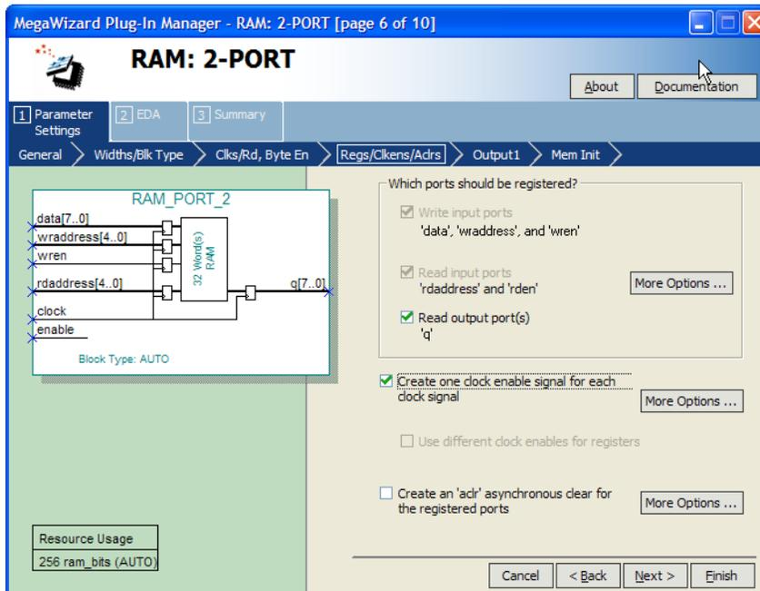
For example, consider a design that contains a 32-bit-wide M4K memory block in ROM mode that is running at 200 MHz. Assuming that the output of this block is only required approximately every four cycles, this memory block will consume 8.45 mW of dynamic power according to the demands of the downstream logic. By adding a small amount of control logic to generate a read clock enable signal for the memory block only on the relevant cycles, the power can be cut 75% to 2.15 mW.
