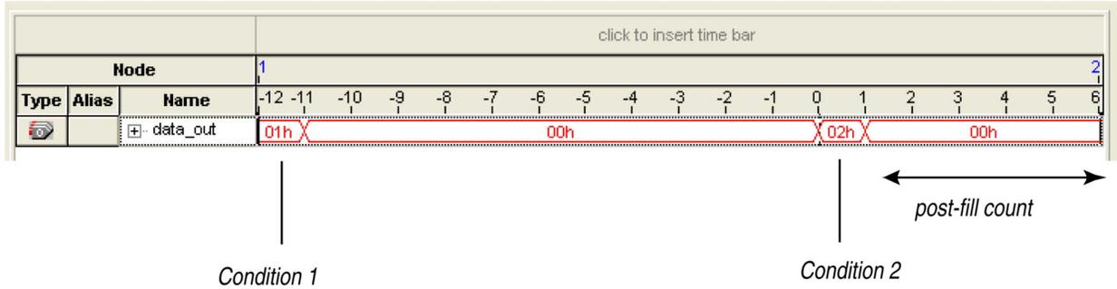
Figure 13-36: Storage Qualification with Post-Fill Count Value Greater than *m* (Acquisition Indefinitely Paused)
