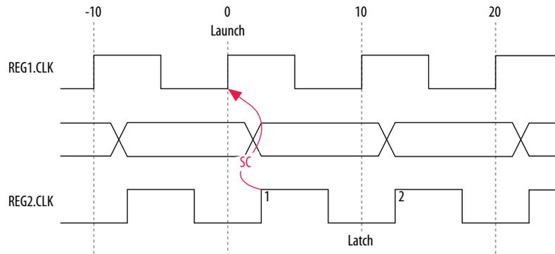
The calculation that the TimeQuest analyzer performs to determine the setup check.
