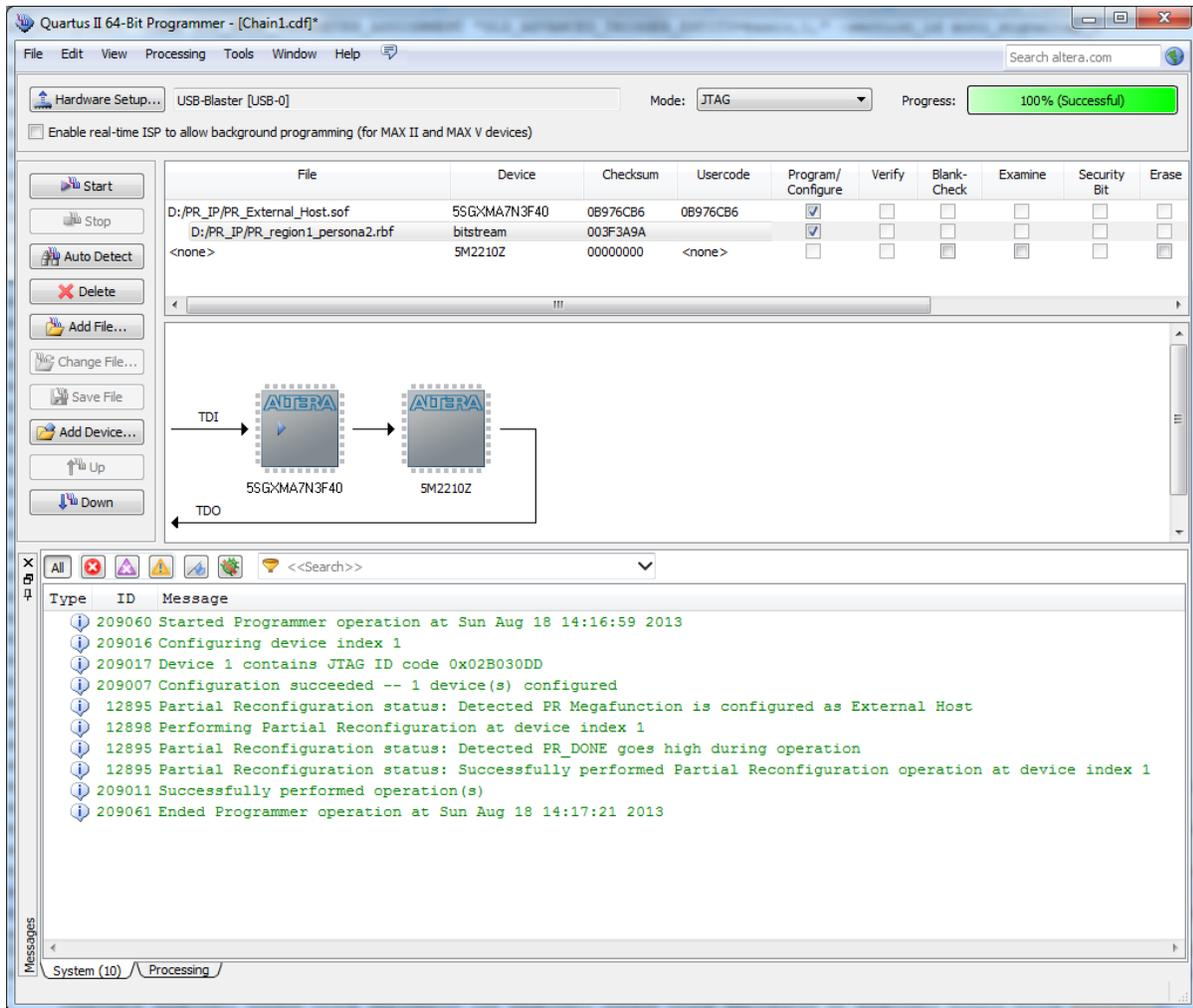
5. The JTAG debug mode is also supported if the PR IP core is pre-programmed on the specified device.
