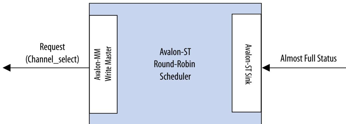
In a multi-channel component, the component can store data either in the sequence that it comes in (FIFO), or in segments according to the channel. When data is stored in segments according to channels, a scheduler is needed to schedule the read operations.
