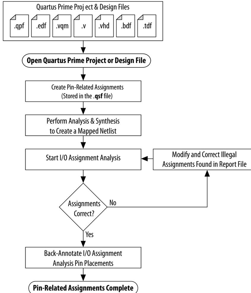
Even if I/O assignment analysis passes on incomplete design files, you may still encounter errors during full compilation. For example, you can assign a clock to a user I/O pin instead of assigning it to a dedicated clock pin, or design the clock to drive a PLL that you have not yet instantiated in the design. This occurs because I/O assignment analysis does not account for the logic that the pin drives, and does not verify that only dedicated clock inputs can drive the a PLL clock port.
