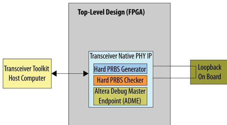
Figure 11-16: Four Channel Loopback Mode for Stratix V / 28nm
