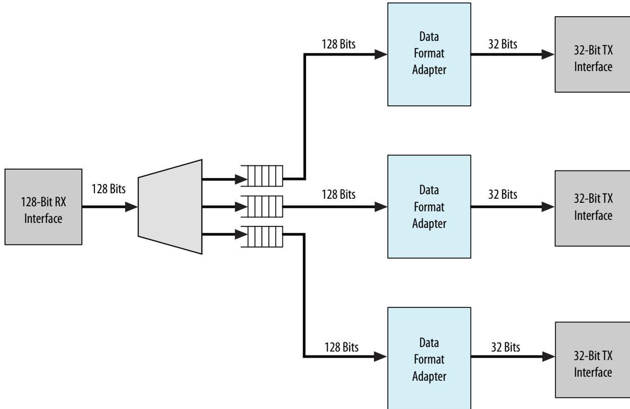
**Avalon-ST Data Format Adapter Input Interface Parameters**
