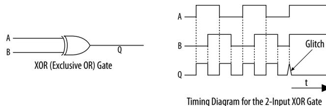
This glitch can propagate to subsequent logic and create unnecessary switching activity, increasing power consumption. Circuits with many XOR functions, such as arithmetic circuits or cyclic redundancy check (CRC) circuits, tend to have many glitches if there are several levels of combinational logic between registers.
