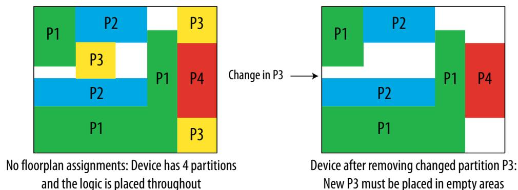
The Fitter has a more difficult task because of more difficult physical constraints, and as a result, compilation time often increases. The Fitter might not be able to find any legal placement for the logic in partition P3, even if it could in the initial compilation. Additionally, if the Fitter can find a legal placement, the quality of results often decreases in these cases, sometimes dramatically, because the new partition is now scattered throughout the device.
