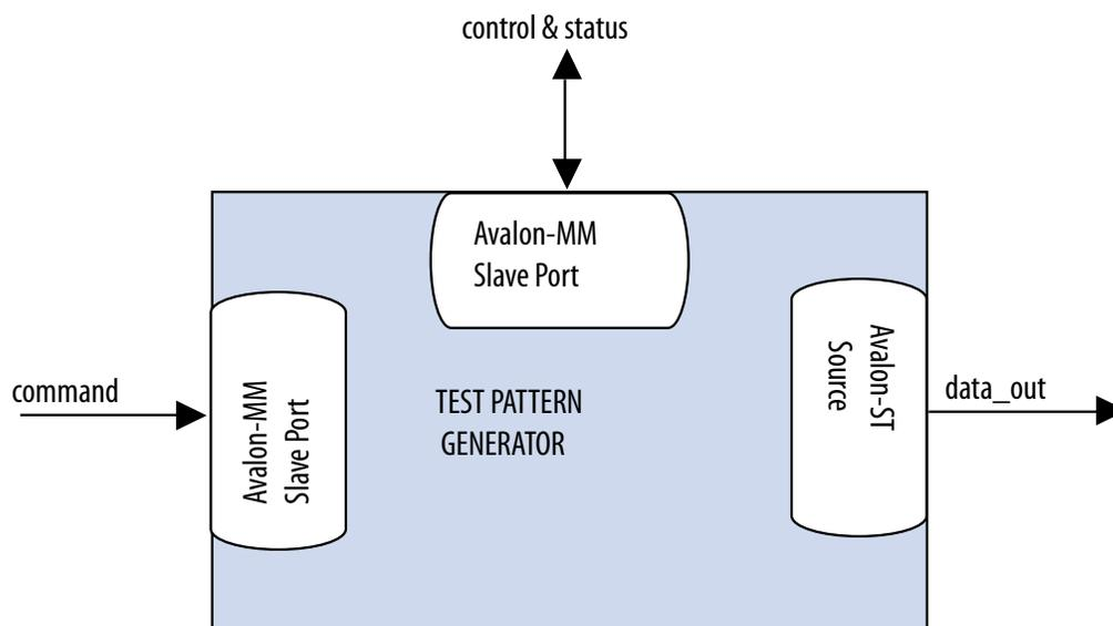
The data pattern is calculated as:  $Symbol\ Value = Symbol\ Position\ in\ Packet \oplus Data\ Error\ Mask$ . Data that is not organized in packets is a single stream with no beginning or end. The test pattern generator has a throttle register that is set via the Avalon-MM control interface. The test pattern generator uses the value of the throttle register in conjunction with a pseudo-random number generator to throttle the data generation rate.
