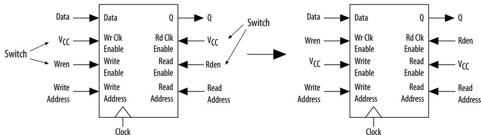
Memory transformation effectively moves the read-enable and write-enable signals to the respective read-clock enable and write-clock enable signals. By using this technique, memory ports are shut down when they are not accessed. This significantly reduces your design’s memory power consumption. For Stratix IV and Stratix V devices, the memory transformation takes place at the Fitter level by selecting the **Normal compilation** settings for the power optimization option.
