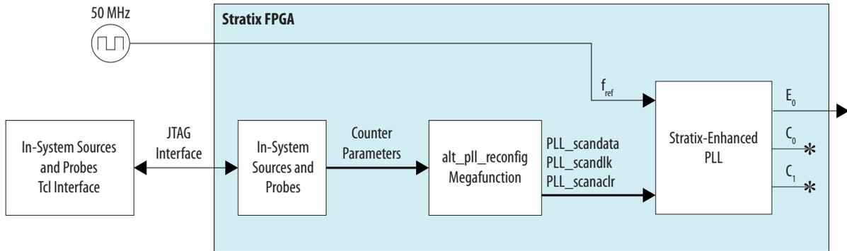
This design example was created using a Nios<sup>®</sup> II Development Kit, Stratix Edition. The file **sourceprobe\_DE\_dynamic\_pll.zip** contains all the necessary files for running this design example, including the following:
