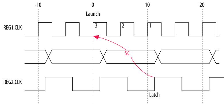
The timing diagram for default hold check analysis the TimeQuest analyzer performs for a start multicycle setup value of three.
