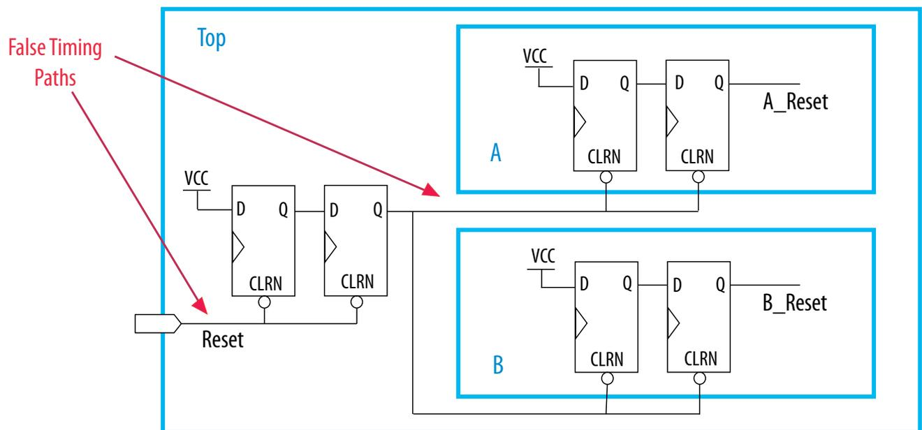
This circuit design can help you achieve timing closure and partition independence for your global reset signal. Evaluate the circuit and consider how it works for your design.
