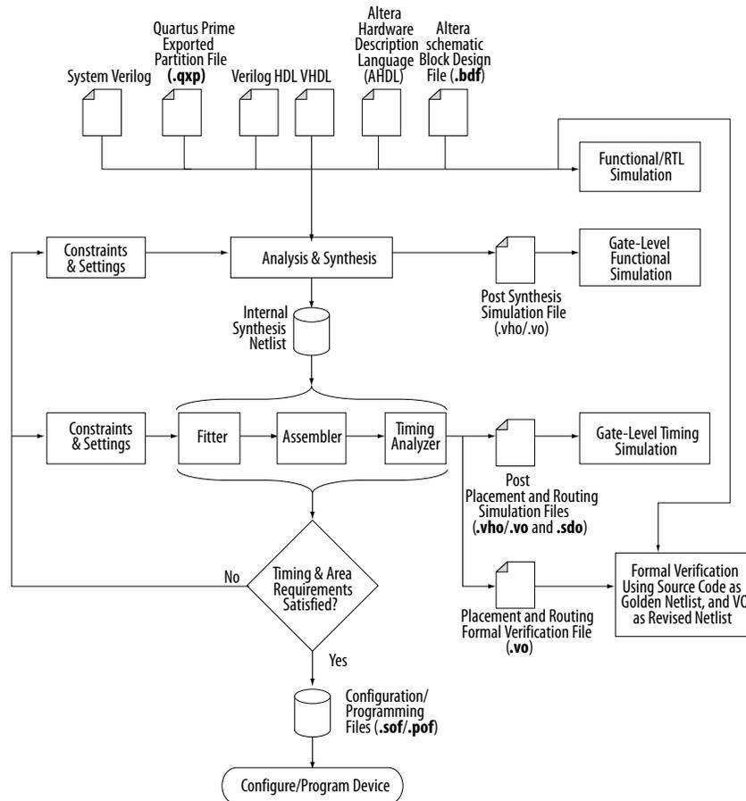
The Quartus Prime Integrated Synthesis design and compilation flow consists of the following steps:
