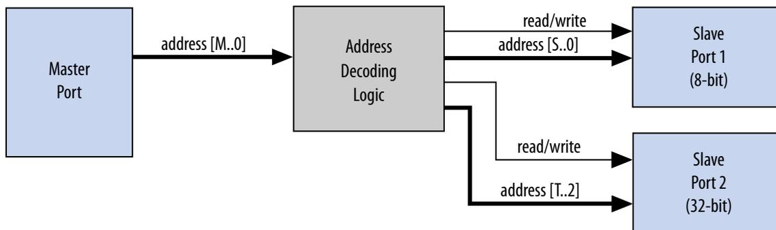
Figure 7-21: Address Decoding Base Settings
