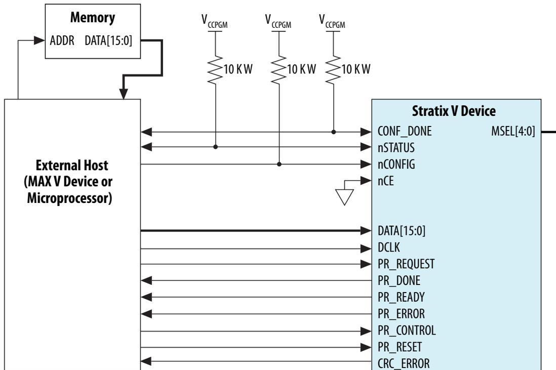
**Note:** If you don't care to write an external host controller, you can implement an external host with the Partial Reconfiguration IP core on a MAX 10 or other FPGA device.
