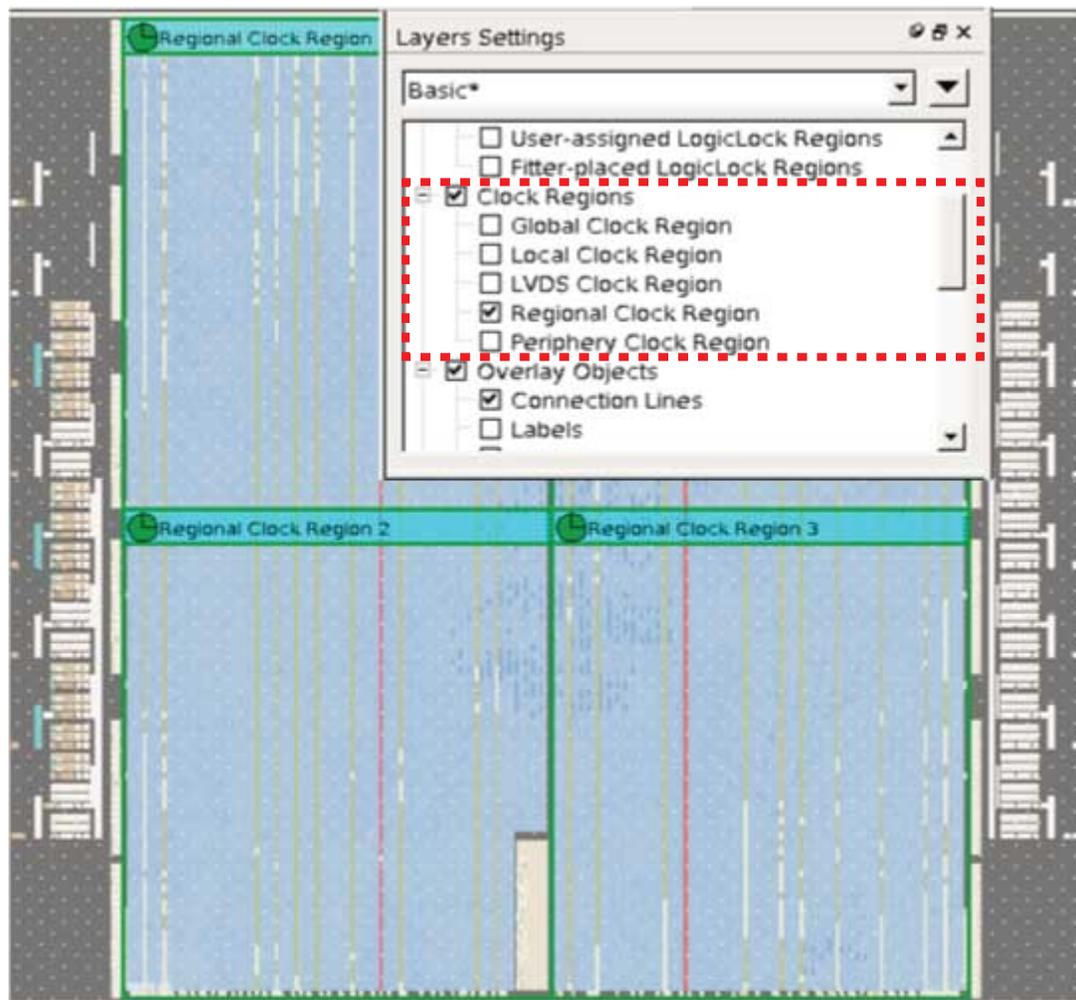
Timing failure can occur when the I/O interface at the top of the device connects to logic driven by a regional clock which is in one quadrant of the device, and placement restrictions force long paths to and from some of the I/Os to logic across quadrants.
