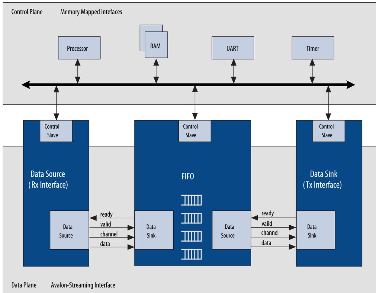
**Figure 7-23: Avalon-ST Connection Between the Source and Sink**
