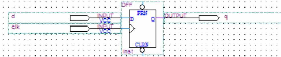
If the top-level design instantiates the subdesign with a single fan-out directly feeding an output pin, and designates the subdesign as a separate design partition, the Quartus Prime software can perform cross-partition register packing because the single partition port feeds the output pin directly.
