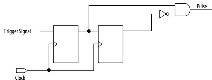
The pulse width is always equal to the clock period. This pulse generator is predictable, can be verified with timing analysis, and is easily moved to other architectures, devices, or speed grades.
