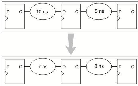
Retiming can create multiple registers at the input of a combinational block from a register at the output of a combinational block. In this case, the new registers have the same clock and clock enable. The asynchronous control signals and power-up level are derived from previous registers to provide equivalent functionality. Retiming can also combine multiple registers at the input of a combinational block to a single register.
