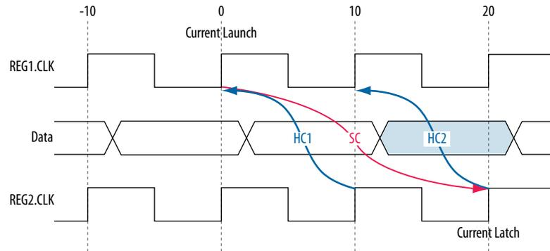
The calculation that the TimeQuest analyzer performs to determine the hold check. Both hold checks are equivalent.
