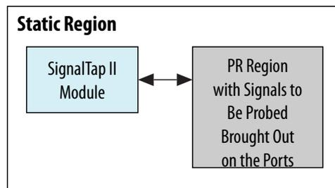
You can use other on-chip debug features in the Quartus Prime software, such as the In-System Sources and Probes or SignalProbe, to debug a PR design. As in the case of SignalTap, In-System Sources and Probes can only be instantiated within the static region of a PR design. If you have to probe any signal inside the PR region, you must bring those signals to the ports of the PR region in order to monitor them within the static region of the design.
