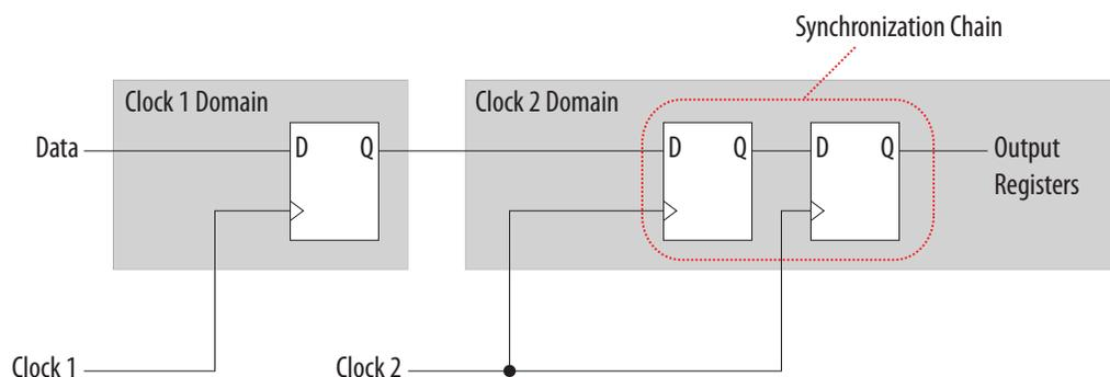
The path between synchronization registers can contain combinational logic as long as all registers of the synchronization register chain are in the same clock domain. The figure shows an example of a synchronization register chain that includes logic between the registers.
