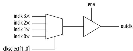
The enable signal is applied to the clock signal before being distributed to global routing. Therefore, the enable signal can either have a significant timing slack (at least as large as the global routing delay) or it can reduce the  $f_{MAX}$  of the clock signal.
