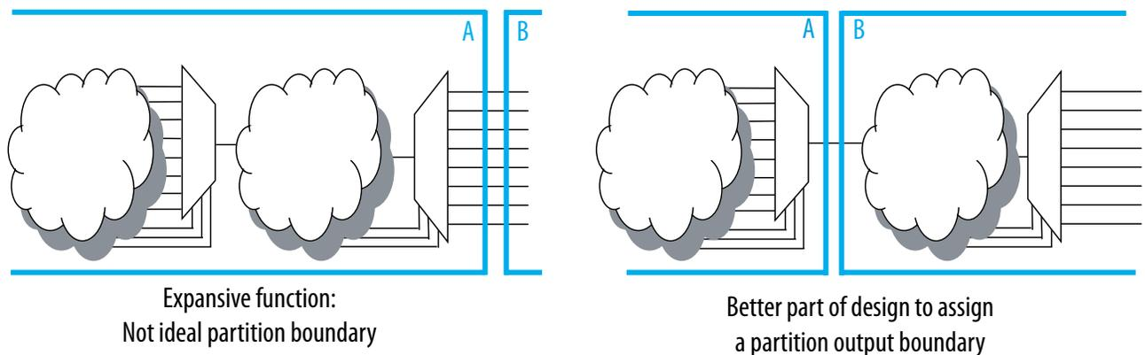
Another way to minimize connections between partitions is to avoid using combinational "glue logic" between partitions. You can often move the logic to the partition at one end of the connection to keep more logic paths within one partition. For example, the bottom diagram includes a new level of hierarchy C defined as a partition instead of block B. Clearly, there are fewer I/O connections between partitions A and C than between partitions A and B.
