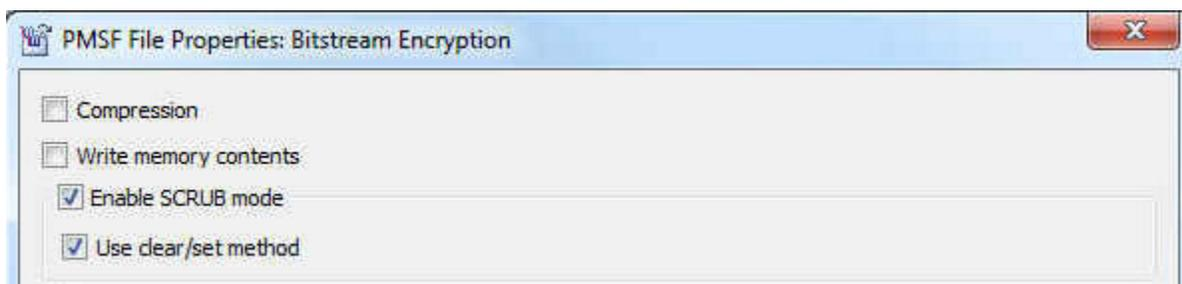
If there are more than one PR regions along a LAB column, and you are trying to reconfigure one of the PR regions, it is not possible to correctly determine the bits associated with the PR region that is not changing. For this reason, you can not use the SCRUB mode when you have two PR regions that have a vertically overlapping column in the device. This restriction does not apply to the static bits because they never change and you can rewrite them with the same value of the configuration bit.
