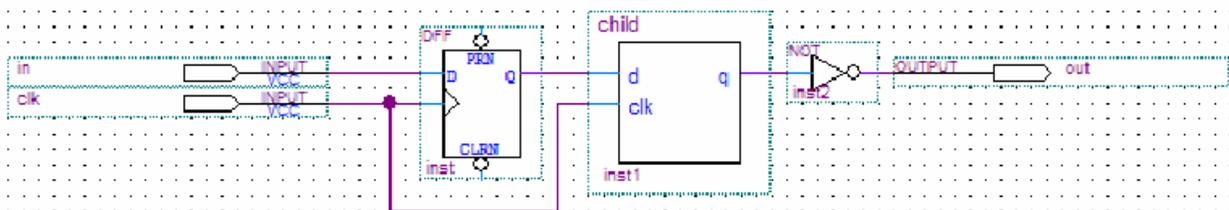
In these cases, the Quartus Prime software does not perform register packing. If there is a **Fast Input Register** assignment on pin `in`, as shown in the top figure, or a **Fast Output Register** assignment on pin `out`, as shown in the bottom figure, the Quartus Prime software issues a warning that the Fitter cannot pack the node to an I/O pin because the node and I/O cell are connected across a design partition boundary.
