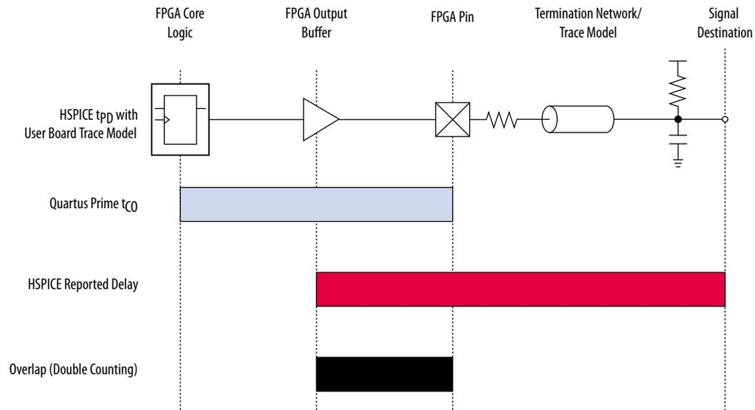
HSPICE models for board simulation measure  $t_{PD}$  (propagation delay) from an arbitrary reference point in the output buffer, through the device pin, out along the board routing, and ending at the signal destination.
