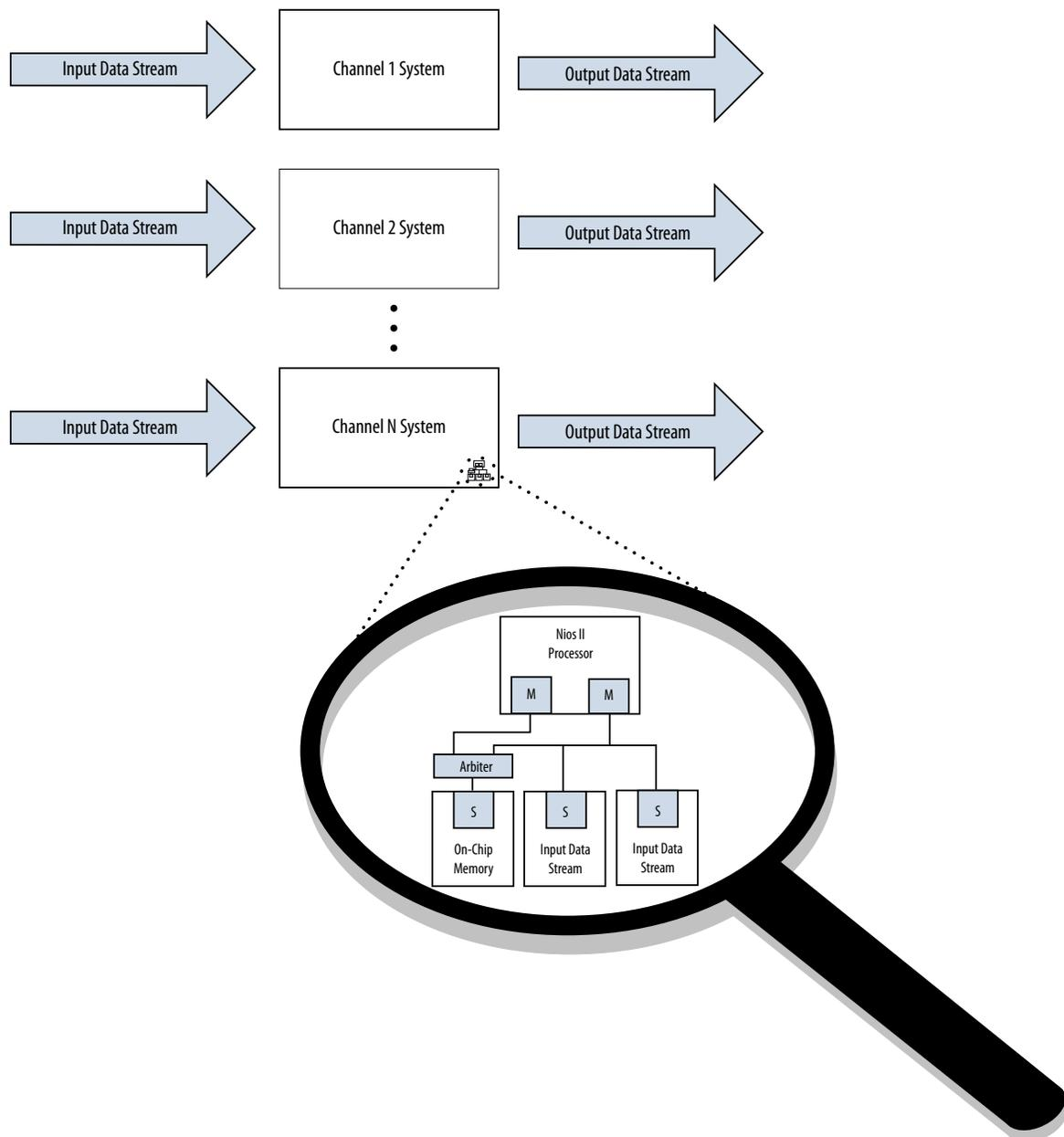
You can also design systems that process multiple data channels by instantiating the same subsystem for each channel. This approach is easier to maintain than a larger, non-hierarchical system. Additionally, such systems are easier to scale because you can calculate the required resources as a multiple of the subsystem requirements.
