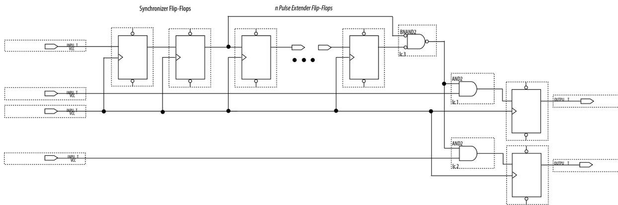
1. Junction dots indicate the number of stages. You can have more flip flops to get a wider pulse that spans more clock cycles.
