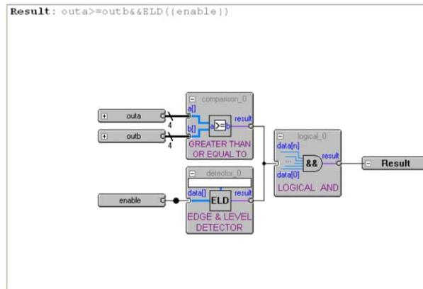
**Figure 13-25: Bitwise AND Operation**
