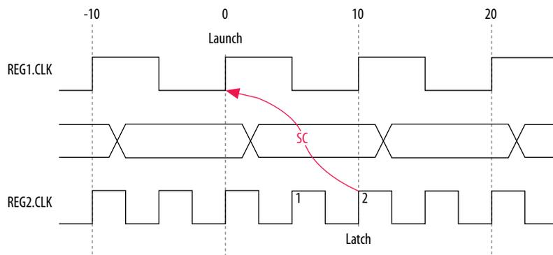
The timing diagram for default hold check analysis performed by the TimeQuest analyzer with an end multicycle setup value of two.
