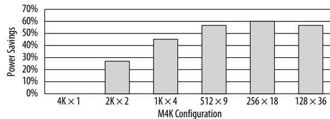
As the memory depth becomes more shallow, memory dynamic power decreases because unaddressed M4K blocks can be shut off using a decoded combination of address bits and the read enable signal. For a 128-deep memory block, power used by the extra LEs starts to outweigh the power gain achieved by using a more shallow memory block depth. The power consumption of the memory blocks and associated LEs depends on the memory configuration.
