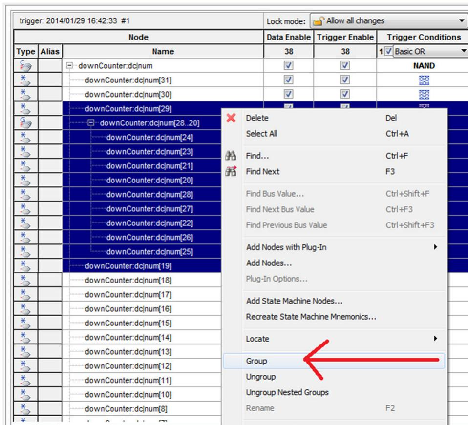
Figure 13-22: Applying Group Trigger Condition
