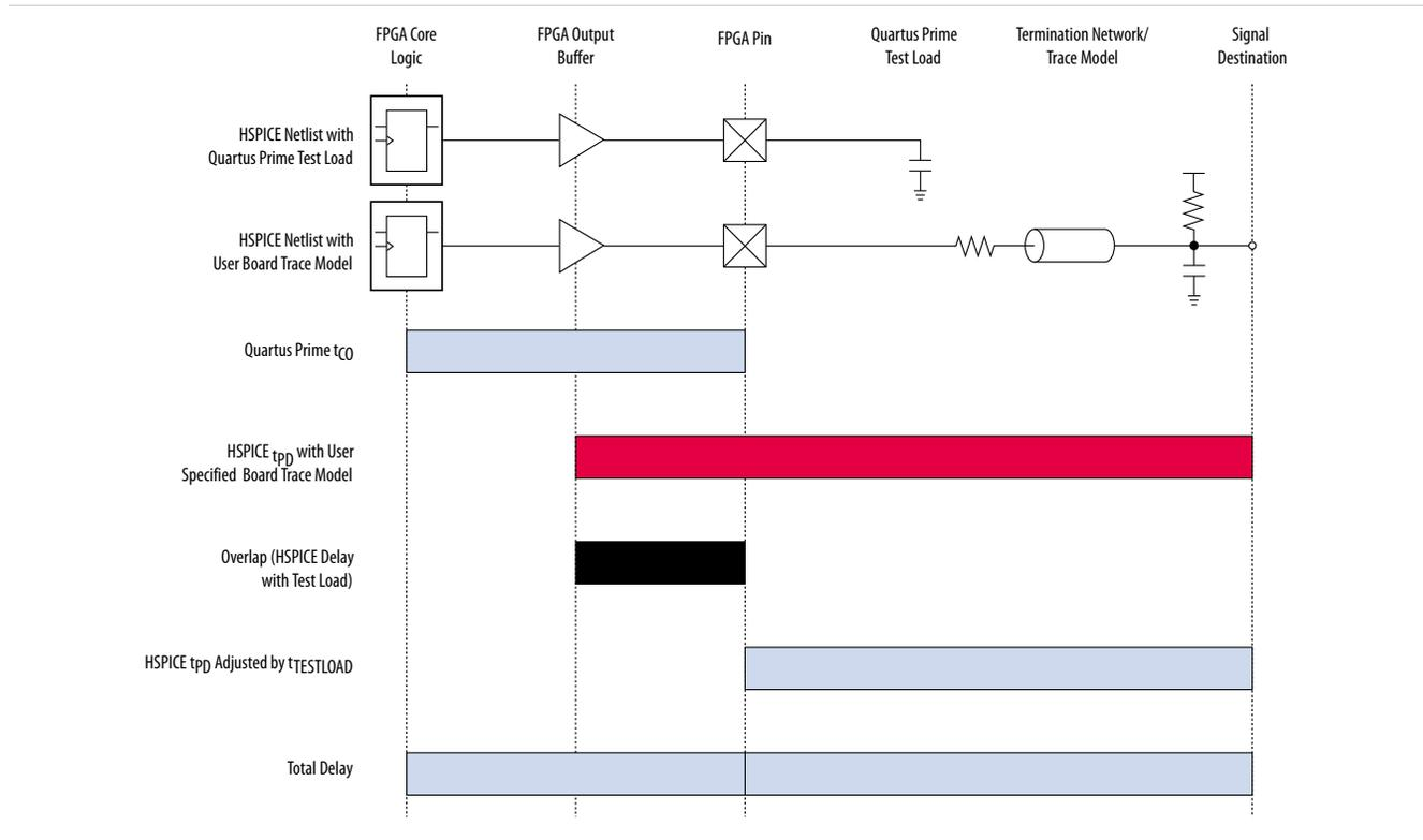
With  $t_{TESTLOAD}$  known, the total delay is calculated for the output signal from the FPGA logic to the signal destination on the board, accounting for the double count.
