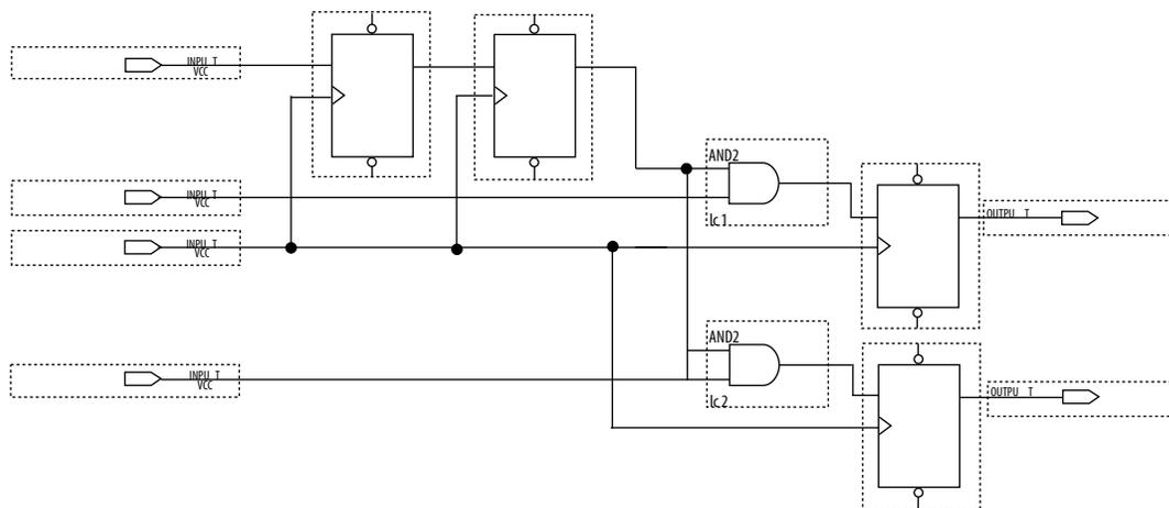
The following example shows the Verilog equivalent of the schematic. Only the clock edge is in the sensitivity list for a synchronous reset.
