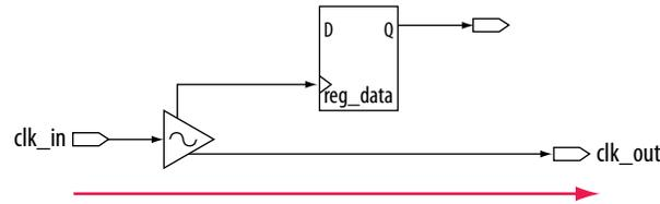
With clock-as-data analysis, the TimeQuest analyzer provides a more accurate analysis of the path based on user constraints. For the clock path analysis, any phase shift associated with the phase-locked loop (PLL) is taken into consideration. For the data path analysis, any phase shift associated with the PLL is taken into consideration rather than ignored.
