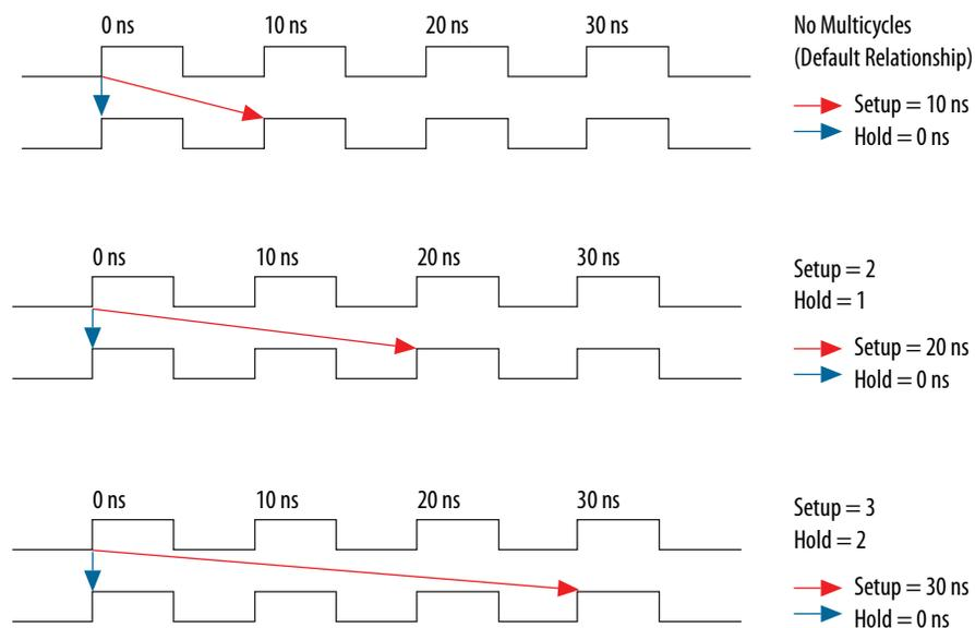
This pattern can be extended to create larger setup relationships in order to ease timing closure requirements. A common use for this exception is when writing to asynchronous RAM across an I/O interface. The delay between address, data, and a write enable may be several cycles. A multicycle exception to I/O ports can allow extra time for the address and data to resolve before the enable occurs.
