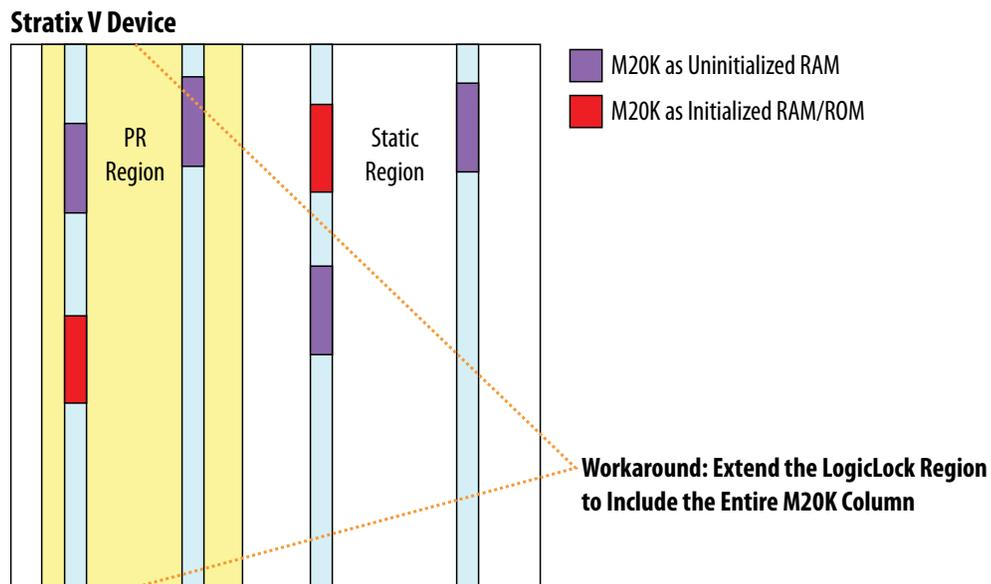
**Figure 4-23: Alternative Workaround for Using M20Ks in PR Region**
