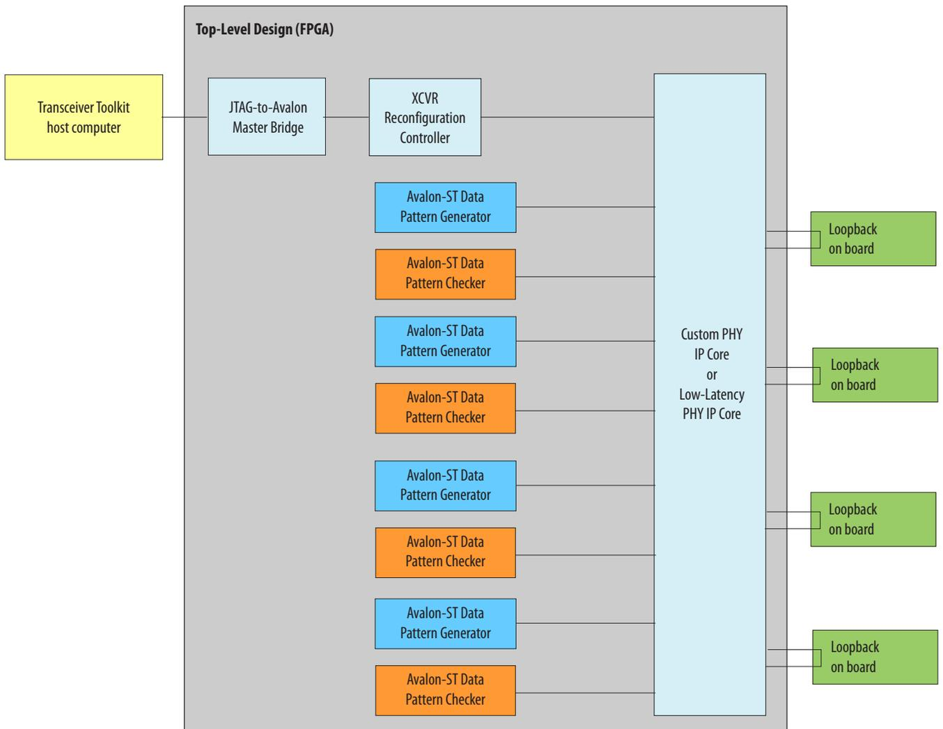
Figure 11-17: Four Channel Loopback Mode for Arria 10 / Generation 10 / 20nm
