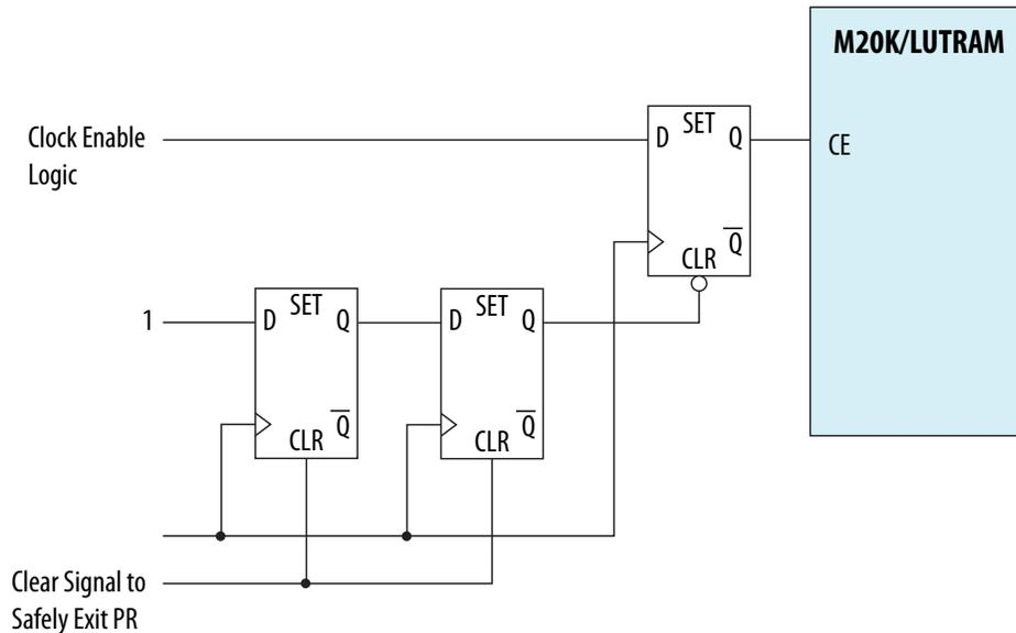
The circuit depends on an active-high clear signal from the static region. Before entering PR, freeze this signal in the same manner as all PR inputs. Your host control logic should de-assert the clear signal as the final step in the PR process.
