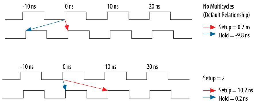
Adding the following constraint in your SDC allows the data to transfer to the following edge.
