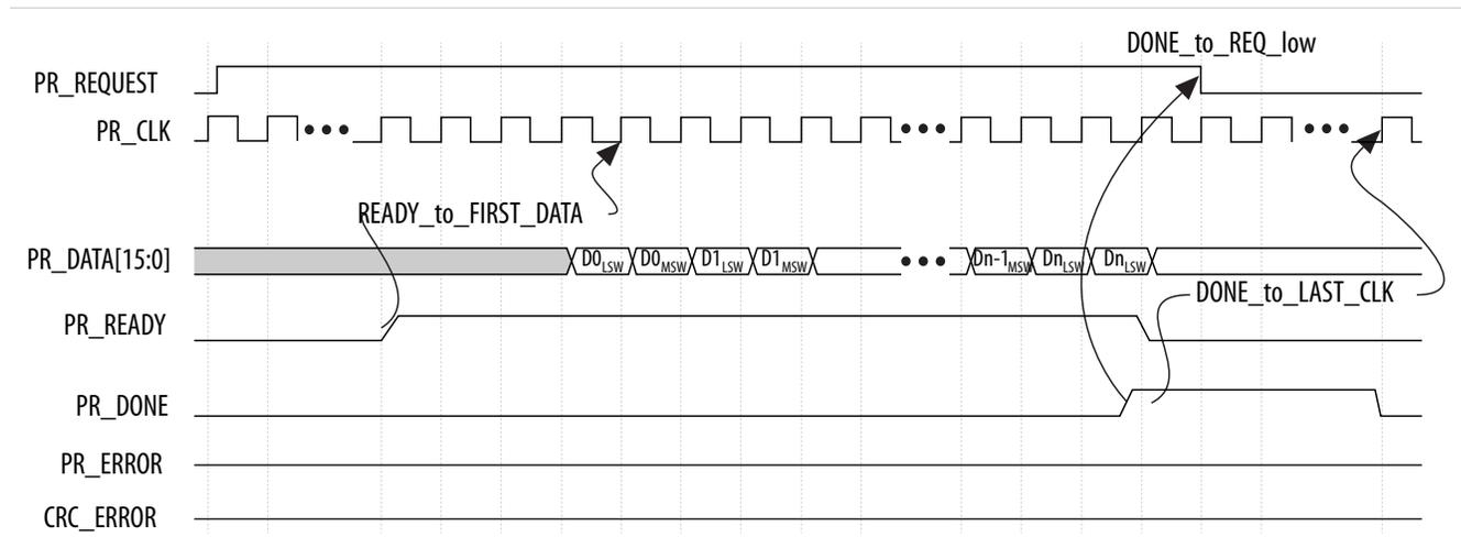
If there is an error encountered during partial reconfiguration, the FPGA device asserts the `PR_ERROR` signal high and de-asserts the `PR_READY` signal low.
