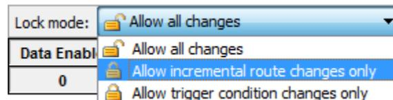
8. Add additional nodes in the SignalTap II **Setup** tab without exceeding the number of manually allocated nodes in step 2. Avoid making changes to non-runtime configurable settings.
