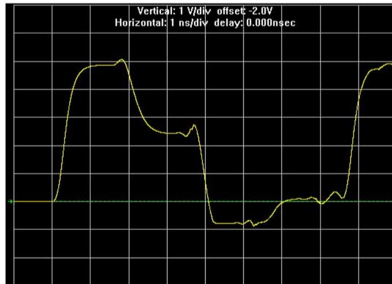
If you see a discontinuity or other anomalies at the destination, such as slow rise and fall times, adjust the termination scheme or termination component values. After making these changes, rerun the simulation to check whether your adjustments solved the problem. In this case, it is not necessary to regenerate the **.ibs** file.
