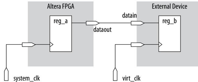
You can create a 10 ns virtual clock named `virt_clk` with a 50% duty cycle where the first rising edge occurs at 0 ns by adding the following code to your SDC file. The virtual clock is then used as the clock source for an output delay constraint.
