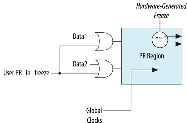
During partial reconfiguration, the static region logic should not depend on the outputs from PR regions to be at a specific logic level for the continued operation of the static region.
