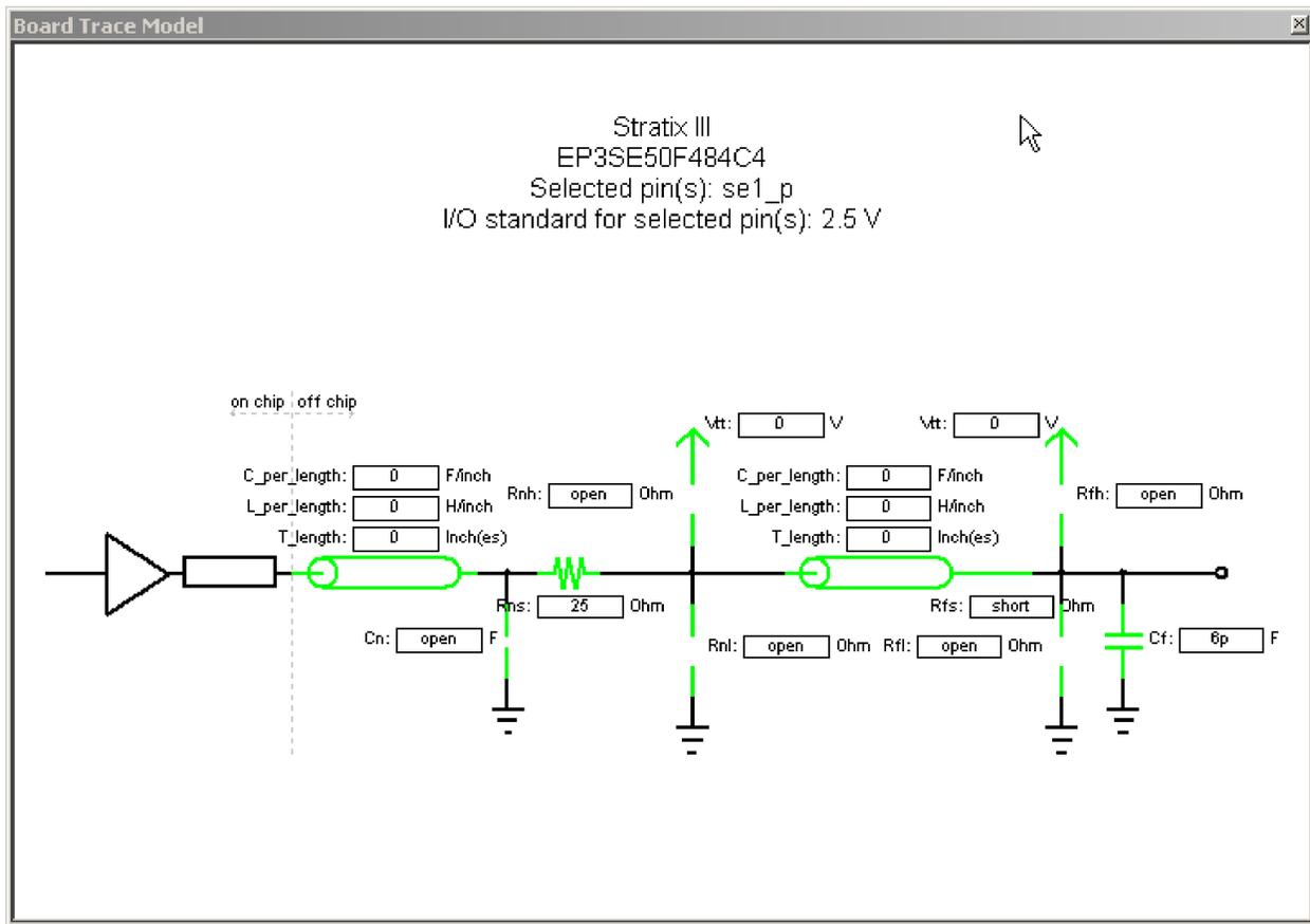
The following figure shows the template for the LVDS I/O standard. The far-end capacitance ( $C_f$ ) represents the external-device or multiple-device capacitive load. If you have multiple devices on the far-end, you must find the equivalent capacitance at the far-end, taking into account all receiver capacitances. The far-end capacitance can be the sum of all the receiver capacitances.
