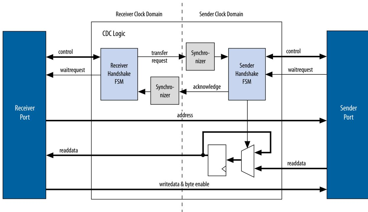
This example illustrates a clock domain adapter between one master and one slave. The synchronizer blocks use multiple stages of flip flops to eliminate the propagation of meta-stable events on the control signals that enter the handshake FSMs. The CDC logic works with any clock ratio.
