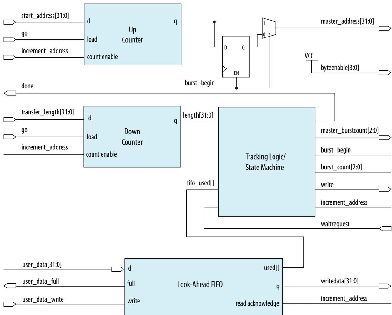
The master performs word accesses and writes to sequential memory locations. When `go` is asserted, the `start_address` and `transfer_length` are registered. On the next clock cycle, the control logic asserts `burst_begin`, which synchronizes the internal control signals in addition to the `master_address` and
