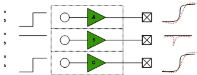
Voltage noise is measured as the change in voltage of a signal due to SSN. When a signal is QH, it is measured as the change in voltage toward 0 V. When a signal is QL, it is measured as the change in voltage toward  $V_{CC}$ .
