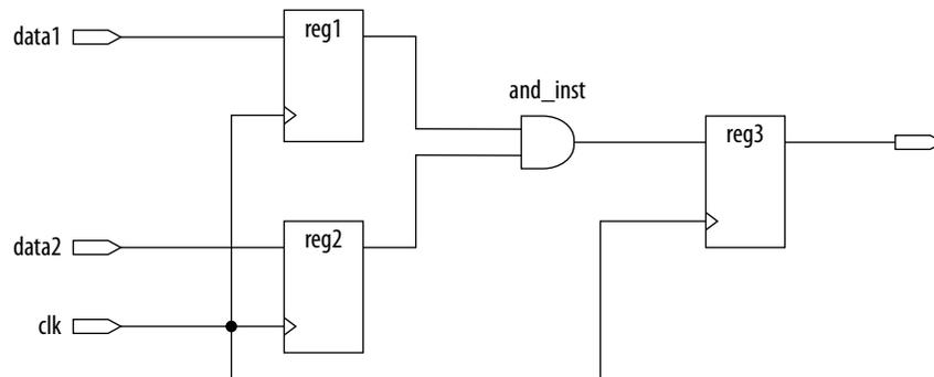
The timing netlist for the sample design shows how different design elements are divided into cells, pins, nets, and ports.
