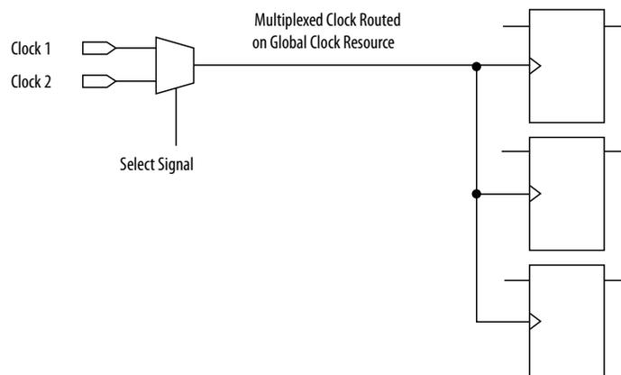
Adding multiplexing logic to the clock signal can create the problems addressed in the previous sections, but requirements for multiplexed clocks vary widely, depending on the application. Clock multiplexing is acceptable when the clock signal uses global clock routing resources and if the following criteria are met:
