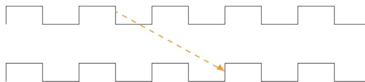
`set_multicycle_path -from <generating register> -setup -end 2`
