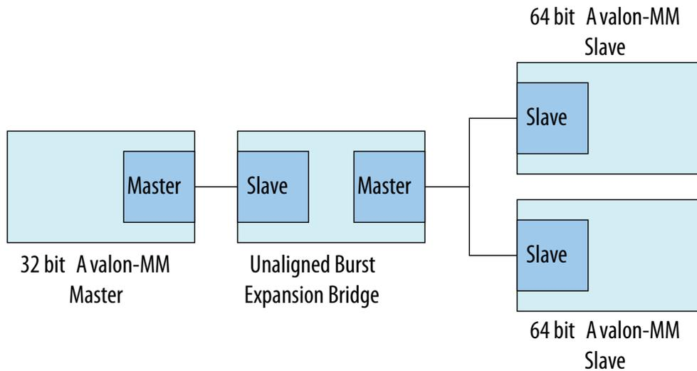
You can use the Avalon Unaligned Burst Expansion Bridge to align read burst transactions from masters that have narrower data widths than the target slaves. Using the bridge for this purpose improves bandwidth utilization for the master-slave pair, and ensures that unaligned bursts are processed as single transactions rather than multiple transactions.
