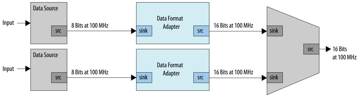
The diagram below illustrates a data path that uses the dual clock version of the on-chip FIFO memory and Avalon-ST channel multiplexer to merge the 100 MHz input from two streaming data sources into a single 200 MHz streaming output. This example shows an output with double the throughput of each interface with a corresponding doubling of the clock frequency.
