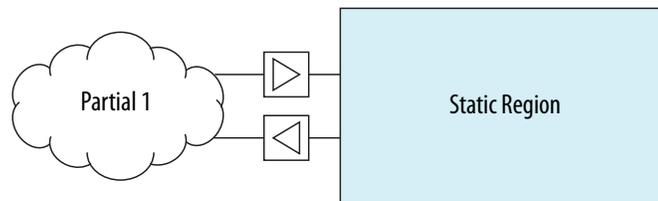
If one persona of your PR region has a different number of ports than others, then you must create a wrapper so that the static region always communicates with this wrapper. In this wrapper, you can create dummy ports to ensure that all of the PR personas of a PR region have the same connection to the static region.
