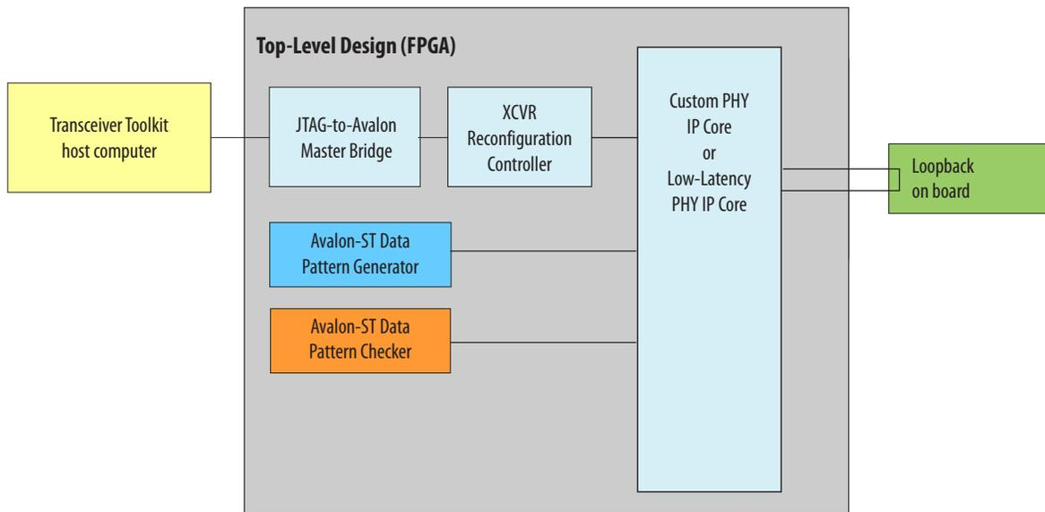
Figure 11-15: One Channel Loopback Mode for Arria 10 / 20nm
