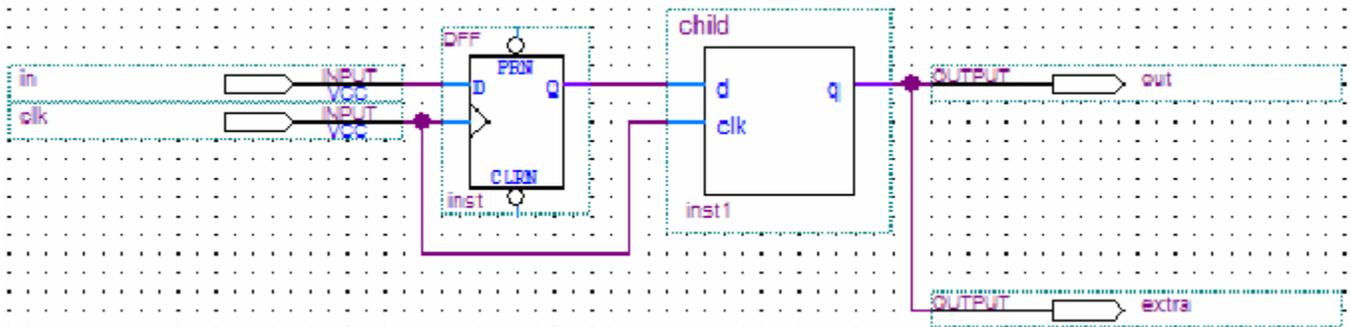
In this case, the Quartus Prime software does not perform output register packing. If there is a **Fast Output Register** assignment on pin `out`, the software issues a warning that the Fitter cannot pack the node to an I/O pin because the node and the I/O cell are connected across a design partition boundary.
