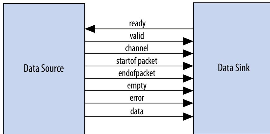
The IP Catalog includes a number of Avalon-ST components that you can use to create datapaths, including datapaths whose input and output streams have different properties. Generated systems that include memory-mapped master and slave components may also use these Avalon-ST components because Qsys generation creates interconnect with a structure similar to a network topology, as described in *Qsys Transformations*. The following sections introduce the Avalon-ST components.
