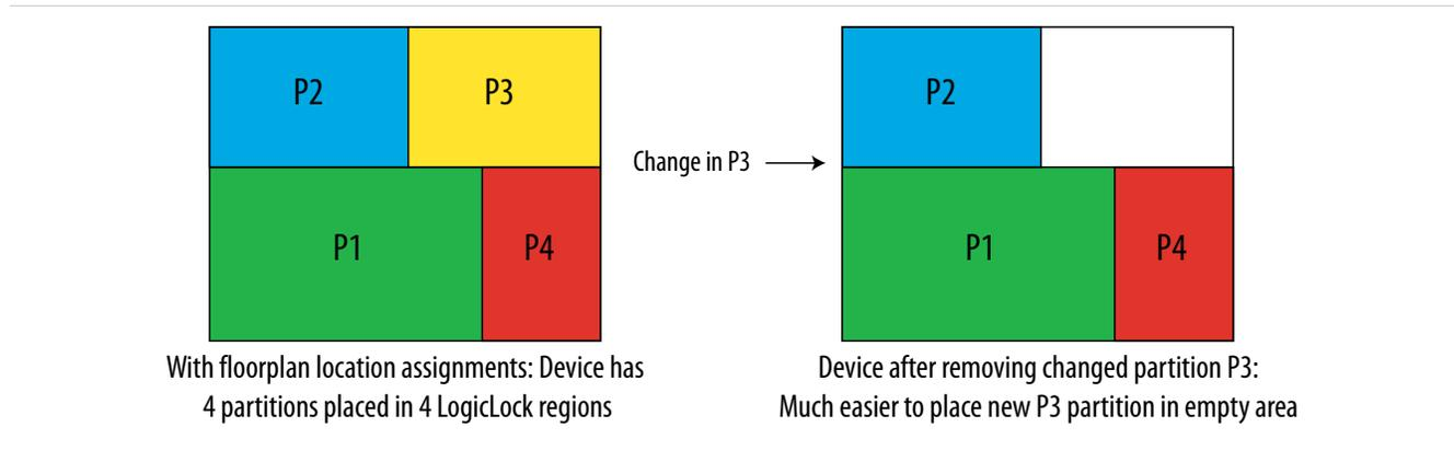
Altera recommends that you create a LogicLock floorplan assignment for timing-critical blocks with little timing margin that will be recompiled as you make changes to the design.
