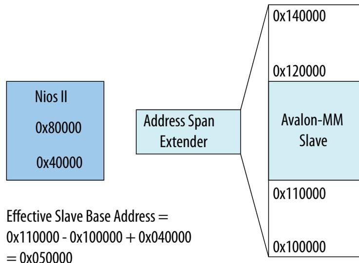
If the address span extender window is dynamic. For example, when the **Disable Slave Control Port** option is turned off, the NIOS II processor is unable to see components on the slave side of the address span extender.
