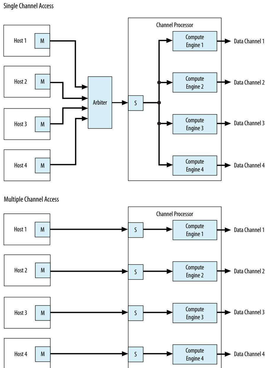
In this example, there are two channel processing systems. In the first, four hosts must arbitrate for the single slave interface of the channel processor. In the second, each host drives a dedicated slave interface, allowing all master interfaces to simultaneously access the slave interfaces of the component. Arbitration is not necessary when there is a single host and slave interface.
