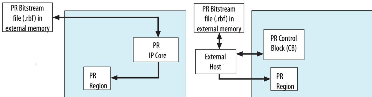
The PR mode is independent of the full chip programming mode. You can use any of the supported full chip configuration modes for configuring the full FPGA for your PR design.
