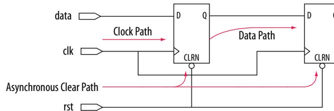
In addition to identifying various paths in a design, the TimeQuest analyzer analyzes clock characteristics to compute the worst-case requirement between any two registers in a single register-to-register path. You must constrain all clocks in your design before analyzing clock characteristics.
