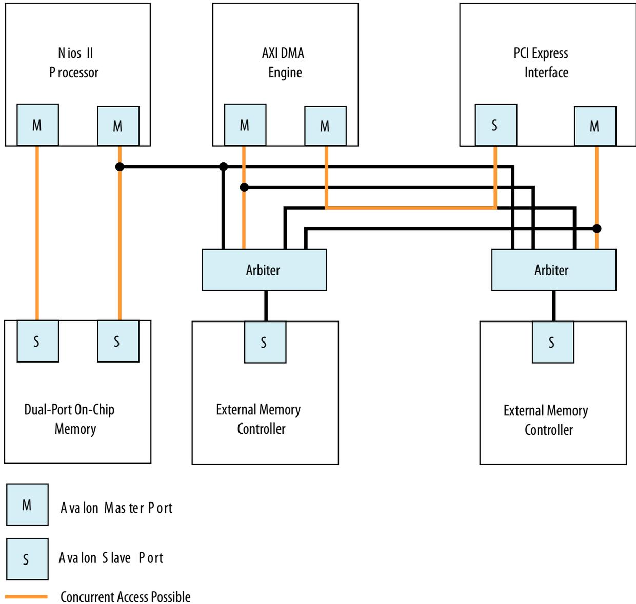
**Figure 8-5: AXI Multiple Master Parallel Access**
