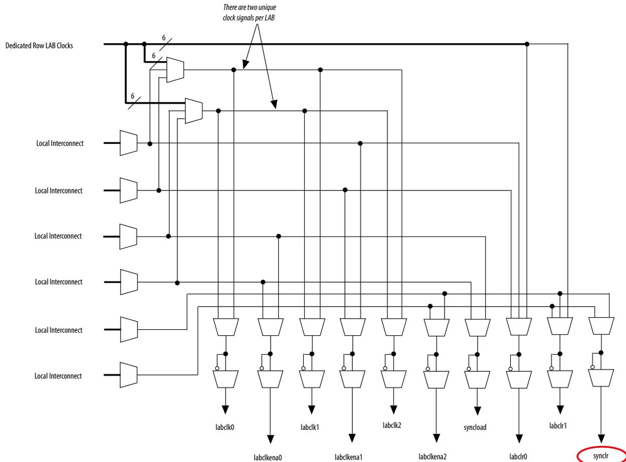
Consider two types of synchronous resets when you examine the timing analysis of synchronous resets—externally synchronized resets and internally synchronized resets. Externally synchronized resets are synchronized to the clock domain outside the FPGA, and are not very common. A power-on asynchronous reset is dual-rank synchronized externally to the system clock and then brought into the FPGA. Inside the FPGA, gate this reset with the data input to the registers to implement a synchronous reset.
