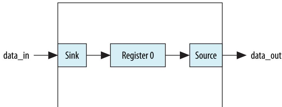
**Figure 10-30: Pipeline Stage Holding Register**
