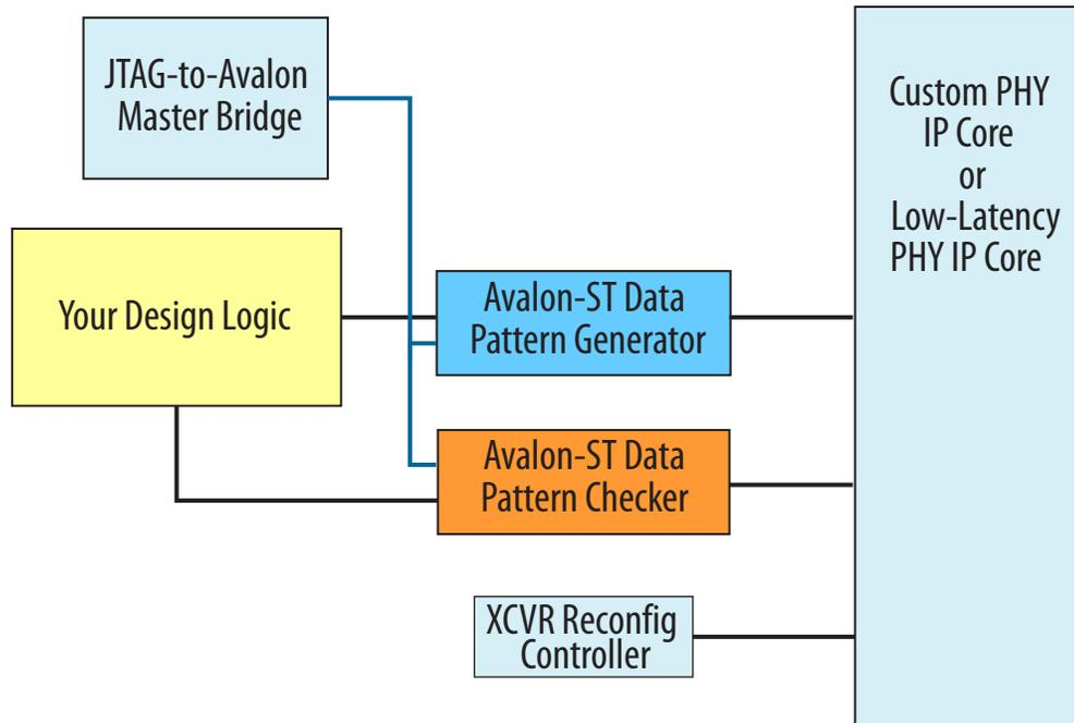
**Table 11-7: System Connections: Bit Error Rate Tests**
