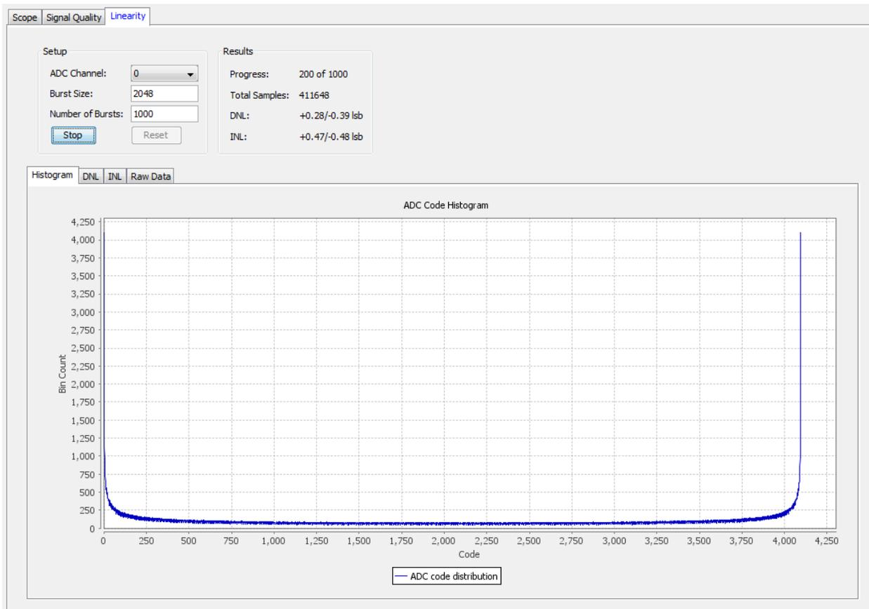
If your reference signal is not a relatively smooth line, but has jagged edges with some bins having a value of 0, and adjacent bins with a much higher value, then the test signal frequency is not adequate. Use **Scope** mode to help choose a good frequency for linearity testing.
