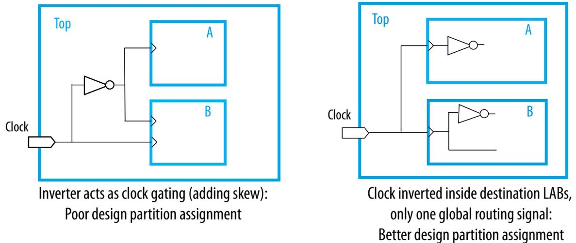
Notice that this diagram also shows another example of a single pin feeding two ports of a partition boundary. In the left diagram, partition B does not have the information that the clock and inverted clock come from the same source. In the right diagram, partition B has more information to help optimize the design because the clock is connected as one port of the partition.
