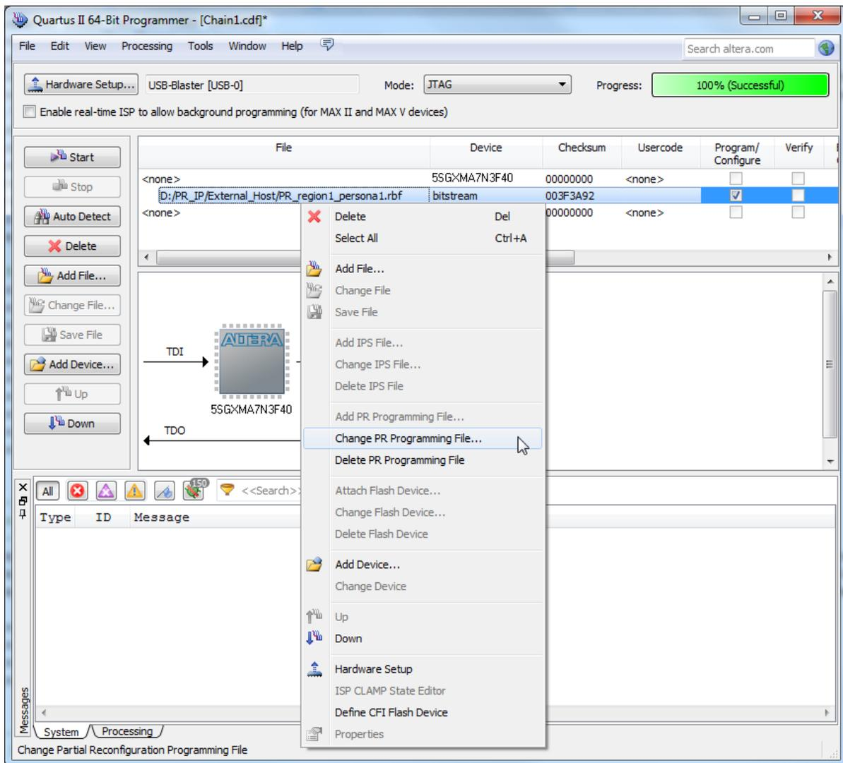
3. Click **Start** to configure the PR bitstream. The Quartus Prime Programmer generates an error message if the specified device does not contain the PR IP core in the design (you must instantiate the Partial Reconfiguration IP core in your design to use the JTAG debug mode).
