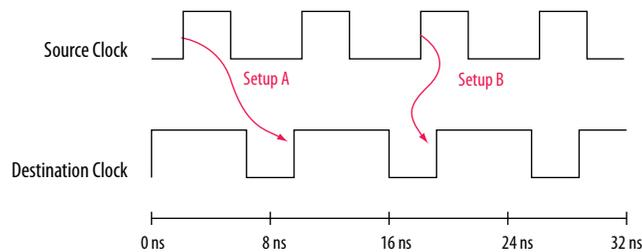
The TimeQuest analyzer reports the result of clock setup checks as slack values. Slack is the margin by which a timing requirement is met or not met. Positive slack indicates the margin by which a requirement is met; negative slack indicates the margin by which a requirement is not met.
