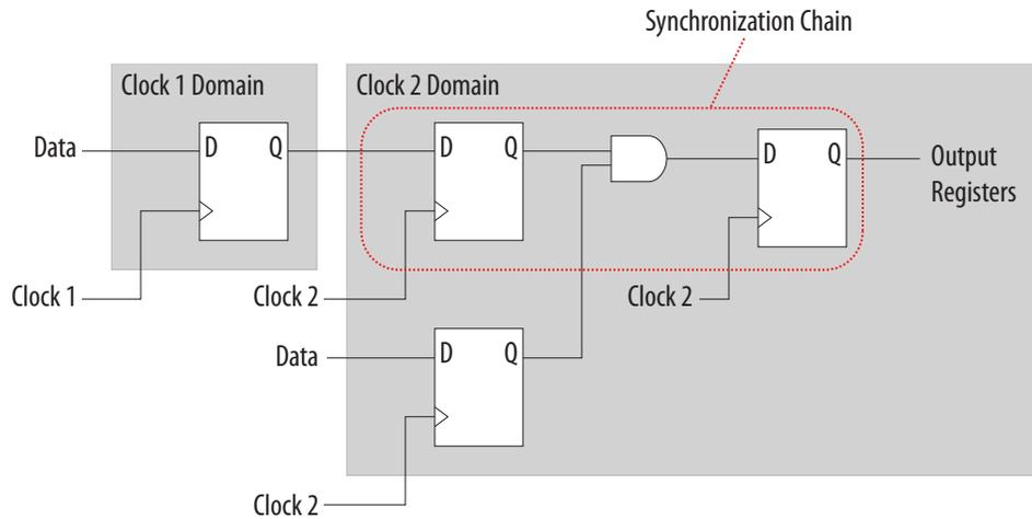
The timing slack available in the register-to-register paths of the synchronizer allows a metastable signal to settle, and is referred to as the available settling time. The available settling time in the MTBF calculation for a synchronizer is the sum of the output timing slacks for each register in the chain. Adding available settling time with additional synchronization registers improves the metastability MTBF.
