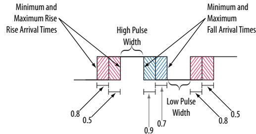
With common clock path pessimism, the minimum pulse width slack can be increased by the smallest value of either the maximum rise time minus the minimum rise time, or the maximum fall time minus the minimum fall time. In the example, the slack value can be increased by 0.2 ns, which is the smallest value between 0.3 ns (0.8 ns – 0.5 ns) and 0.2 ns (0.9 ns – 0.7 ns).
