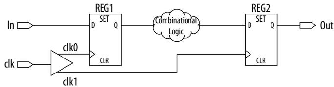
Timing diagram for default setup check analysis the TimeQuest analyzer performs.
