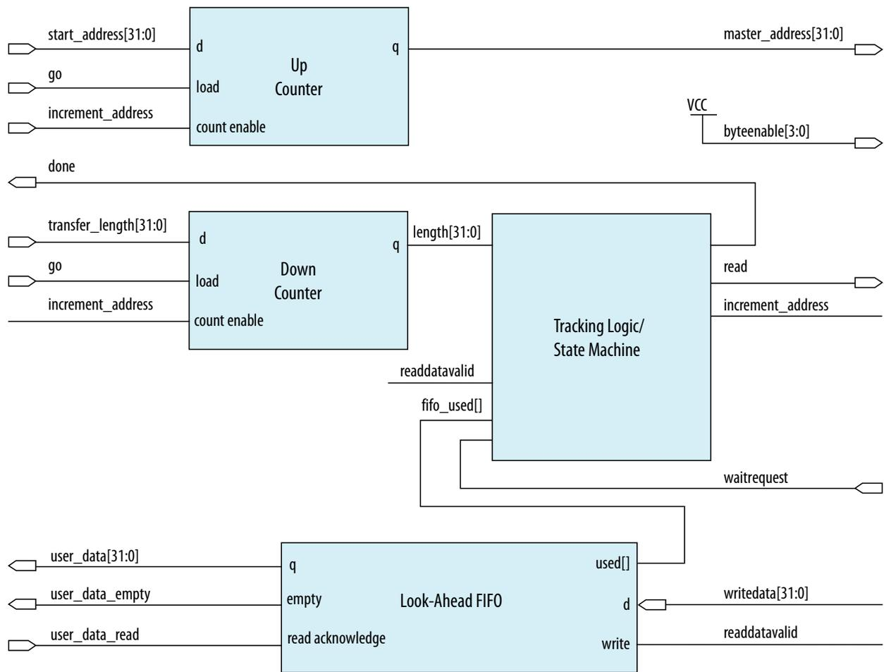
This example shows a pipelined read master that stores data in a FIFO. The master performs word accesses that are word-aligned and reads from sequential memory addresses. The transfer length is a multiple of the word size.
