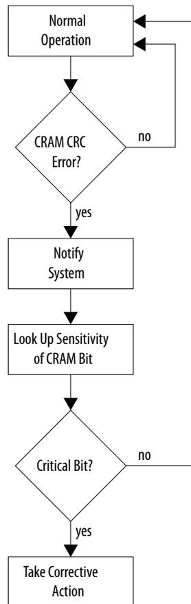
The ratio of SEU strikes versus functional interrupts is the Single Event Functional Interrupt (SEFI) ratio. Minimizing this ratio improves SEU mitigation.
