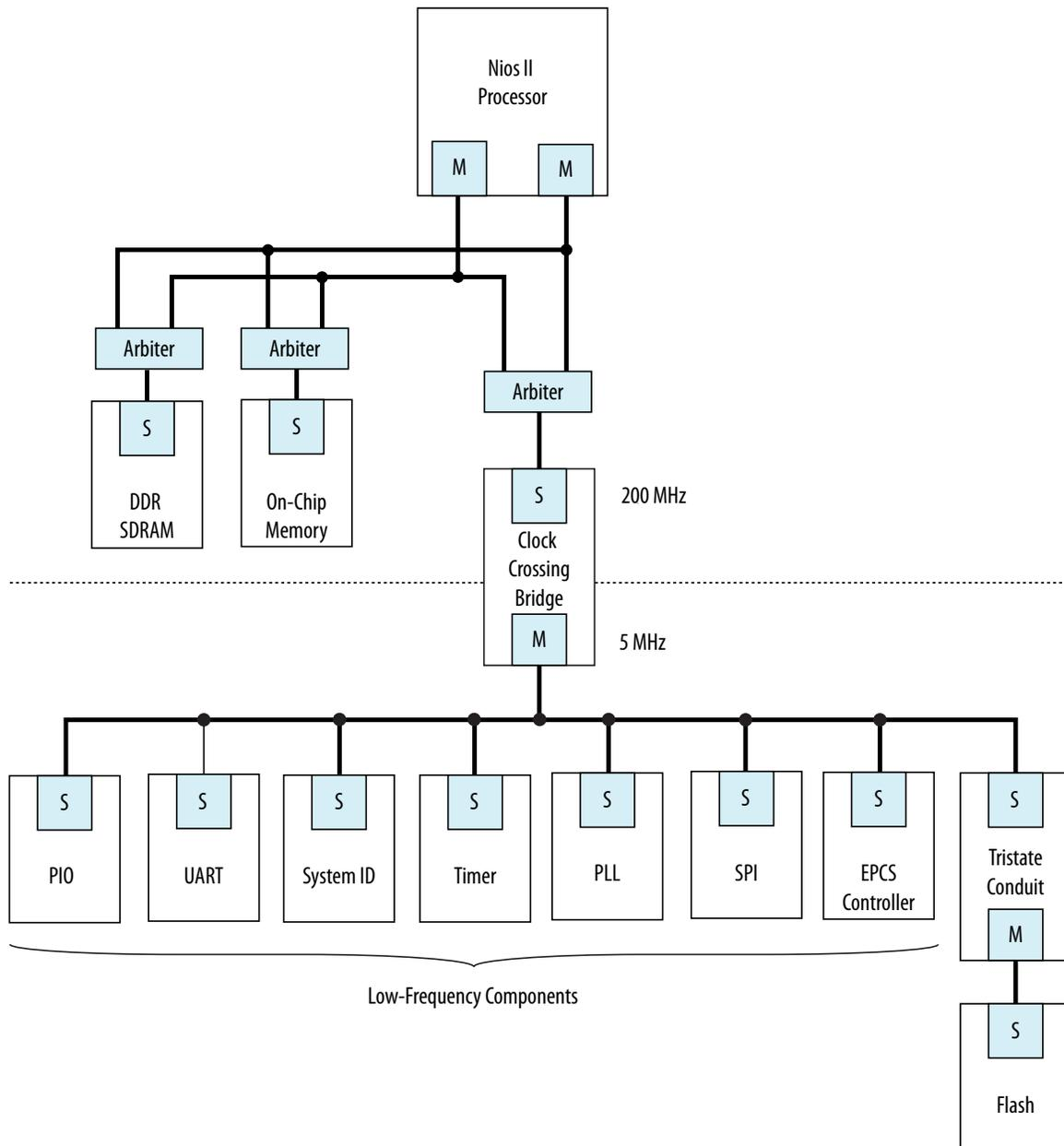
Qsys automatically inserts clock crossing adapters between master and slave interfaces that operate at different clock frequencies. You can choose the type of clock crossing adapter in the Qsys **Project Settings**
