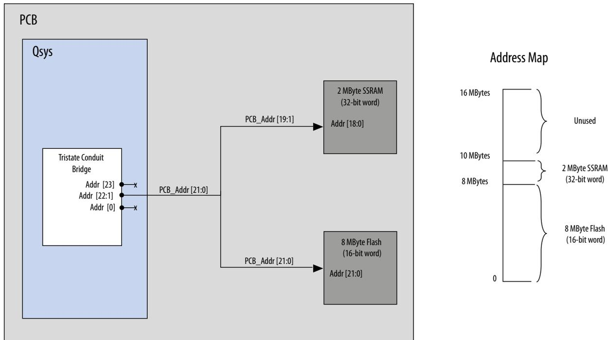
**Note:** If you create a custom tri-state conduit master with word aligned addresses, the Tri-state Conduit Pin Sharer does not change or align the address signals.
