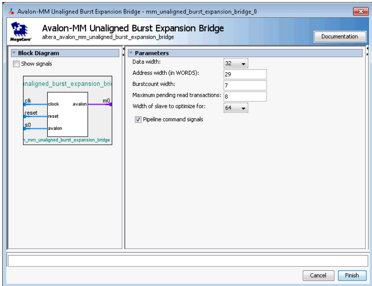
Table 10-2: Avalon-MM Unaligned Burst Expansion Bridge Parameters
