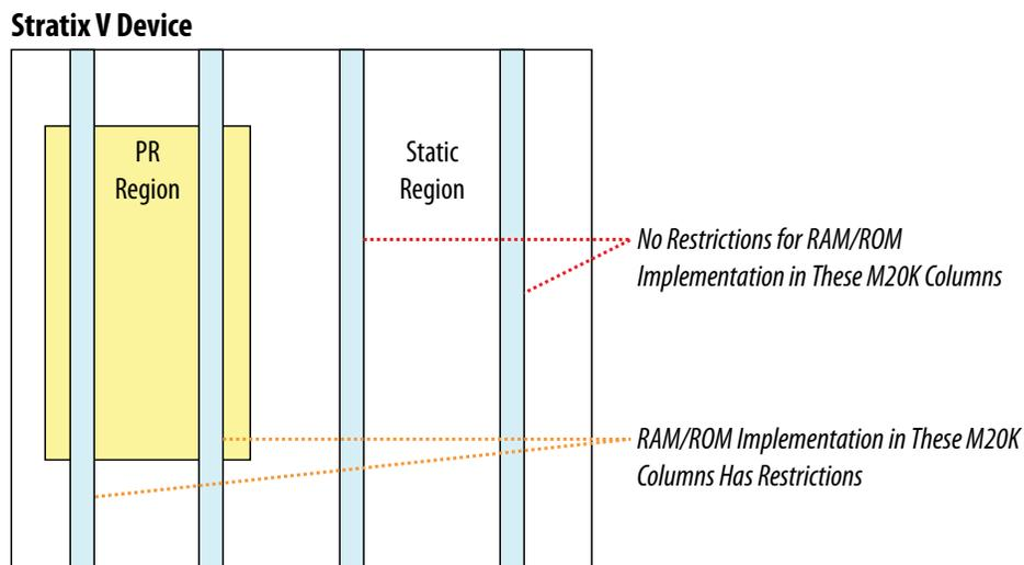
If the functionality of the static region depends on any data read out from M20K RAMs in the static region, the design will malfunction.
