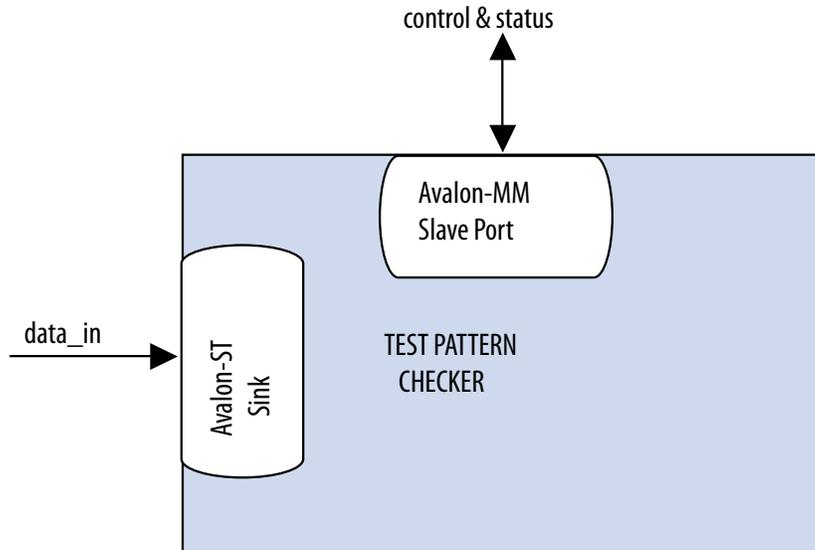
The test pattern checker detects exceptions and reports them to the control interface via a 32-element deep internal FIFO. Possible exceptions are data error, missing start-of-packet (SOP), missing end-of-packet (EOP), and signaled error.
