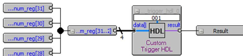
5. Right-click your Custom Trigger HDL object and configure the object's properties, see [Table 13-4](#).
