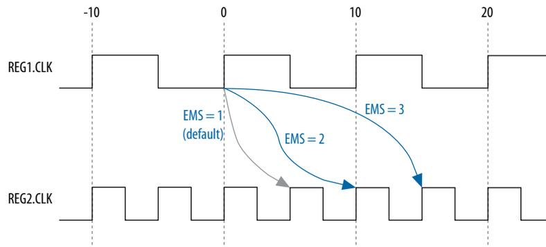
A start multicycle setup assignment modifies the launch edge of the source clock by moving the launch edge the specified number of clock periods to the left of the determined default launch edge. A start multicycle setup (SMS) assignment with various values can result in a specific launch edge.
