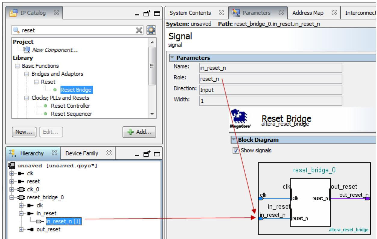
Each Qsys component has its own requirements for reset synchronization. Some blocks have internal synchronization and have no requirements, whereas other blocks require an externally synchronized reset. You can define how resets are synchronized in your Qsys system with the **Synchronous edges** parameter. In the clock source or reset bridge component, set the value of the **Synchronous edges** parameter to one of the following, depending on how the reset is externally synchronized:
