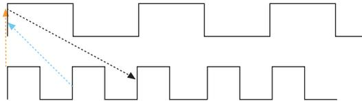
However, the default hold requirement, shown with the dashed blue line, may cause the router to add wire to guarantee that data is delayed by one cycle. To correct the hold requirement, add a multicycle constraint with a hold option.
