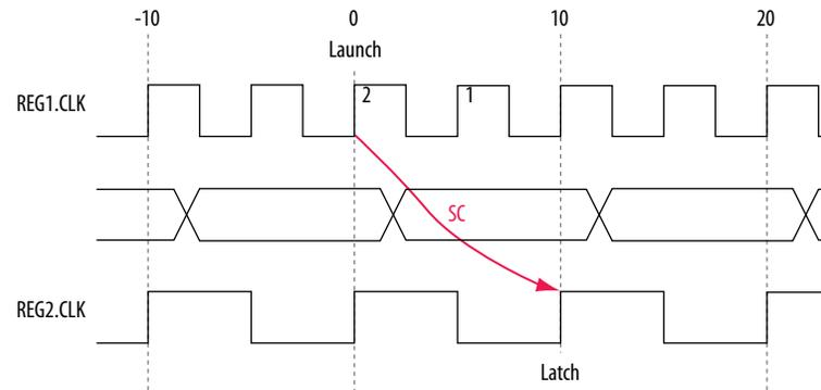
The timing diagram for default hold check analysis the TimeQuest analyzer performs for a start multicycle setup value of two.
