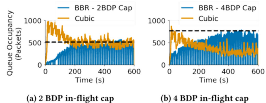
Figure 5: BBR vs Cubic in a 10Mbps×40ms testbed with a 32 BDP queue. Black dashed line is the model (5).
