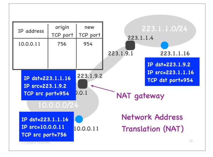
When the border router receives a packet coming from the private subnet, it first creates a piece of state, mapping IP address 10.0.0.11 and port number 756 to a new port number 954. Then it rewrites, not only the source IP address to 223.1.9.2; but also the source port number to 954.
