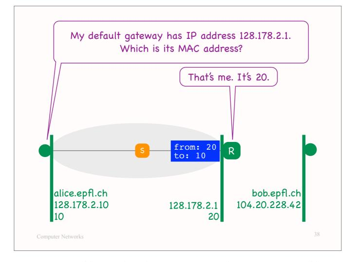
When R receives the ARP request, it recognizes its IP address and sends an ARP response that states its MAC address.
