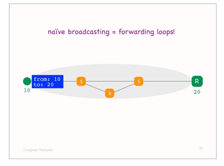
We said that, when a switch receives a packet with unknown destination MAC address, the switch broadcasts the packet. If all switches broadcast packets with unknown destination MAC addresses to all links (except the one where the packet arrived), there may be forwarding loops.
