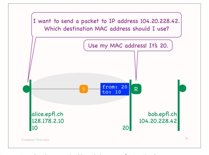
When R receives the ARP request, it recognizes that the target IP address belongs to a foreign IP subnet, meaning that any packet addressed to that IP address will have to exit the local IP subnet through R. Hence, R sends an ARP response that states its own MAC address.
