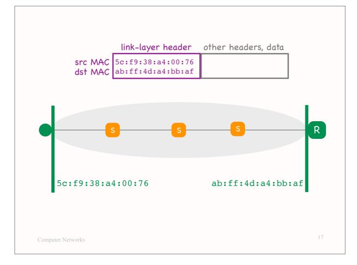
What if an end-system sends a packet to another end-system that is located in a different IP subnet? In that case, the packet will necessarily cross a router located at the border of the source end-system's IP subnet (to exit the subnet). While the packet is traveling inside the source end-system's IP subnet, its source MAC address is the MAC address of the source end-system, while the destination MAC address is the MAC address of this router.
