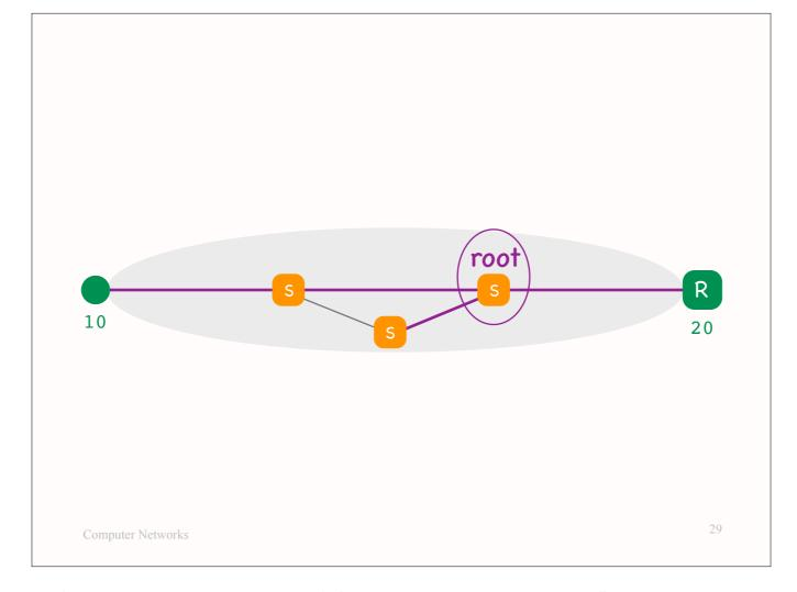
To avoid this, all the switches in an IP subnet participate in a protocol that creates a "spanning tree."
