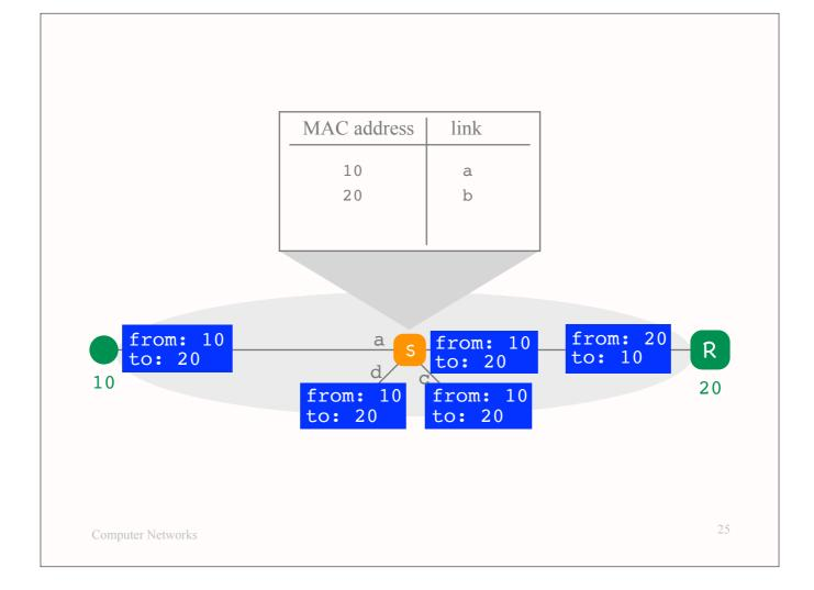
The forwarding table of a link-layer switch is initially empty. The switch fills the table based on the traffic it receives.
