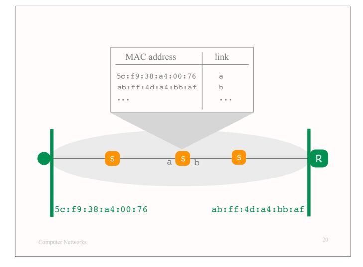
Each switch names its network interfaces (also called links, or ports), and keeps a forwarding table that maps MAC addresses to links.
