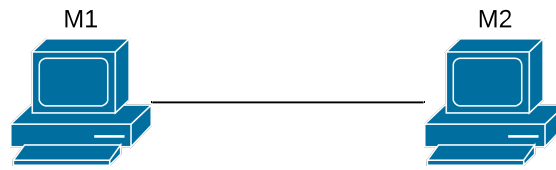
Figure 5: Point-to-point wired connection of two physical machines
