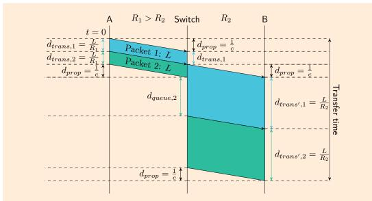
Figure 13: Timing diagram for a transmission over two links connected by a storeand-forward switch.
