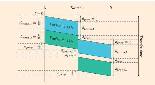
Figure 7: Timing diagram for a transmission over two links connected by a store-and-forward switch.
