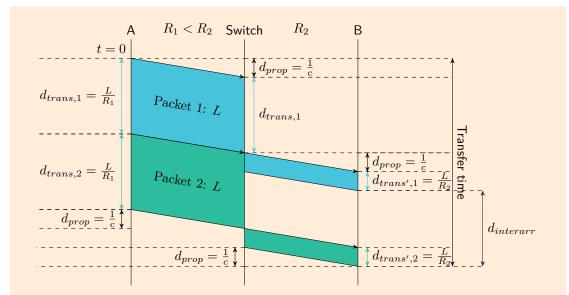
Figure 12: Timing diagram for a transmission over two links connected by a storeand-forward switch.
