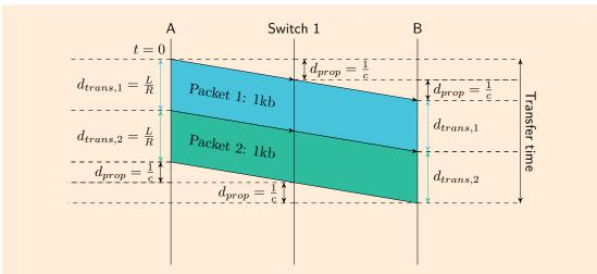
Figure 4: Timing diagram for a transmission over two links connected by a packet switch performing circuit switching.
