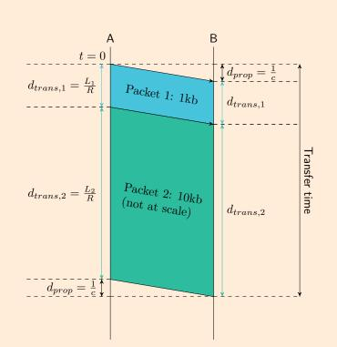
Figure 2: Timing diagram for transmitting two packets in sequence over a single link.
