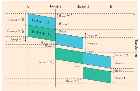
Figure 8: Timing diagram for a transmission over three links connected by store-and-forward switches.
