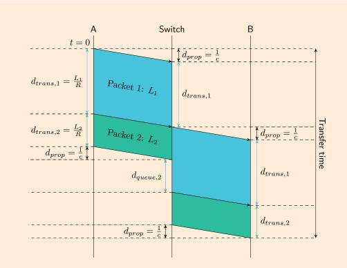
Figure 11: Timing diagram for a transmission over two links connected by a storeand-forward switch.
